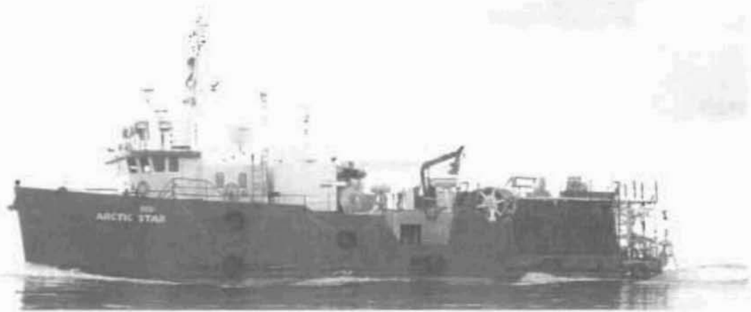
FIGURE 2.3. WesternGeco's larger source vessel, the R/V Arctic Star . This steel-hulled vessel was used to operate the 1210 in 3 airgun array (1999 photograph by W. Burgess, Greeneridge Sciences).
