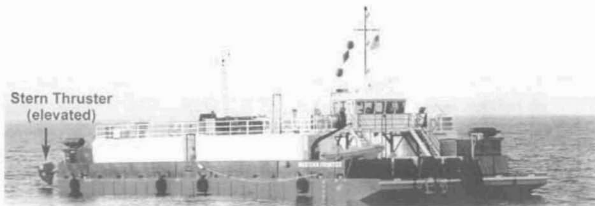
FIGURE 2.6. One of WesternGeco's cable vessels, the R/V Western Frontier , seen from the R/V Arctic Star (2000 photograph by J. Lawson, LGL). One of its three thrusters can be seen in an elevated configuration at the stern of the vessel.
