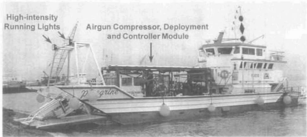
FIGURE 2.1. The primary source vessel R/V Peregrine as it appeared in 2001 after an "airgun compressor, deployment and controller module", painted blue, was installed on the foredeck (photograph by J. Lawson, LGL).
