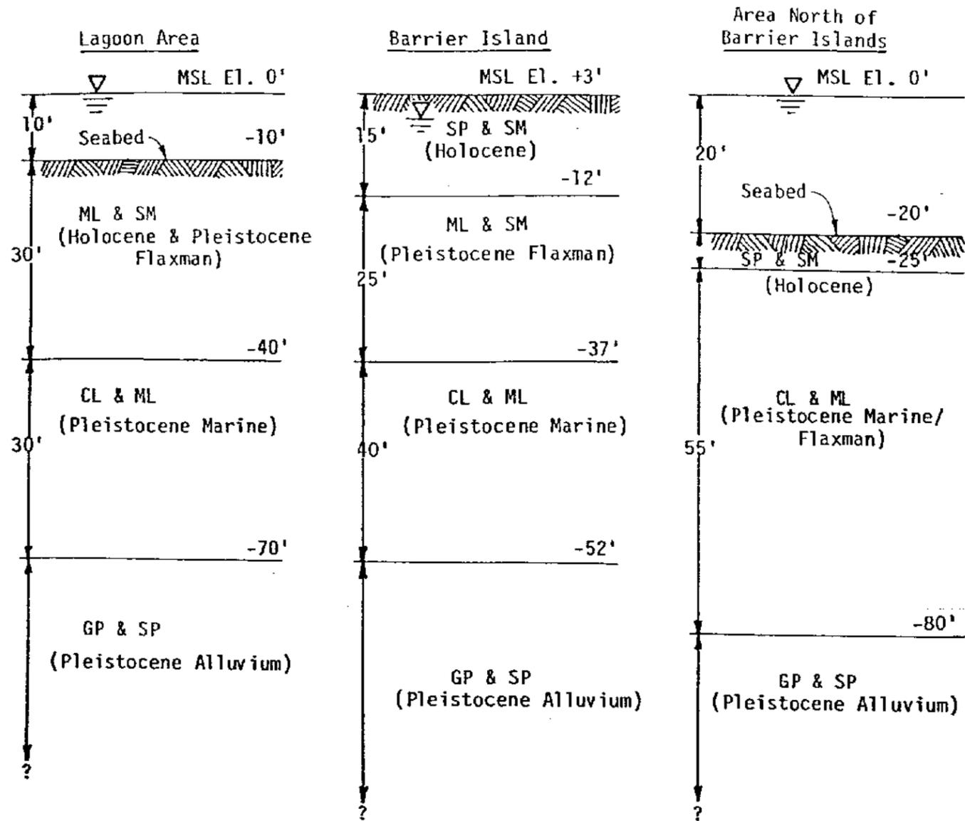
TYPICAL SOIL PROFILES AND LAYER THICKNESSES
