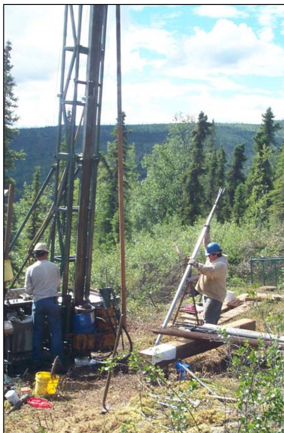
Front cover and above: Core drilling at the Hook target on AngloGold's Gobi gold property near the Pogo property in the Goodpaster mining district. Photos by David Szumigala.
