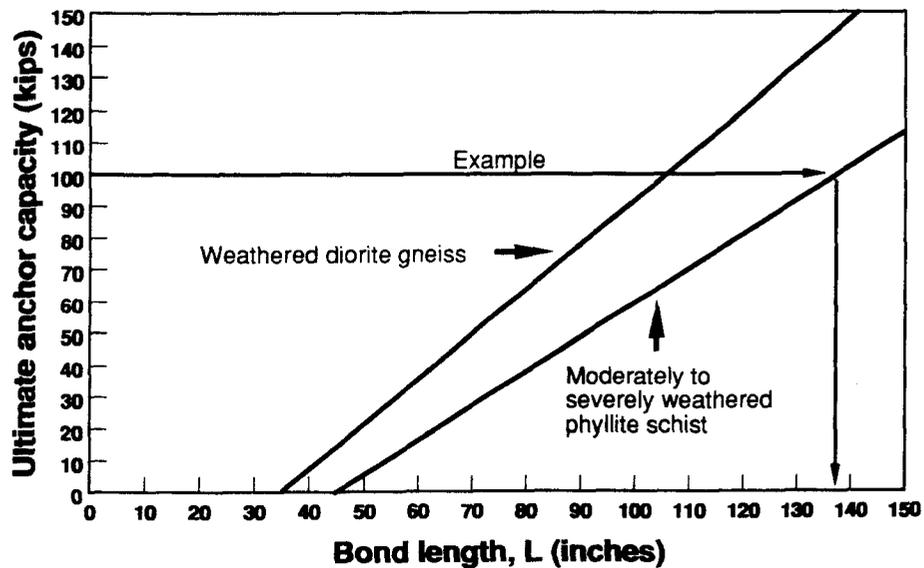
Figure 3—Ultimate anchor capacity as a function of grouted bond length in rock. This figure is based on results of anchor tests in rocks commonly found on Wrangell Island, southeast Alaska, and should be used with care at other localities where extensive weathering, fracturing, and discontinuous rock units are encountered.
