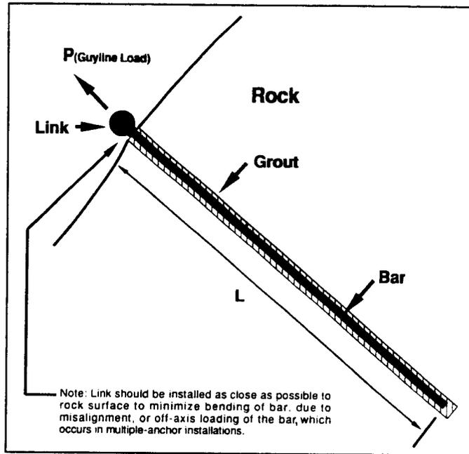
Figure 1—Elements of a grouted rock anchor.  $P$  is total guylines force or "load." A "link" is the mechanical connection between the guylines and the anchor. (One kip equals 1,000 pounds.)
