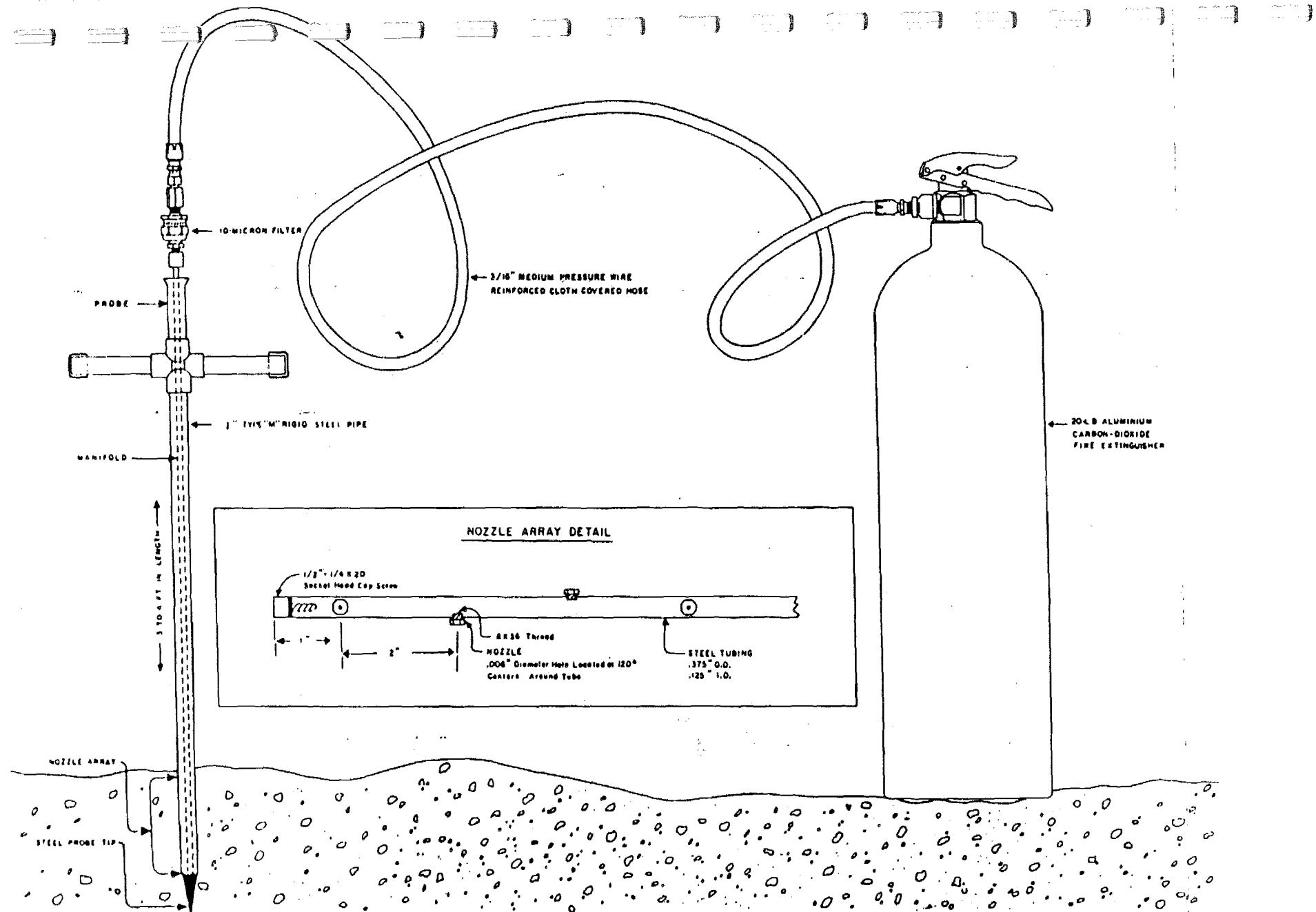
Figure 1. Single probe freeze core sampling system used for sampling substrate and eggs.
