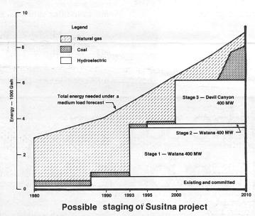
This diagram shows how the Susitna development would be staged under the medium forecast of future energy requirements. With this energy demand and ensuring that adequate generating reserves are maintained, power costs would be minimized if:
