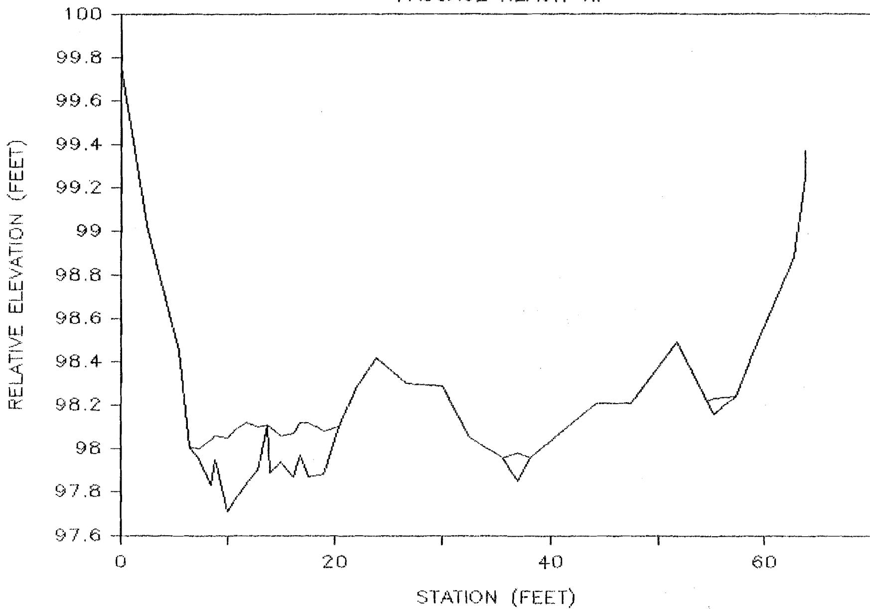
Appendix Figure D-28. Cross sectional profile of Passage Reach VII in Slough 9A, September 23, 1984.
