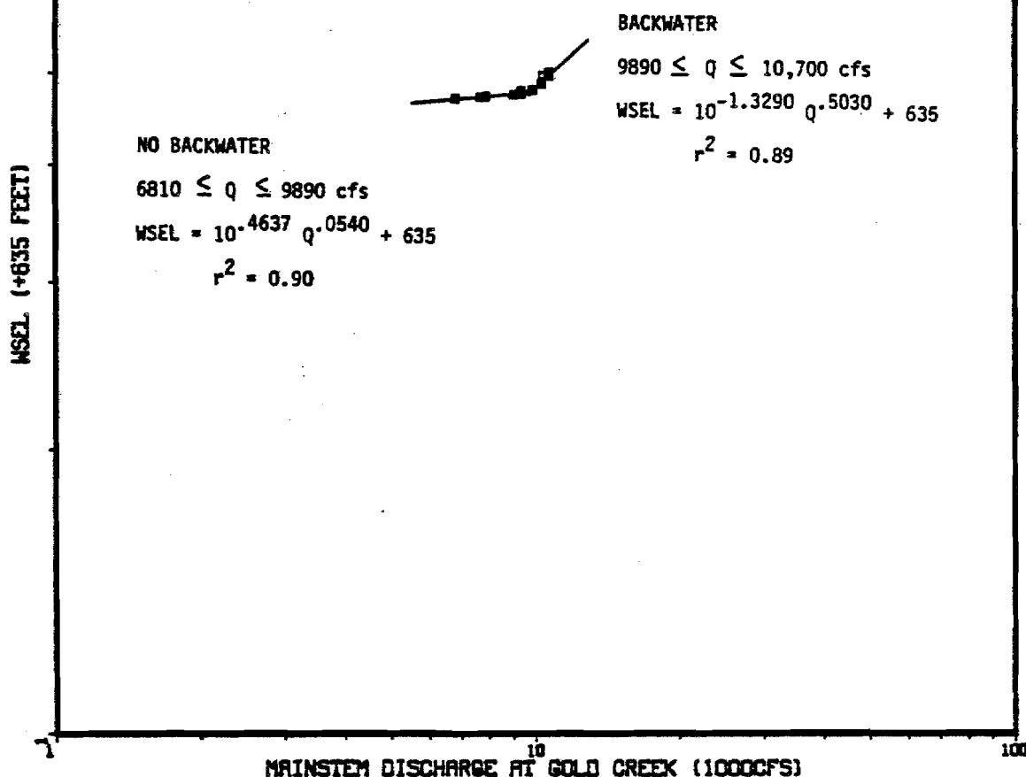
Appendix Figure E-4. Mainstem discharge (Provisional USGS 1984) versus the water surface elevation at Slough 9A mouth.
