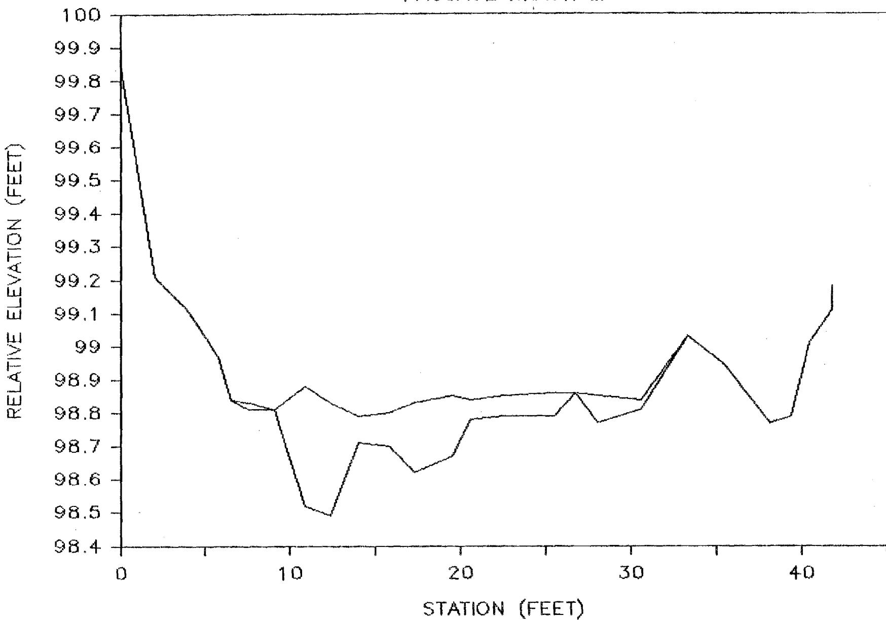
Appendix Figure D-4B. Cross sectional profile of Passage Reach III in Side Channel 21, October 16, 1984.
