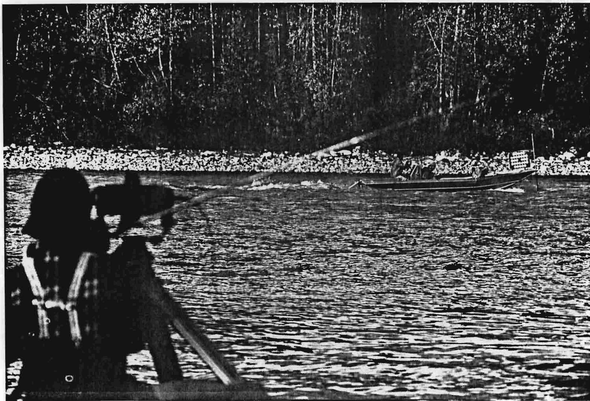
Plate 10. Use of an EDM distance finder for determining cross section profiles.
