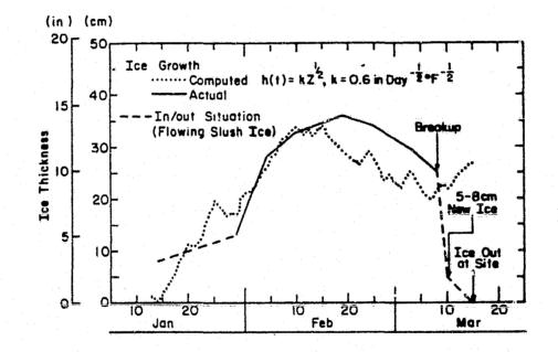
Figure 2-4. Actual measured ice thickness vs. computed growth at Shelburne Point, Vermont: Winter 1975-76.
