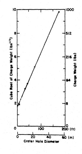
Figure 3-2. Relationship of explosive weight to crater hole (good for ice 1 to 10 feet thick).
