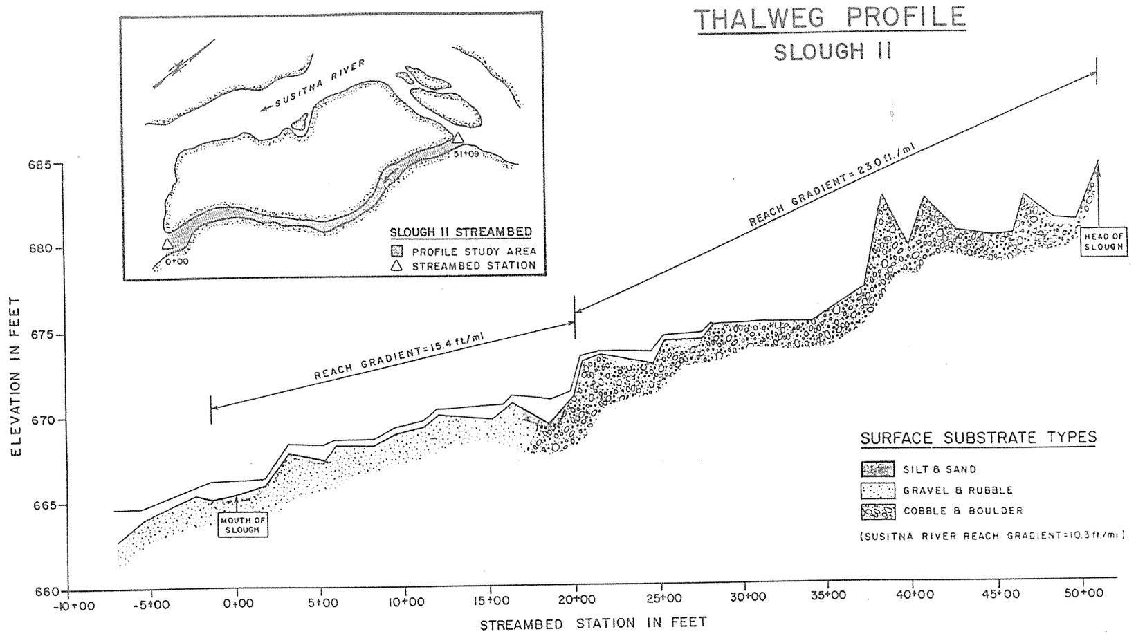
Figure 4I-3-28. Streambed profile for Slough 11.
