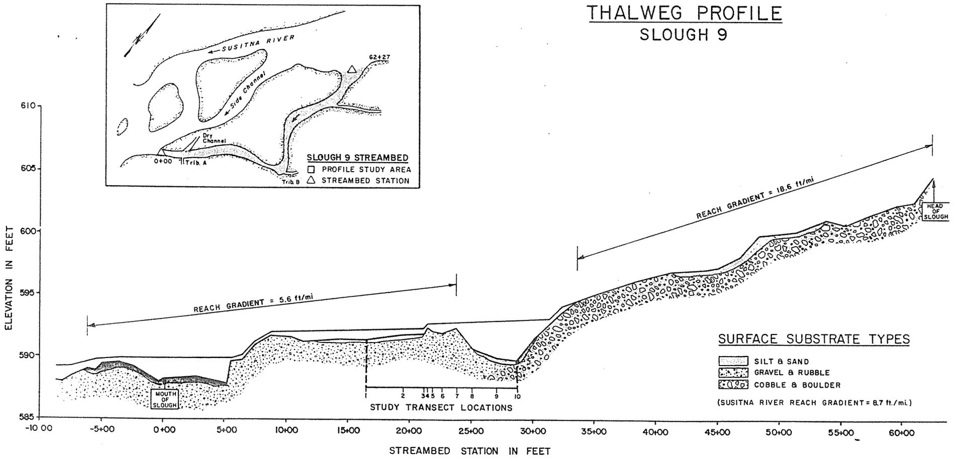
Figure 4I-3-27. Streambed profile for Slough 9.
