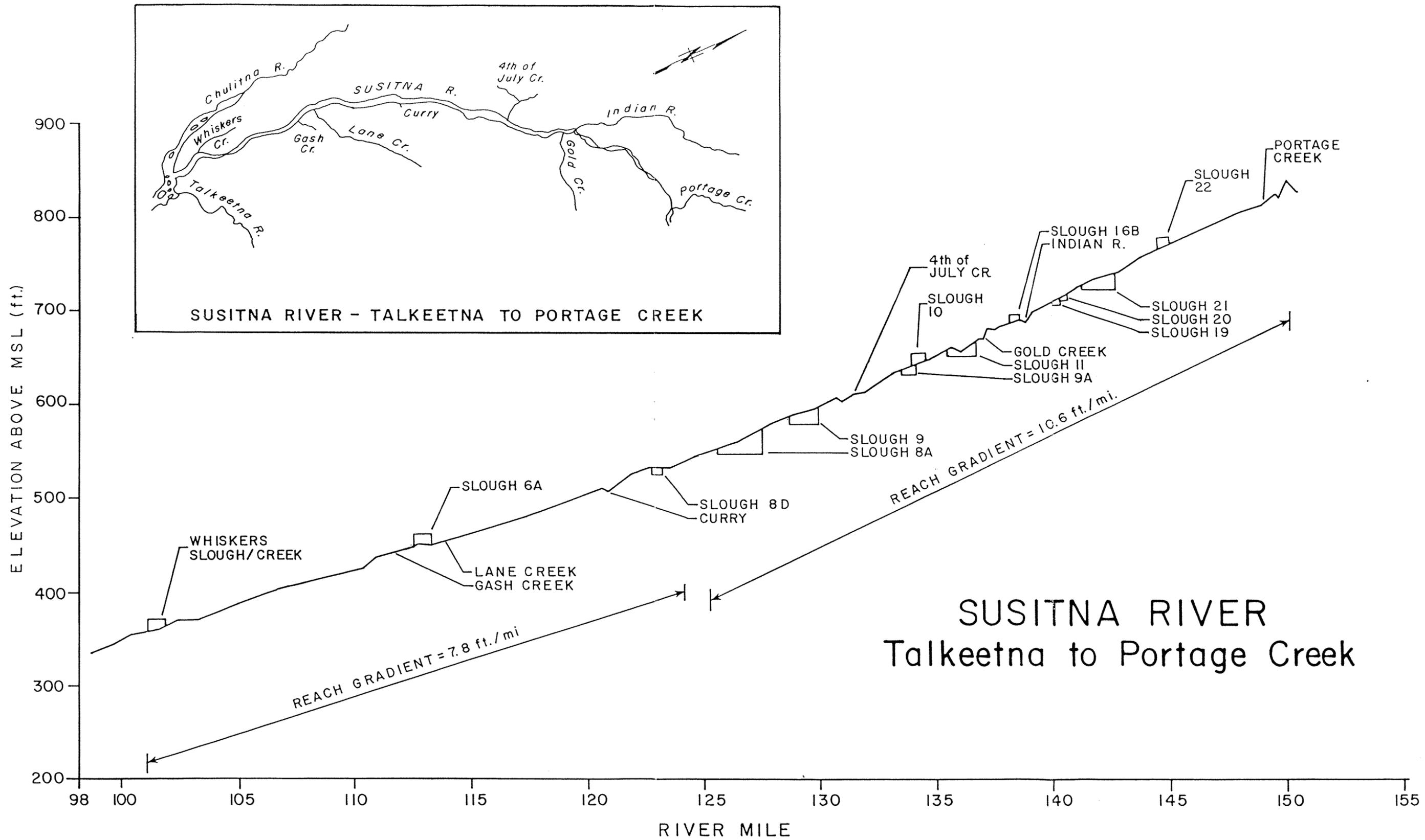
Figure 4I-3-1. Gradient of the Susitna River from Portage Creek to Whiskers Creek/Slough.
