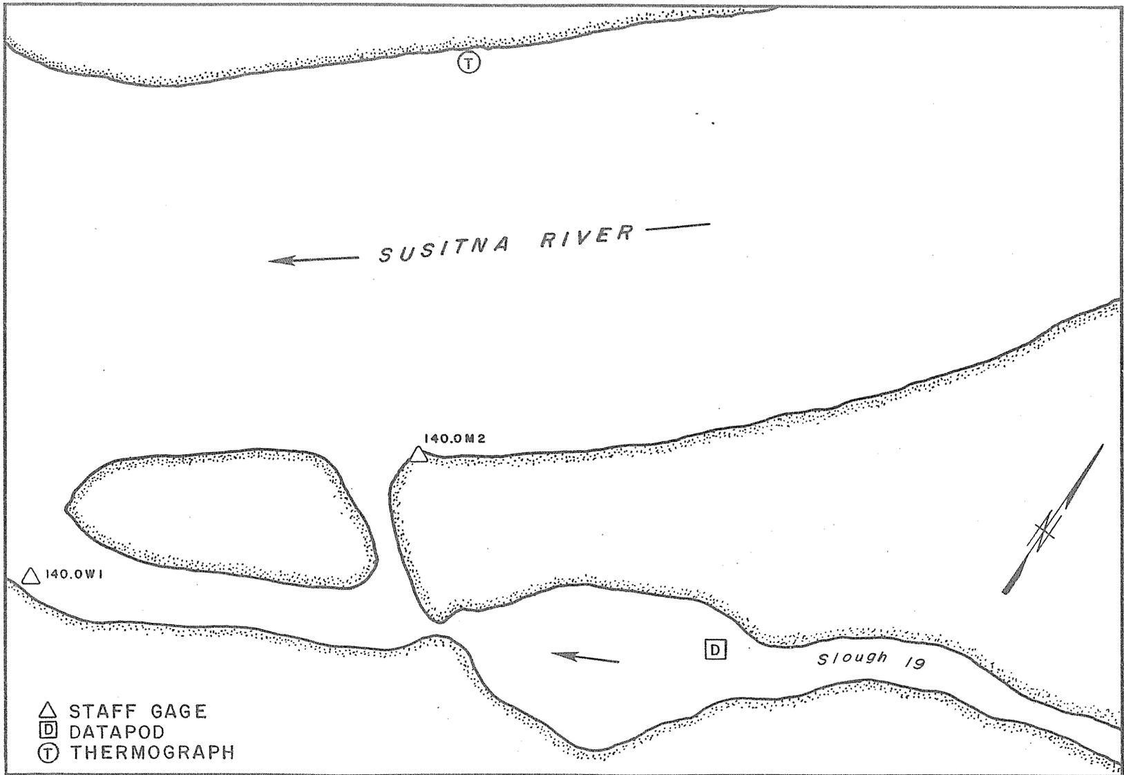
Figure 4E-3-3 Planimetric site map of Slough 19, RM 140.0, GC S31N02W10DBB.
