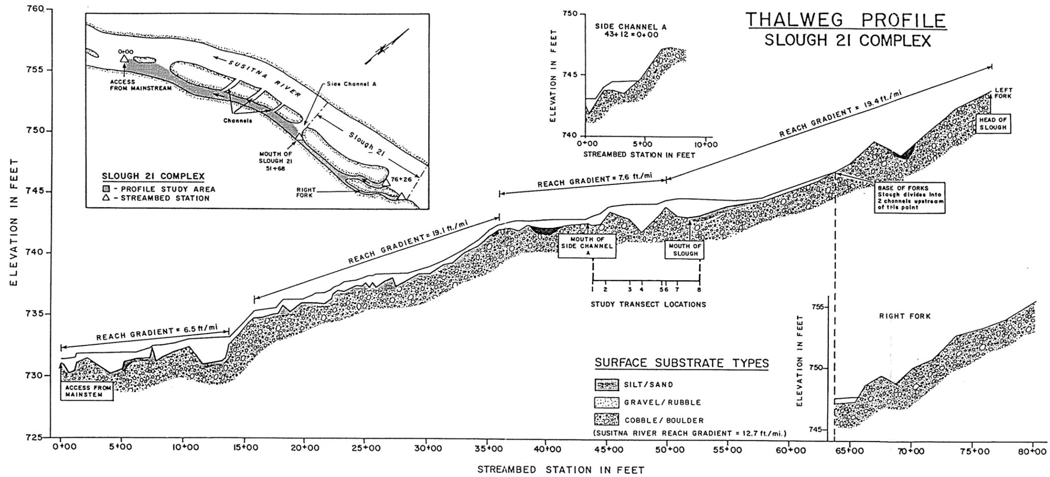
Figure 4I-3-29. Streambed profile for Slough 21.
