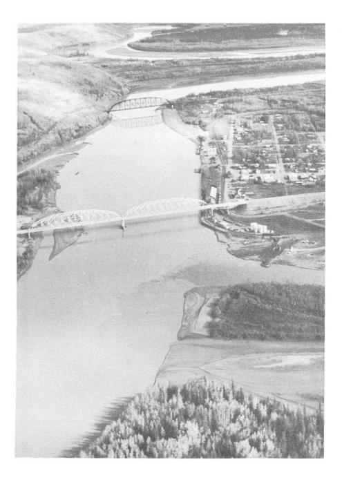
Town of Nenana, at confluence of Tanana River and Nenana River, which flows in from lower right. Double-span bridge is for the Anchorage-Fairbanks Highway; single-span bridge is for Alaska Railroad.
