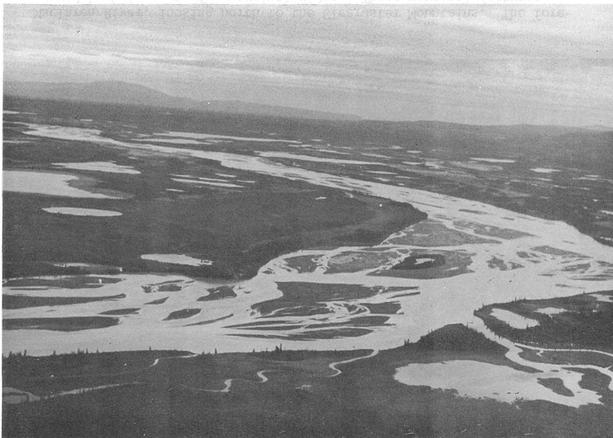
Impoundment area of Denali damsite. The Susitna here is a meandery, aggrading river, the surrounding land is very poorly drained and underlain by fairly continuous permafrost.
