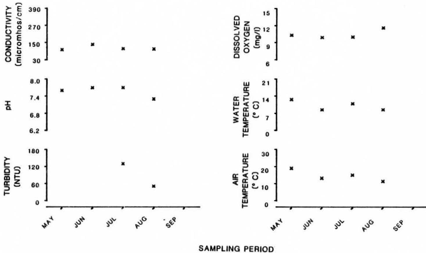
Figure 61. Physiochemical parameters versus time (May-September, 1981) for Mainstem Susitna 50' upstream of Deadman Creek (R.M. 183.4, Geographic Code 32N05E26CAA)
