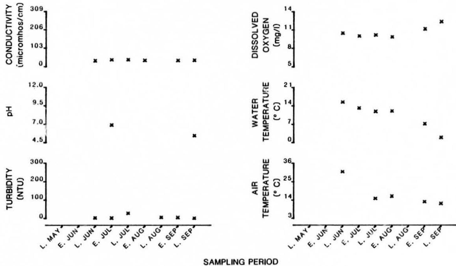
Figure 22. Physiochemical parameters versus time (May-September, 1981)
