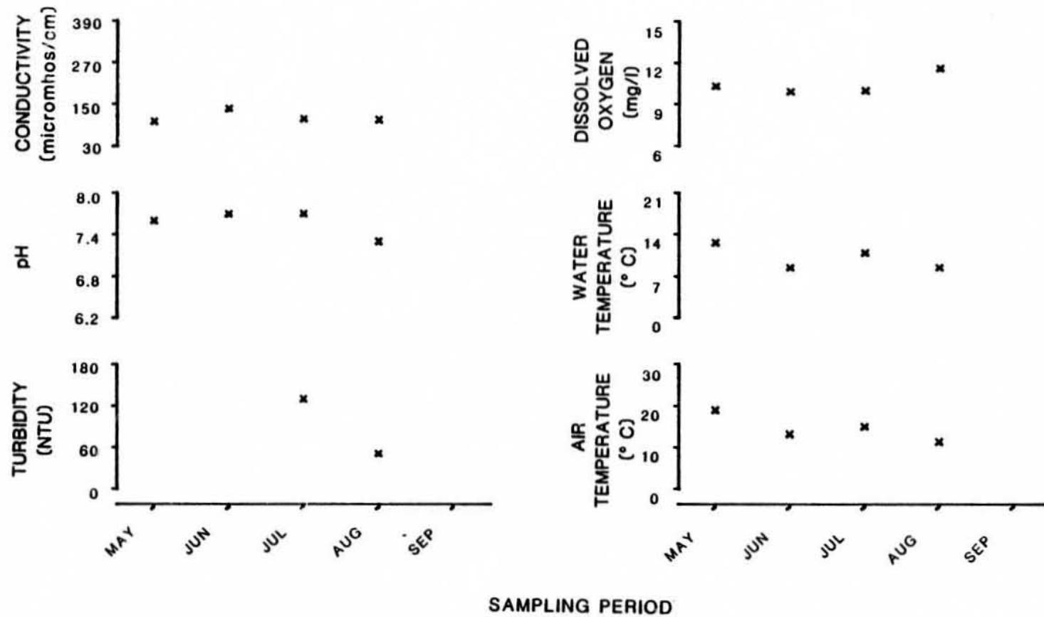
Figure 61. Physiochemical parameters versus time (May-September, 1981) for Mainstem Susitna 50' upstream of Deadman Creek (R.M. 103.4, Geographic Code 32N05E26CAA)
