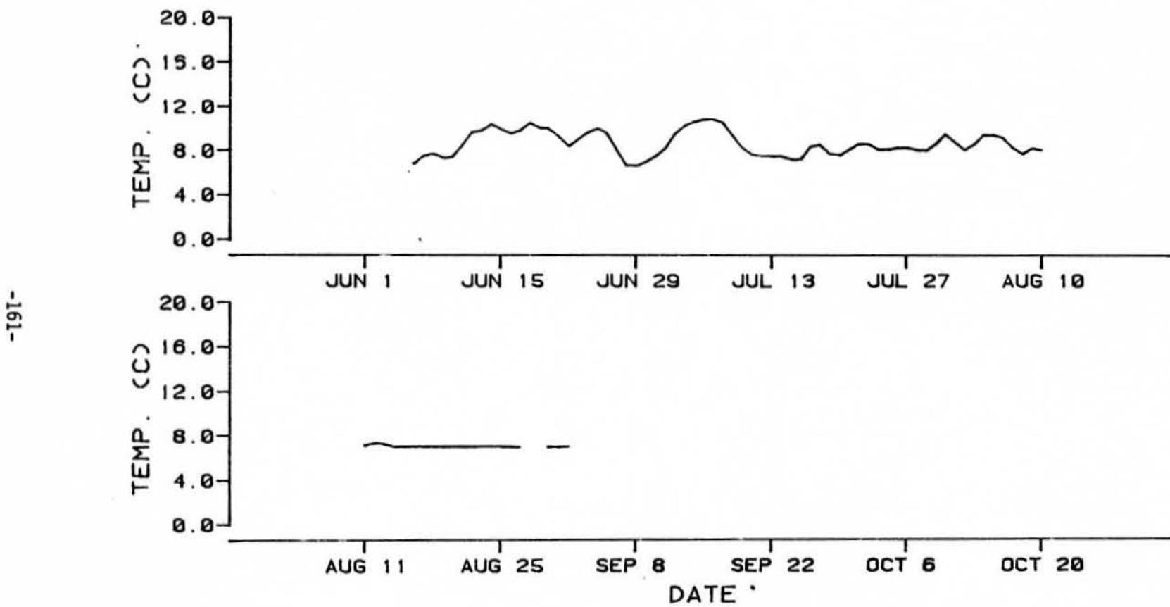
Figure 96. Water temperature versus time for the mainstem Susitna River above Alexander Creek (R.M. 10.1, 15N07W05CDB).
