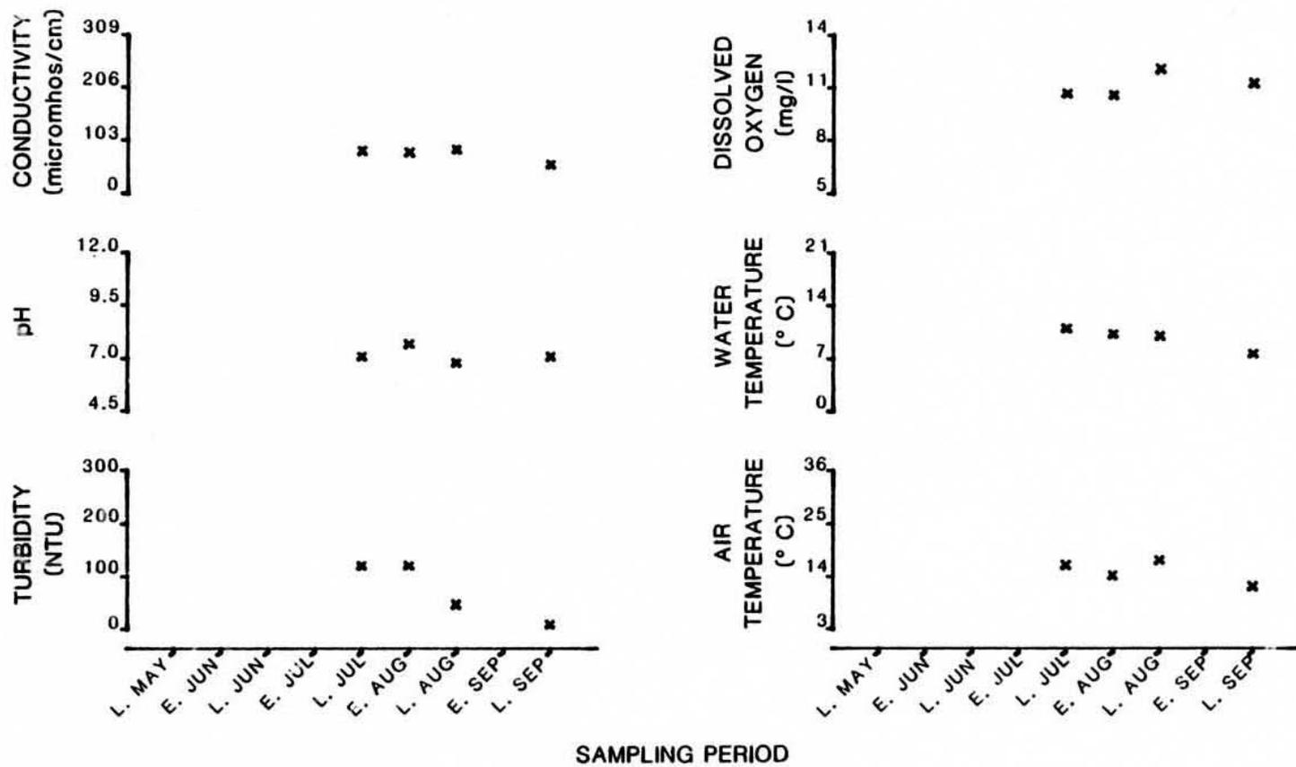
Figure 30. Physiochemical parameters versus time (May-September, 1981)
