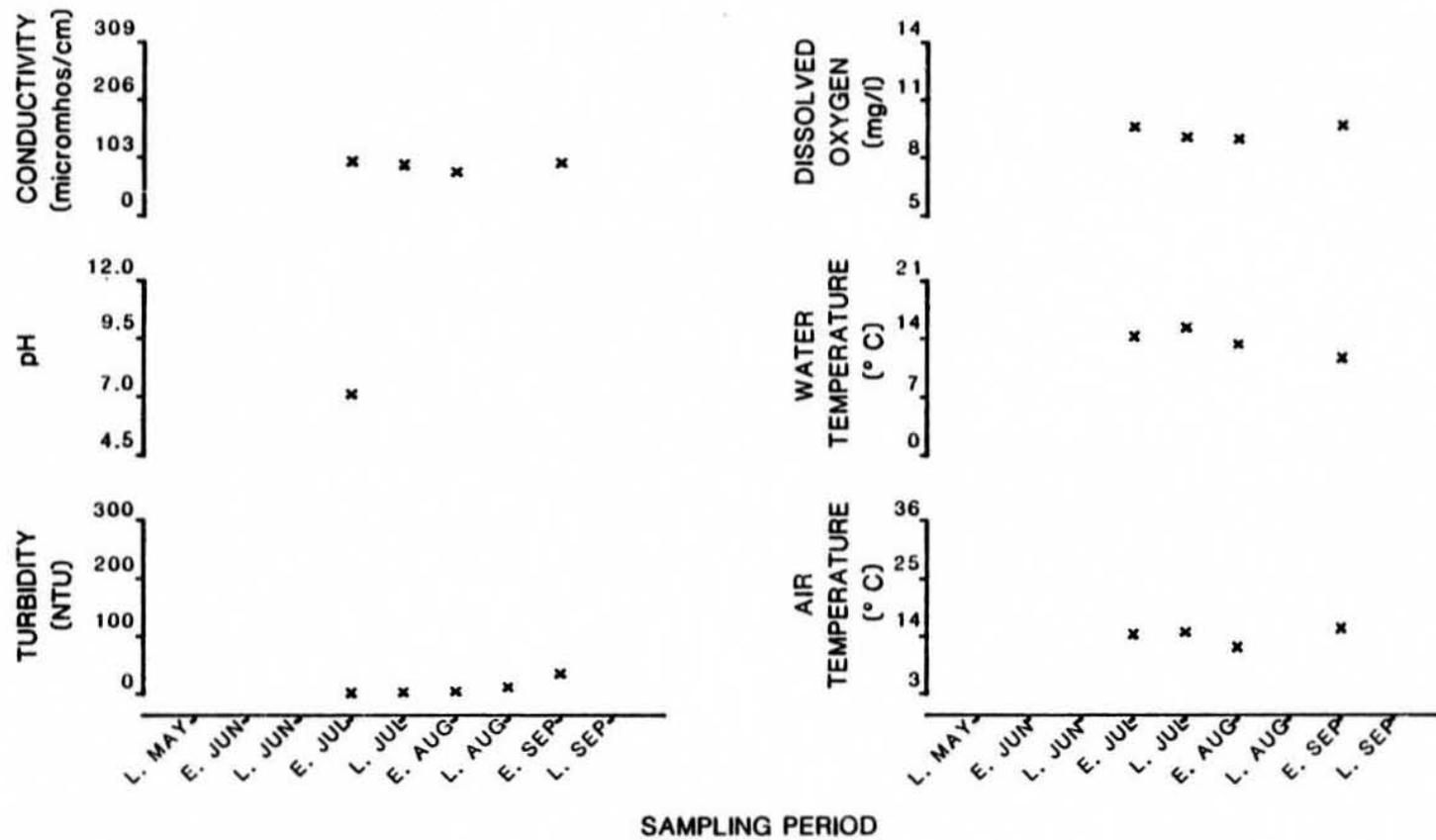
Figure 12. Physiochemical parameters versus time (May-September, 1981) for Alexander Creek - Site B (R.M. 10.1, Geographic Code 16N07W32CCB)
