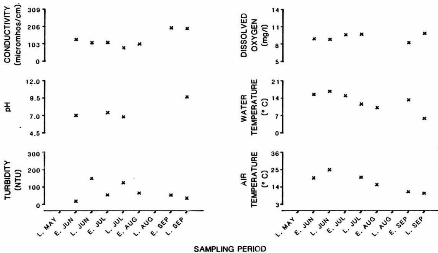
Figure 15. Physiochemical parameters versus time (May-September, 1981)
