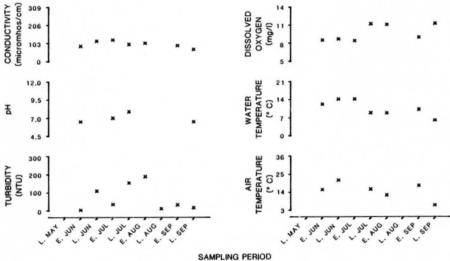
Figure 14. Physiochemical parameters versus time (May-September, 1981) for Anderson Creek (R.M. 23.8, Geographic Code 17N07W29DDD)
