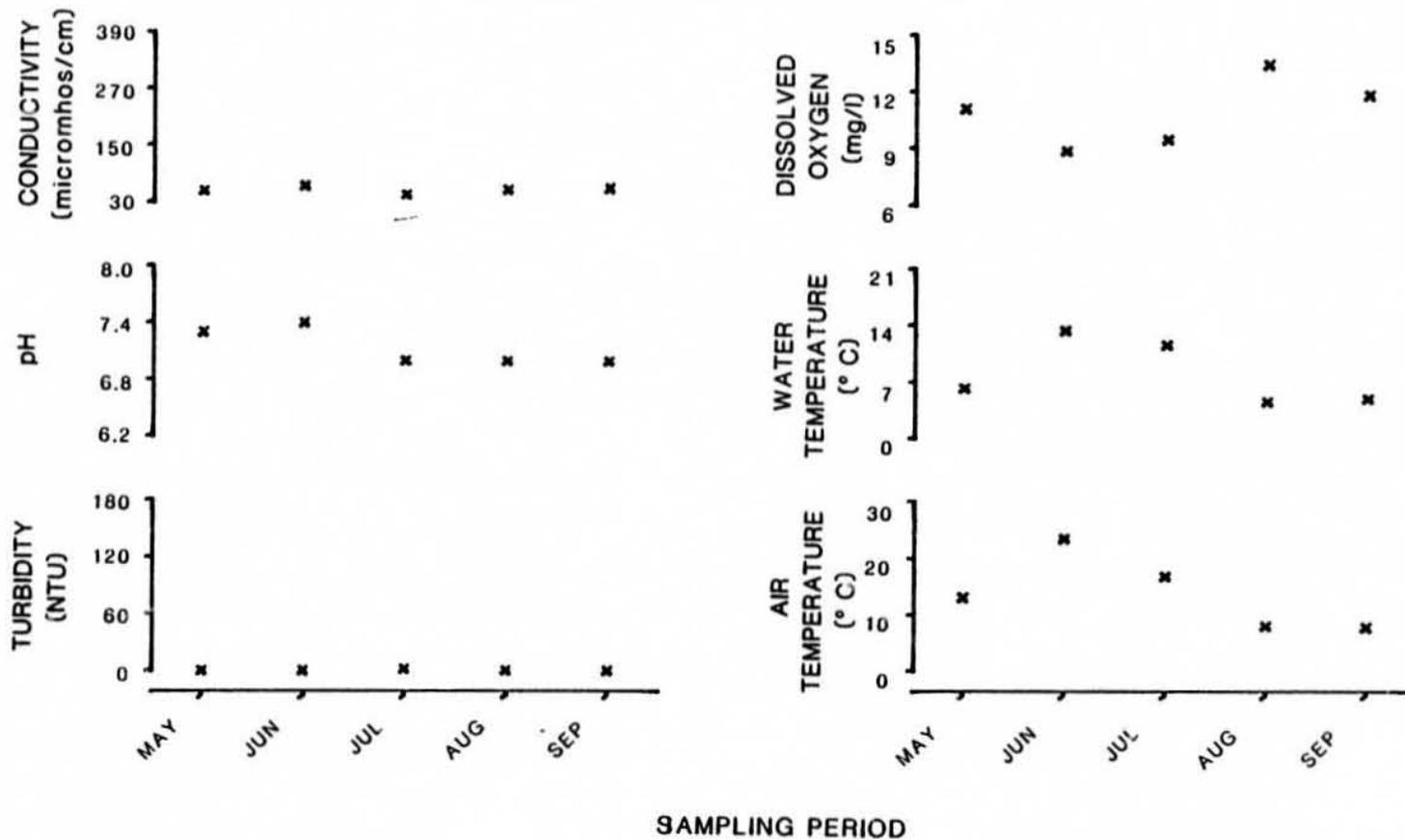
Figure 85. Physiochemical parameters versus time (May-September, 1981)
