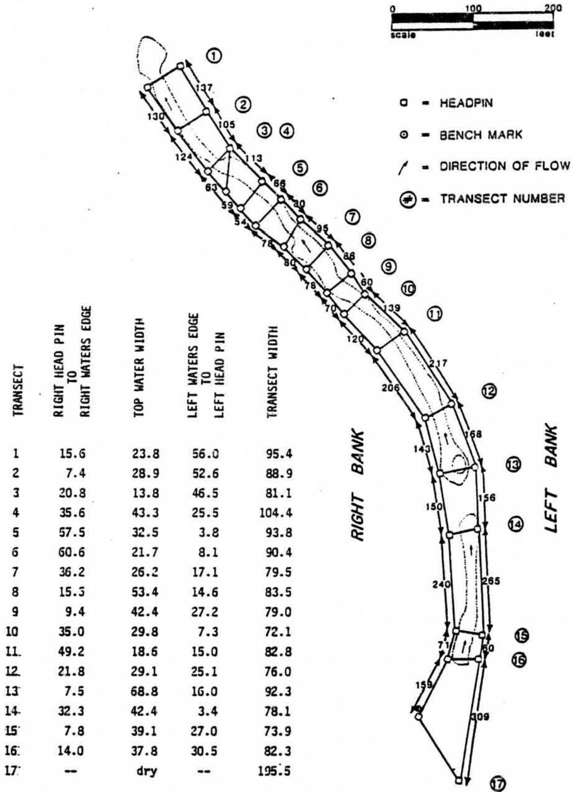
Figure 122. Waters edge location and head pin distance for Slough 16 (R.M. 139, 31N11W17ABD). -201-
