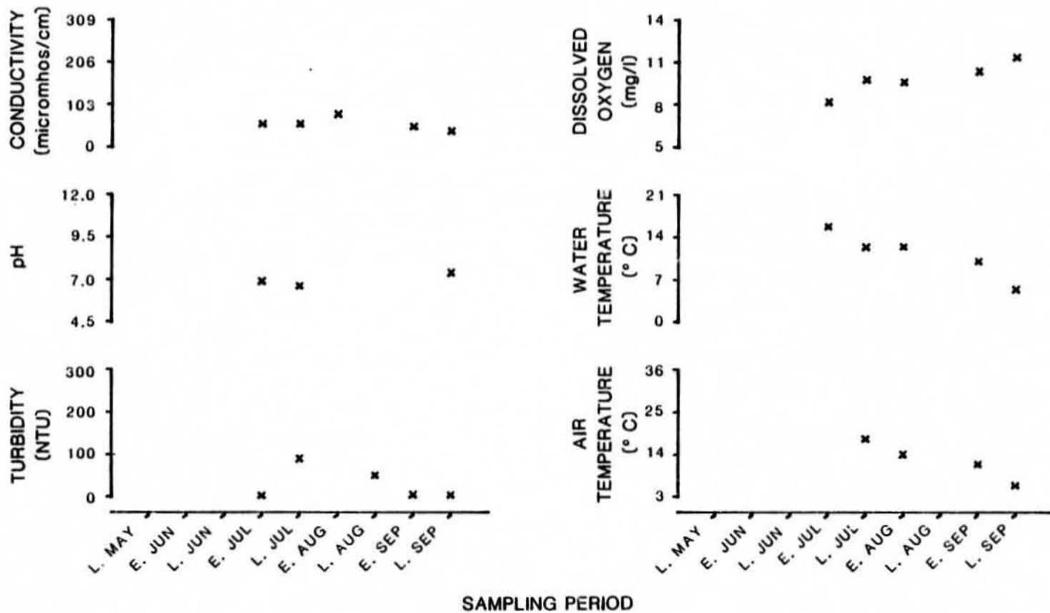
Figure 18. Physiochemical parameters versus time (May-September, 1981) for Deshka River - Site A (R.M. 40.6, Geographic Code 19N06W35BDA)
