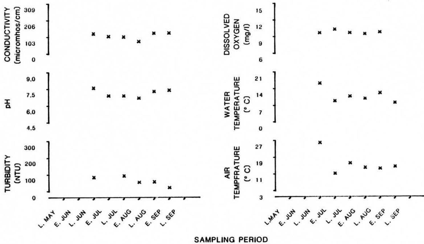
Figure 45. Physiochemical parameters versus time (May-September, 1981)
