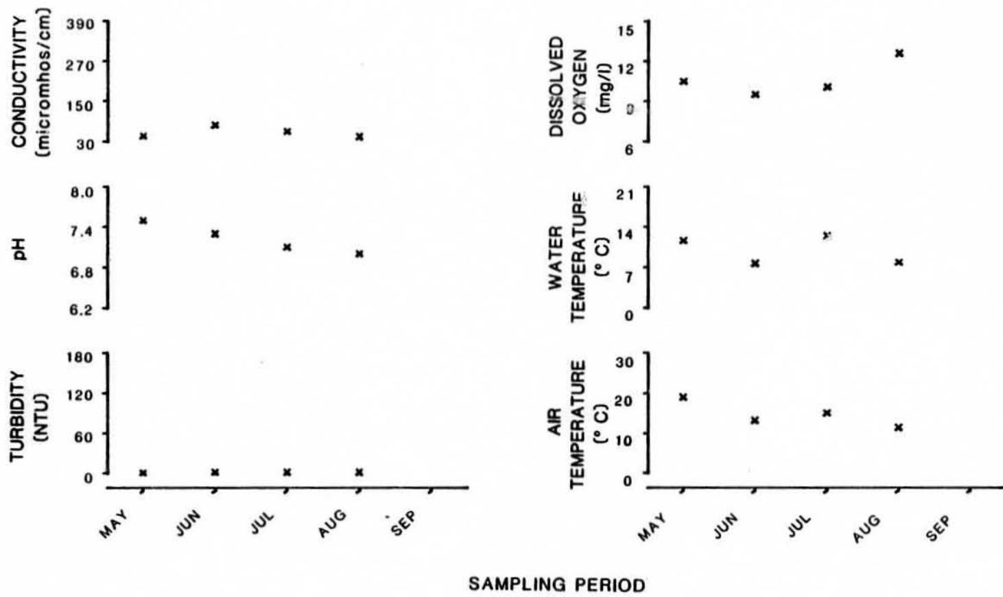
Figure 62. Physiochemical parameters versus time (May-September, 1981)
