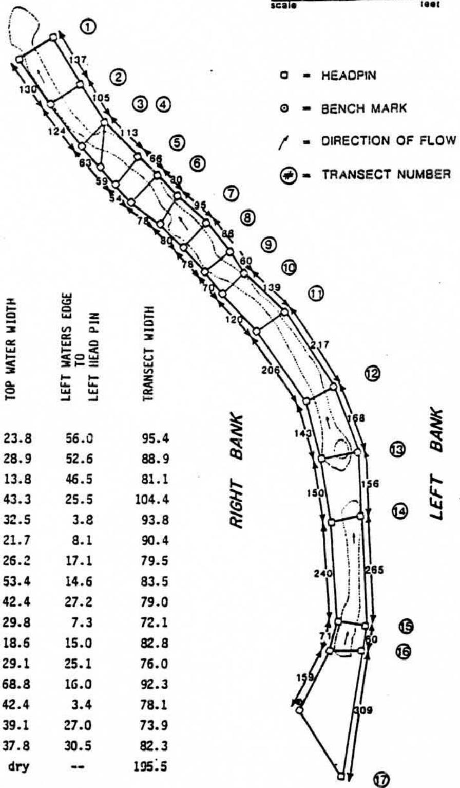
Figure 122. Waters edge location and head pin distance for Slough 16 (R.M. 139, 31N11W17ABD). -201-
