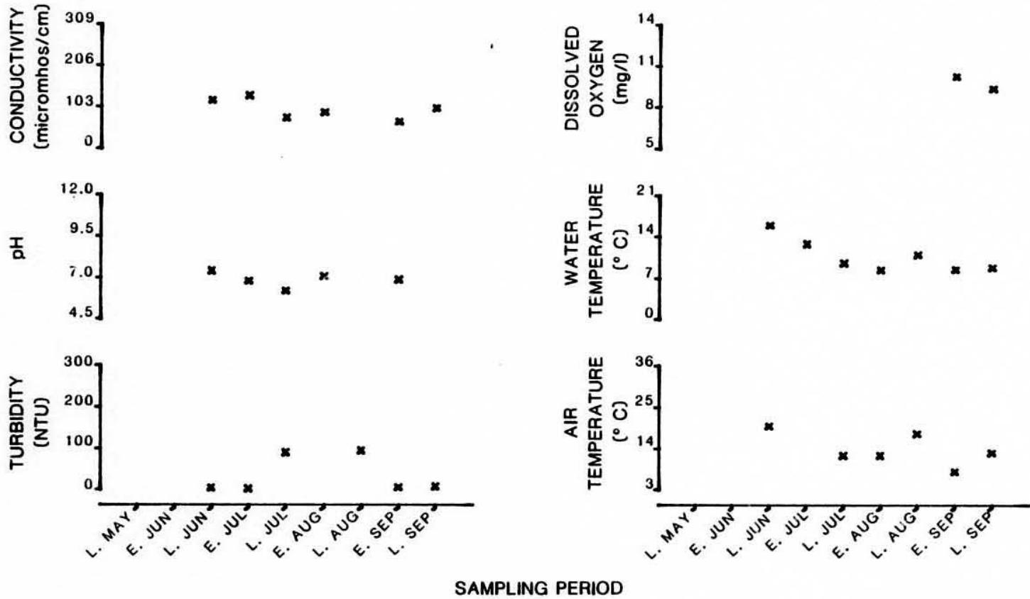
Figure 35. Physiochemical parameters versus time (May-September, 1981)
