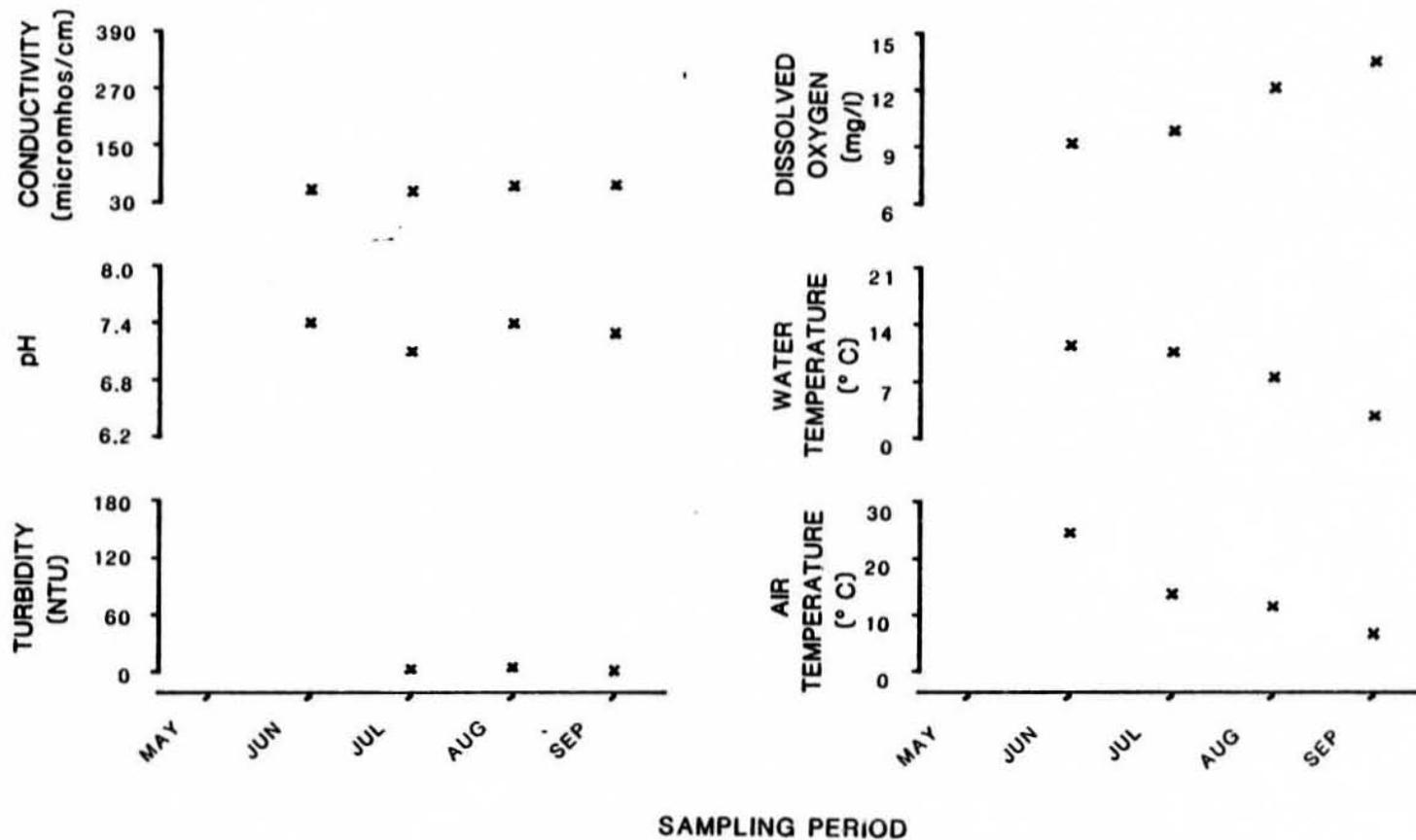
Figure 75. Physiochemical parameters versus time (May-September, 1981)
