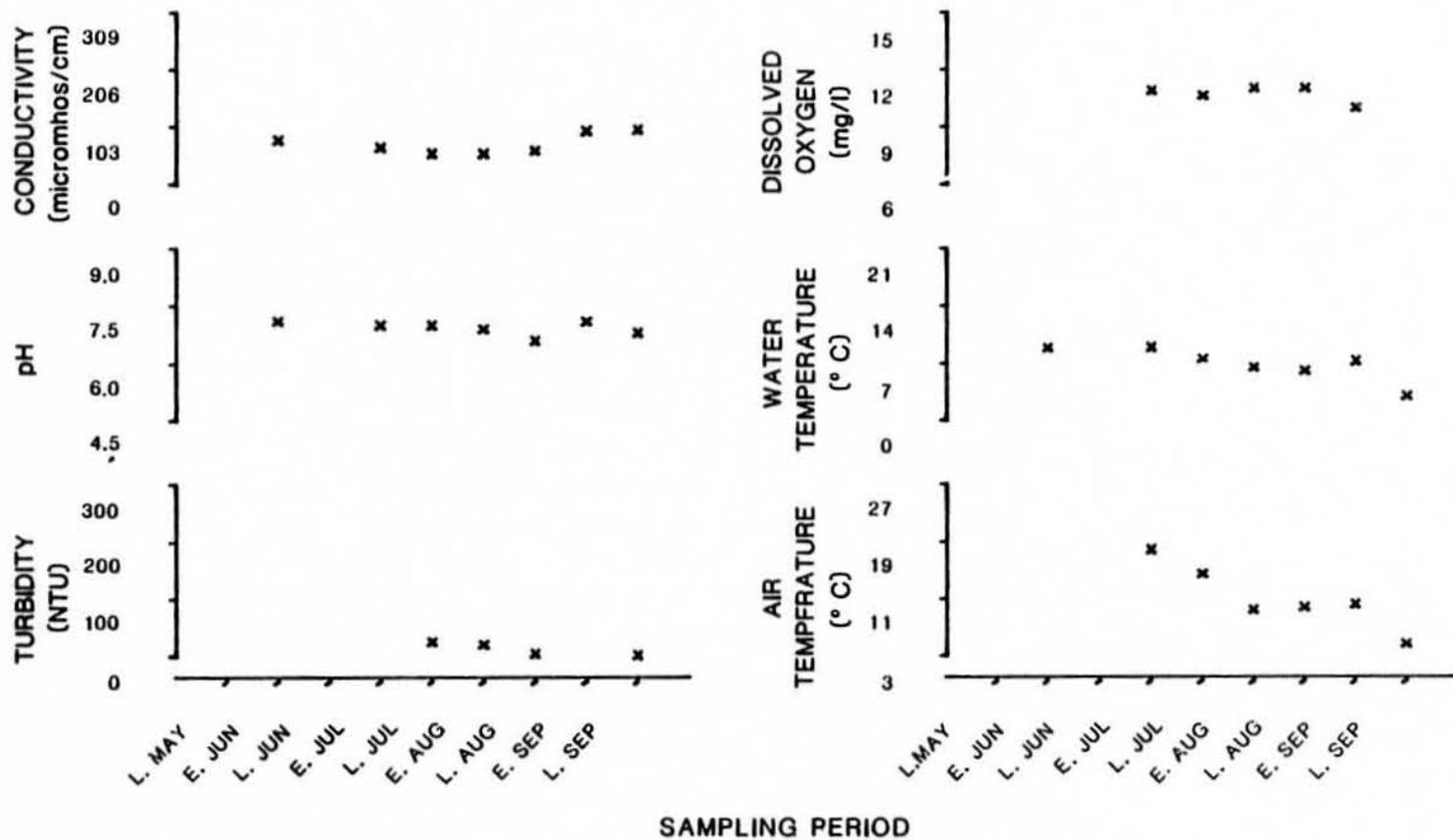
Figure 55. Physiochemical parameters versus time (May-September, 1981)
