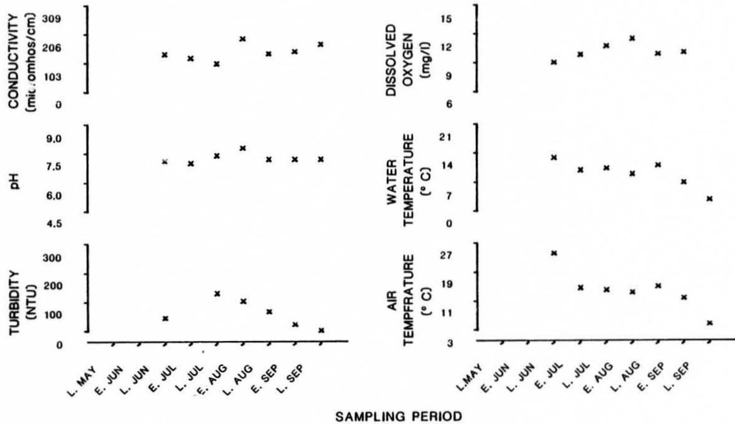
Figure 49. Physiochemical parameters versus time (May-September, 1981)
