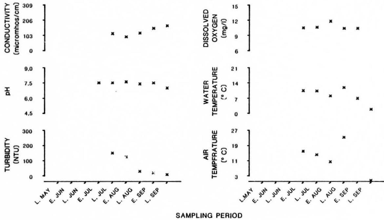
Figure 51. Physiochemical parameters versus time (May-September, 1981) for Mainstem Susitna - Inside Bend (Su-Gold)
