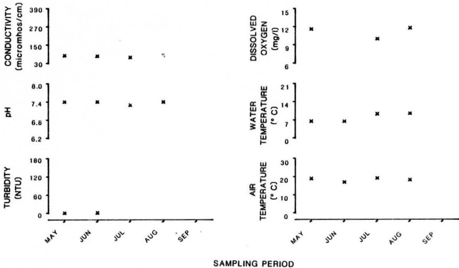
Figure 57. Physiochemical parameters versus time (May-September, 1981) for Fog Creek - Site 2 (R.M. 173.9, Geographic Code 31N04E16DBD)
