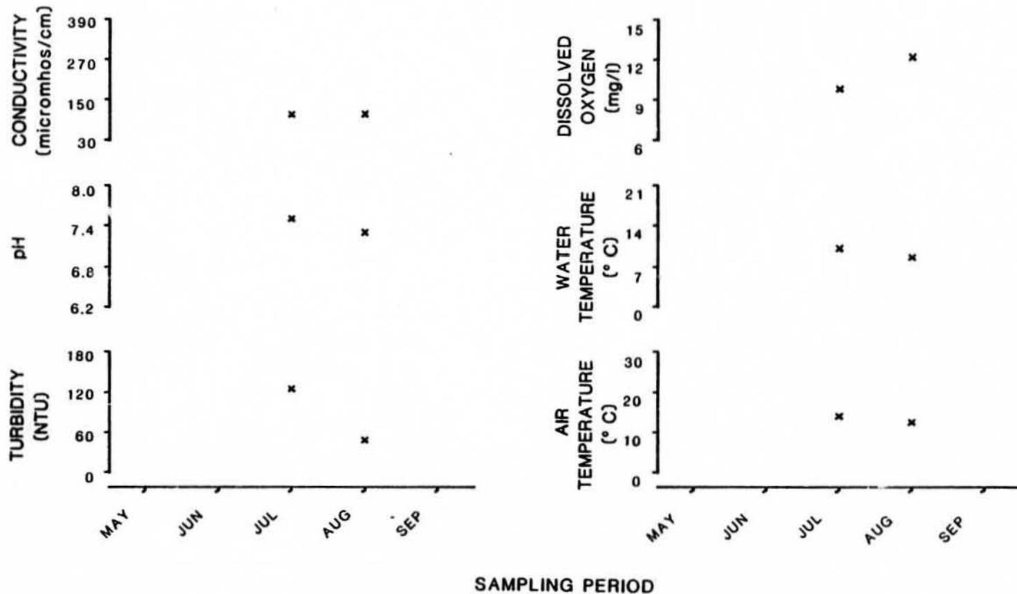
Figure 59. Physiochemical parameters versus time (May-September, 1981) for Mainstem Susitna 50' upstream of Tsusena River (R.M. 178.9, Geographic Code 32N04E36ADB)
