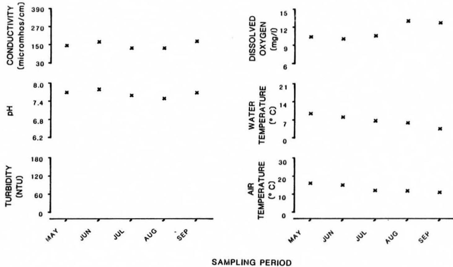
Figure 78. Physiochemical parameters versus time (May-September, 1981)
