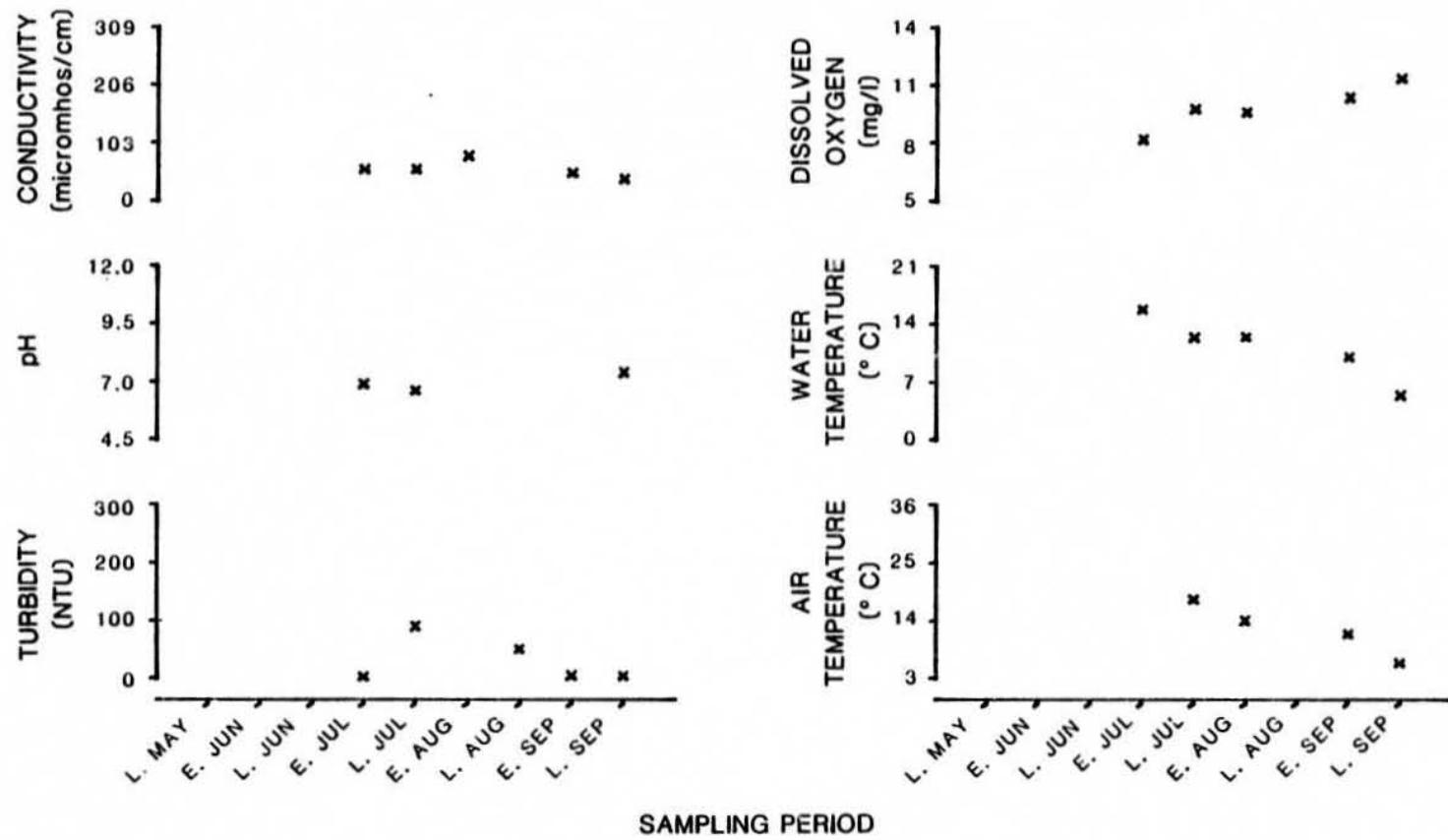
Figure 18. Physiochemical parameters versus time (May-September, 1981)
