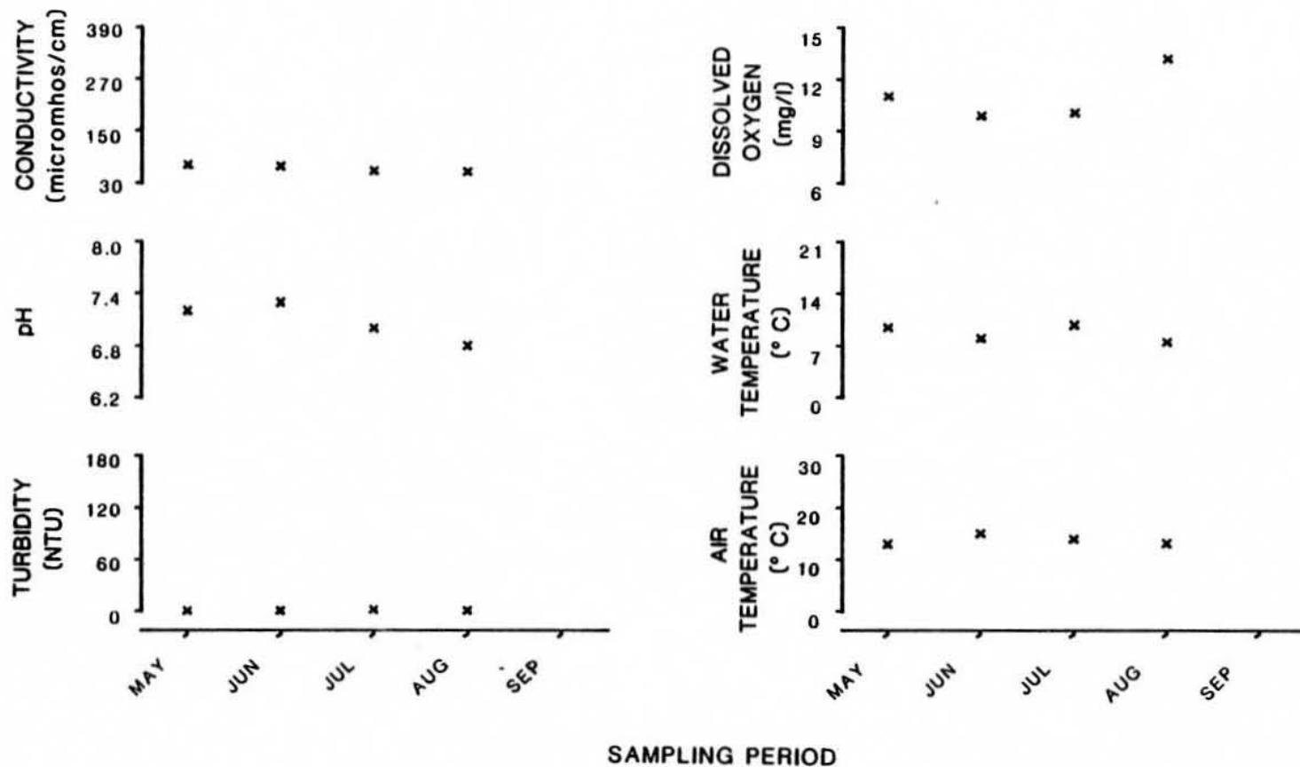
Figure 60. Physiochemical parameters versus time (May-September, 1981)
