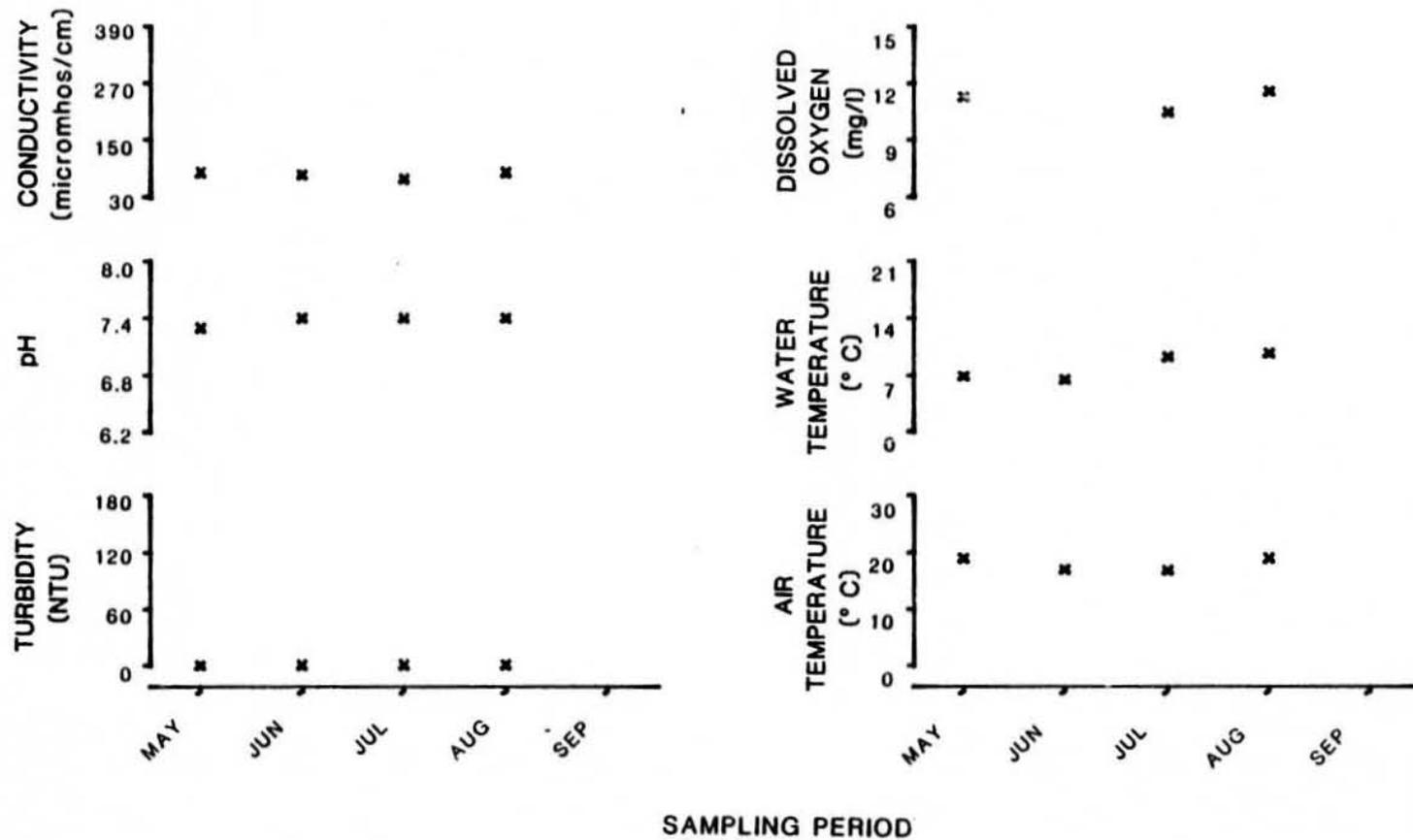
Figure 58. Physiochemical parameters versus time (May-September, 1981) for Fog Creek - Site 3 (R.M. 173.9, Geographic Code 31N04E16DAD)
