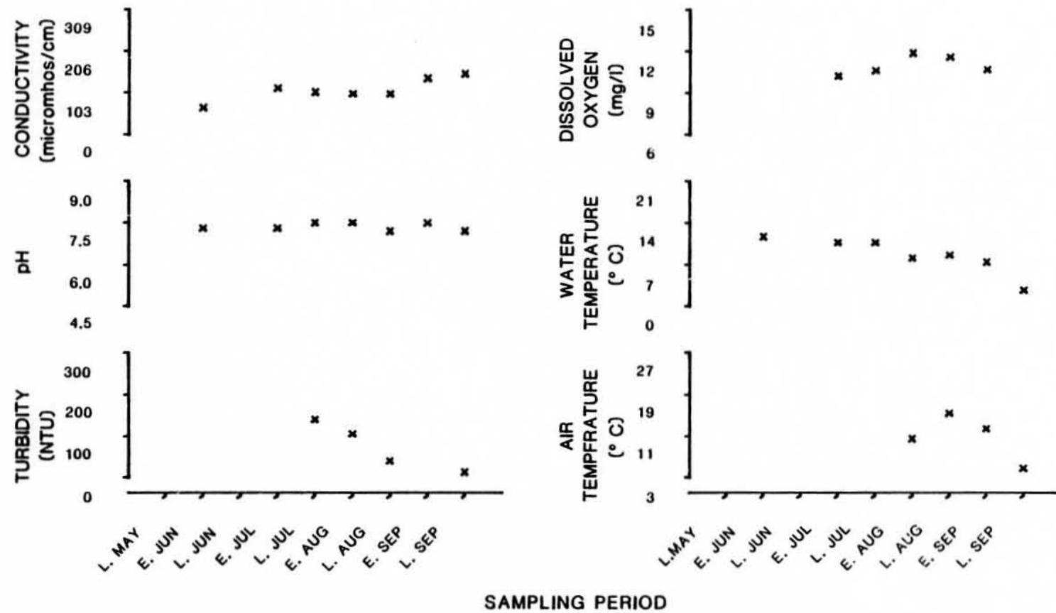
Figure 54. Physiochemical parameters versus time (May-September, 1981) for Mainstem Susitna - Island (Su-Island)
