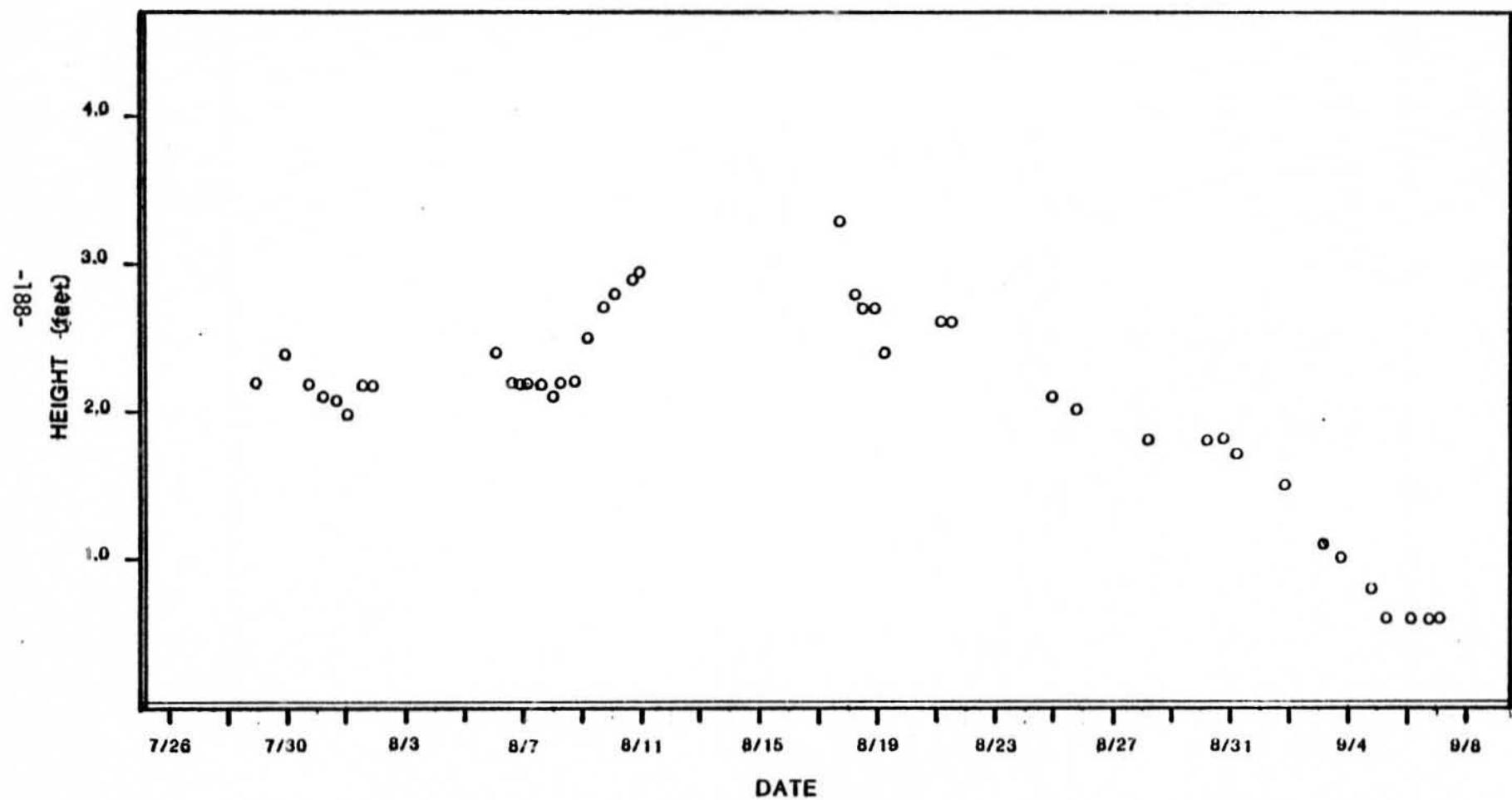
Figure 119. Stage versus time for the AA Sunshine west bank fishwheel site (RM 81.0, 24N05W23CCA).
