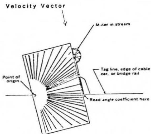
Figure 2. Measurement of Horizontal Angles (from Buchanan and Somers 1973).
