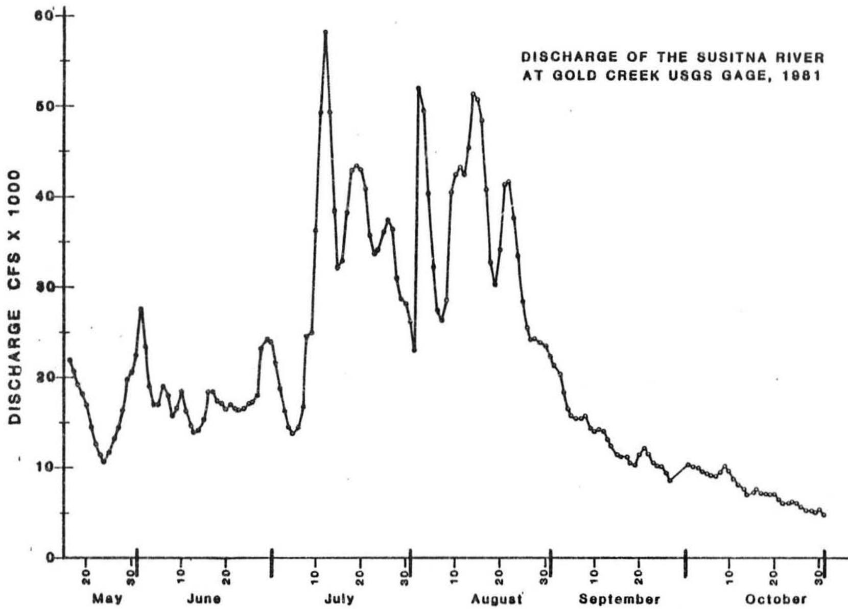
Figure 1. Mainstem Susitna River discharge at Gold Creek versus time (May - October, 1981).
