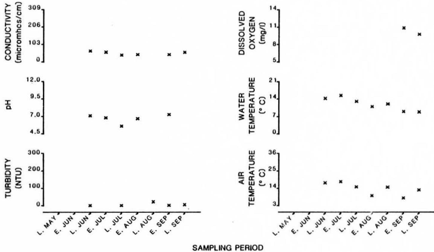
Figure 34. Physiochemical parameters versus time (May-September, 1981)
