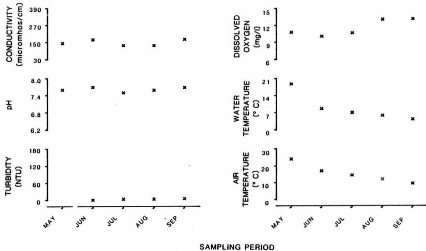
Figure 81. Physiochemical parameters versus time (May-September, 1981)
