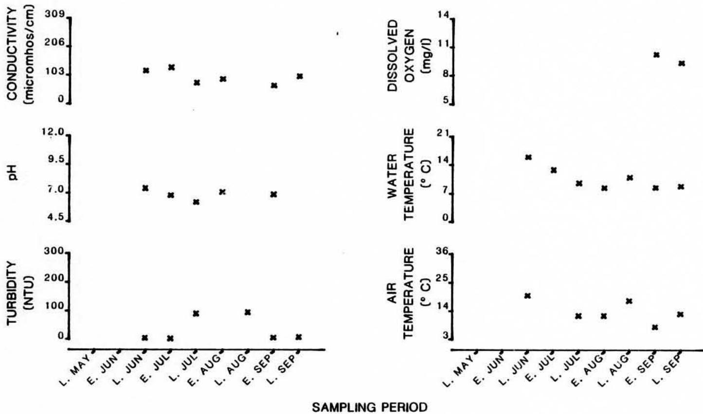
Figure 35. Physiochemical parameters versus time (May-September, 1981) for Birch Creek Slough (R.M. 88.4, Geographic Code 25N05W25DCC)
