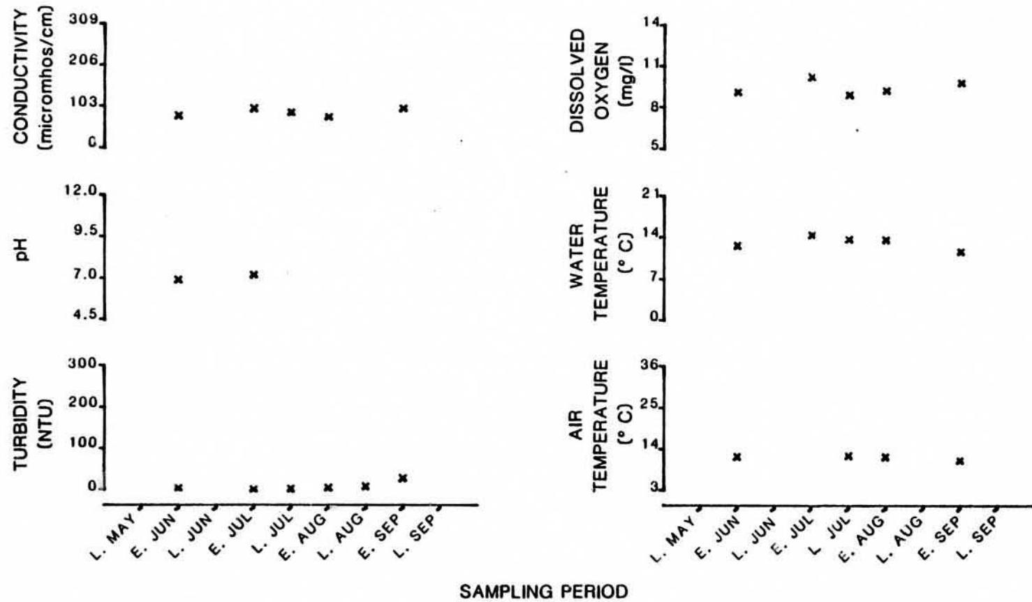
Figure 11 . Physiochemical parameters versus time (May-September, 1981)
