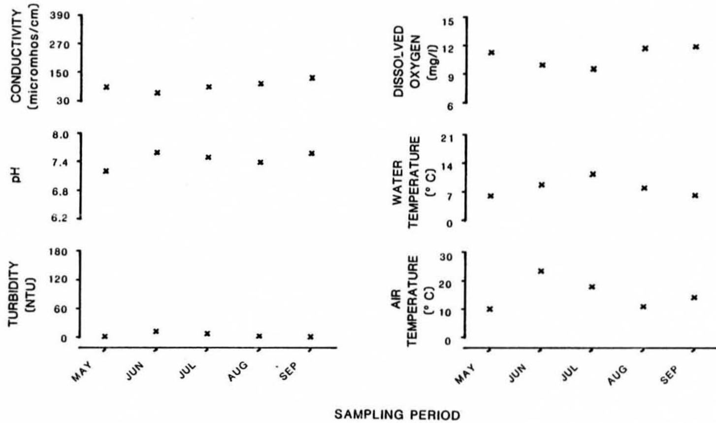
Figure 93. Physiochemical parameters versus time (May-September, 1981)
