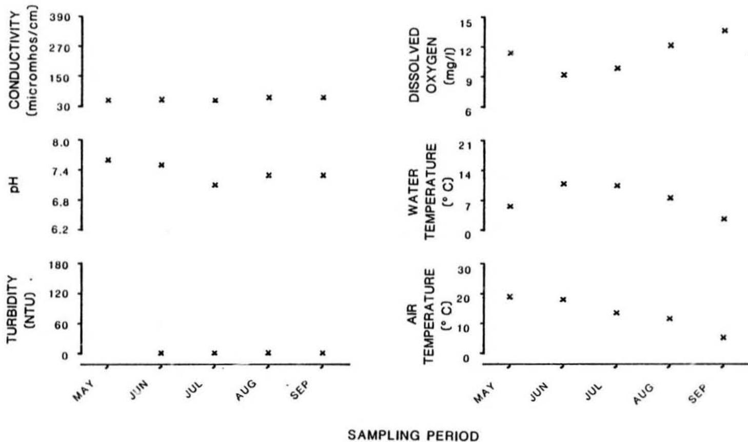
Figure 73. Physiochemical parameters versus time (May-September, 1981)
