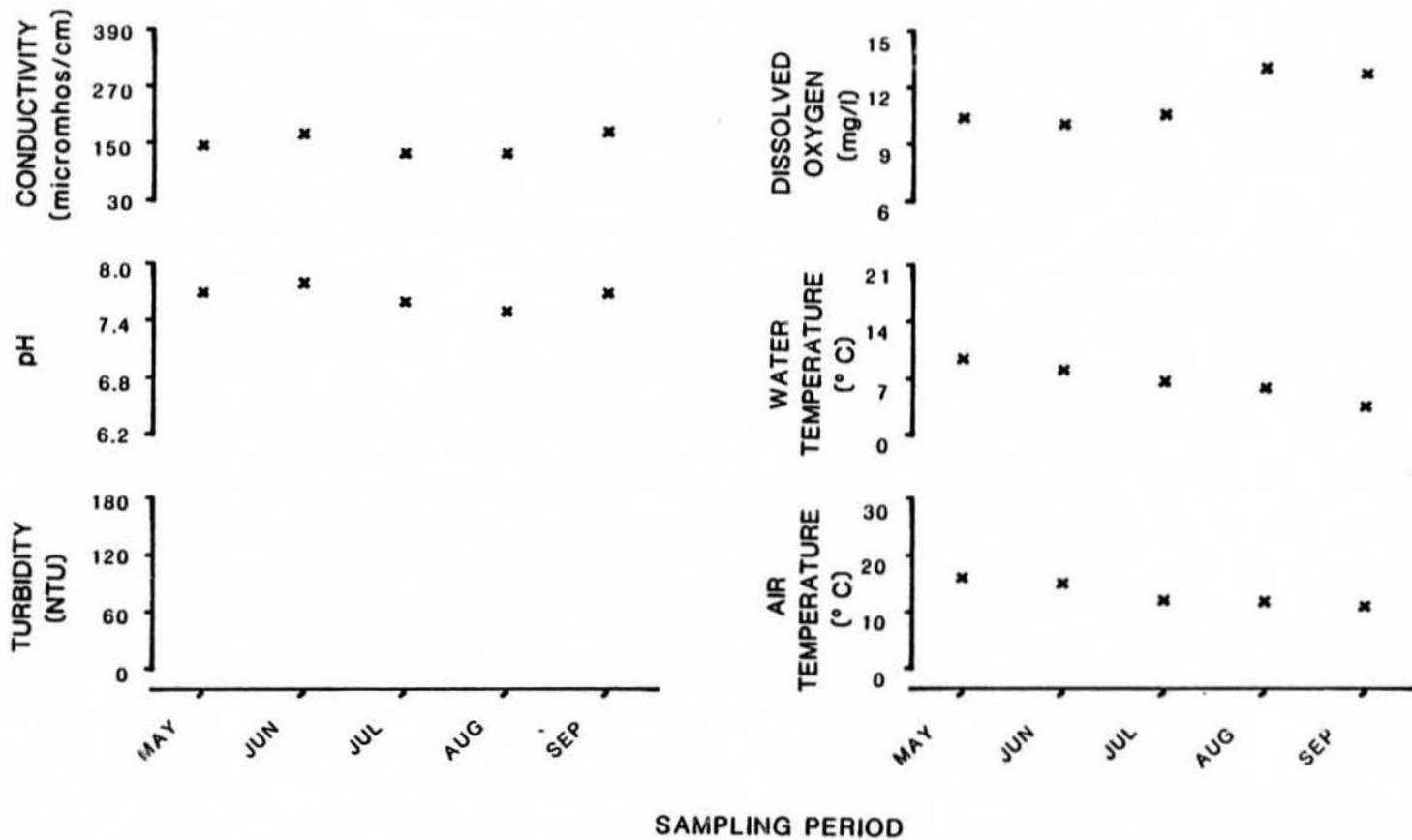
Figure 78. Physiochemical parameters versus time (May-September, 1981)
