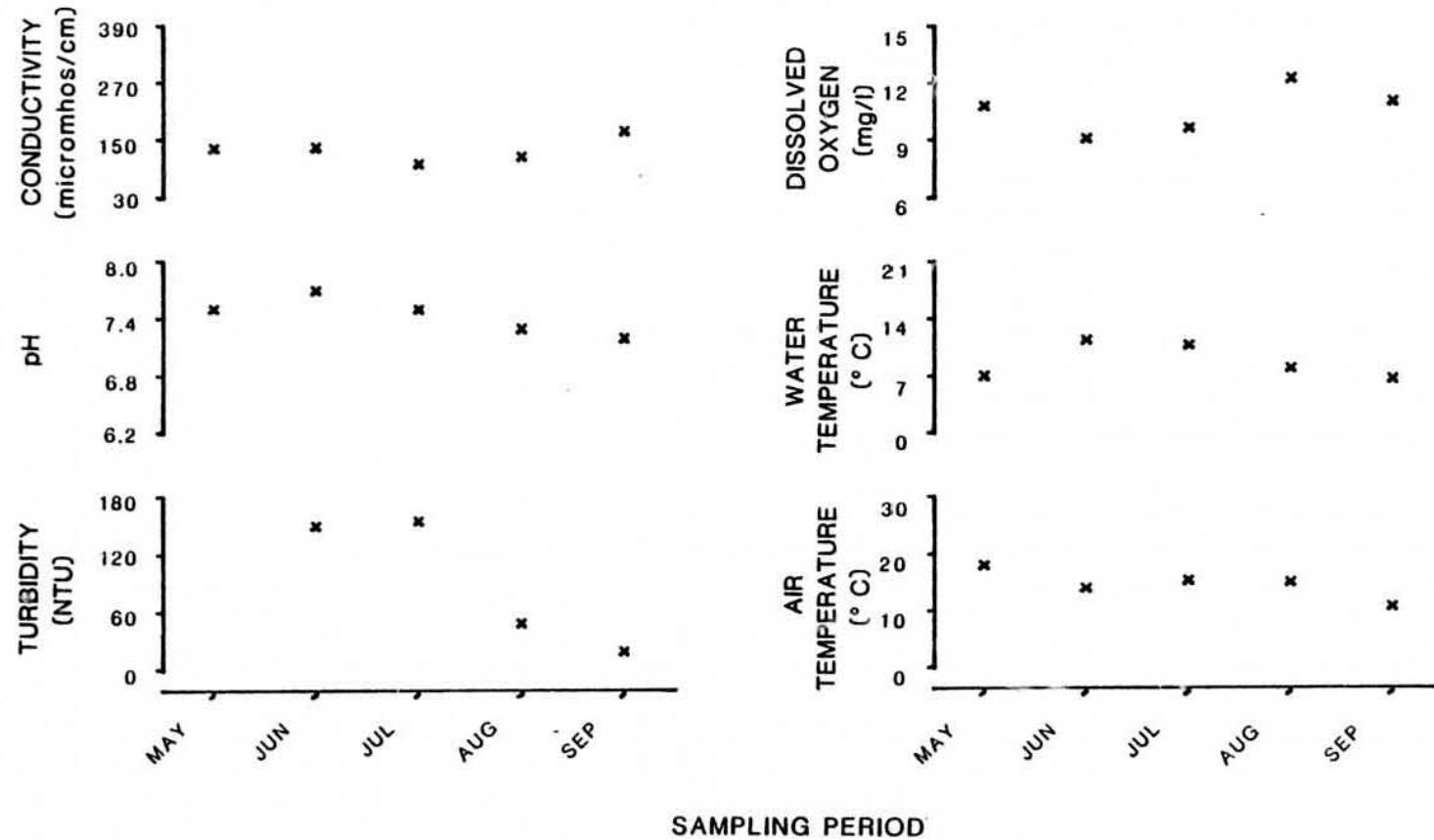
Figure 76. Physiochemical parameters versus time (May-September, 1981) for Mainstem Susitna 50' upstream of Jay Creek
