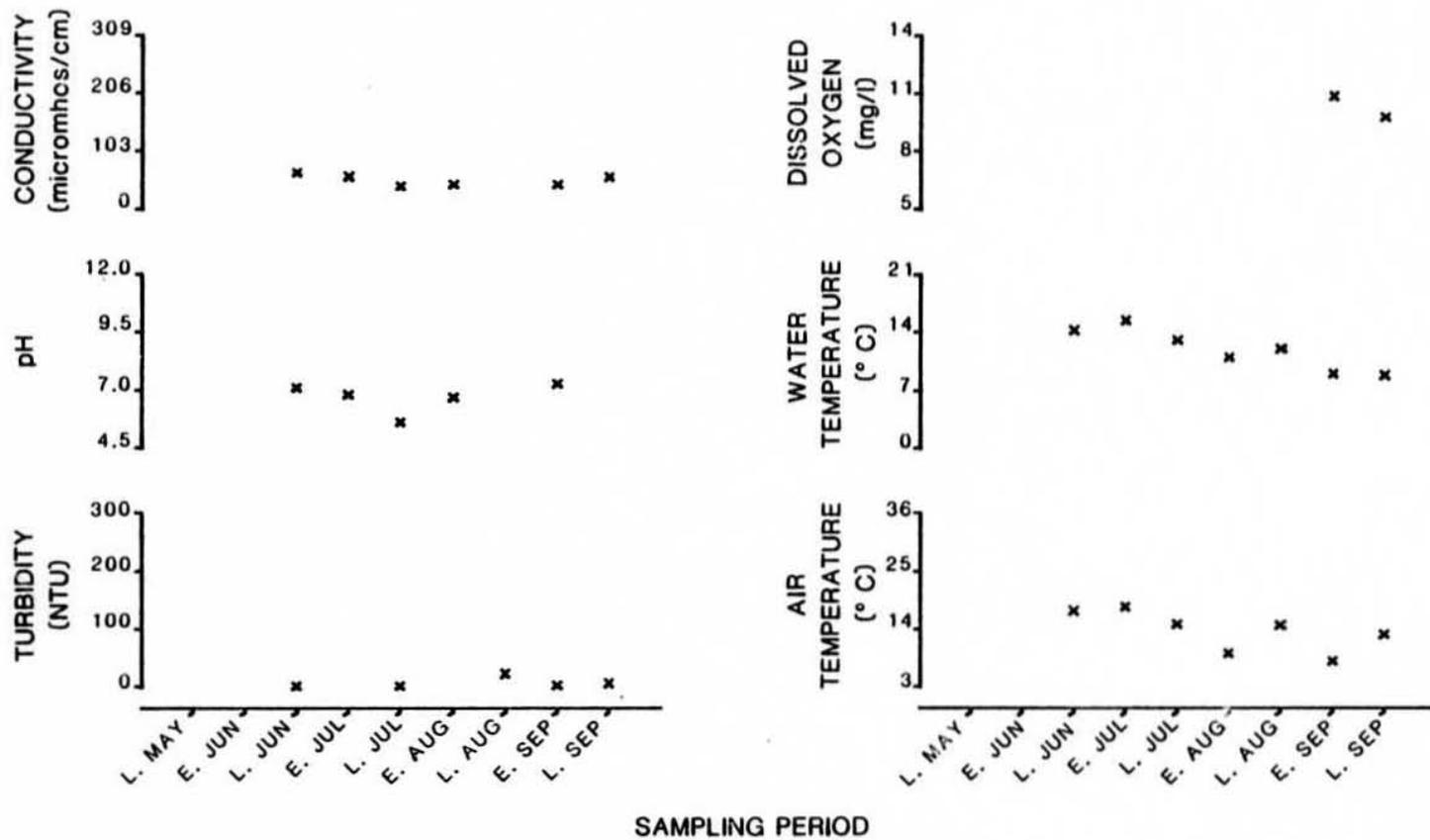
Figure 34. Physiochemical parameters versus time (May-September, 1981) for Sunshine Creek (R.M. 85.7, Geographic Code 24N05W14AAB)
