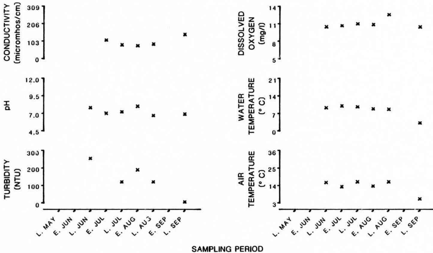
Figure 31. Physiochemical parameters versus time (May-September, 1981)
