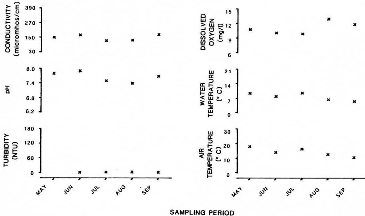
Figure 77. Physiochemical parameters versus time (May-September, 1981)
