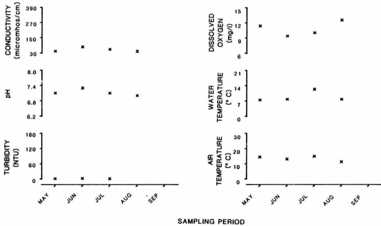
Figure 63. Physiochemical parameters versus time (May-September, 1981)
