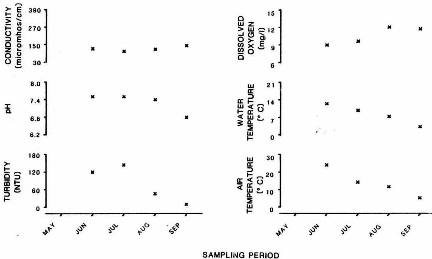
Figure 70. Physiochemical parameters versus time (May-September, 1981) for Mainstem Susitna 50' upstream of Kosina Creek (R.M. 202.4, Geographic Code 31N08E15BAB)
