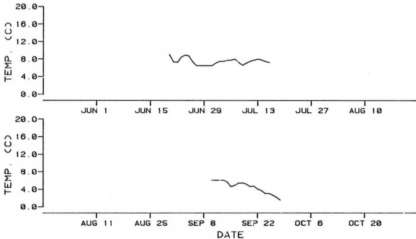
Figure 107. Water temperature versus time for the Chulitna River (R.M. 98.0, 26N05W15DAA).
