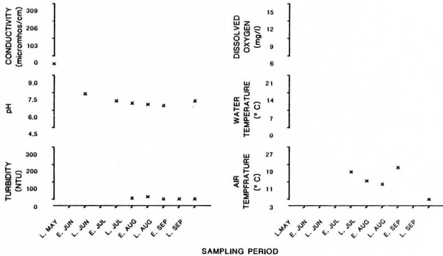
Figure 52. Physiochemical parameters versus time (May-September, 1981)
