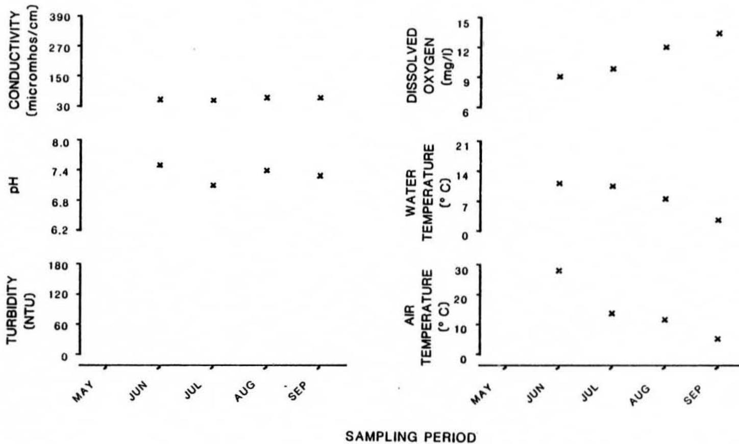
Figure 74. Physiochemical parameters versus time (May-September, 1981)
