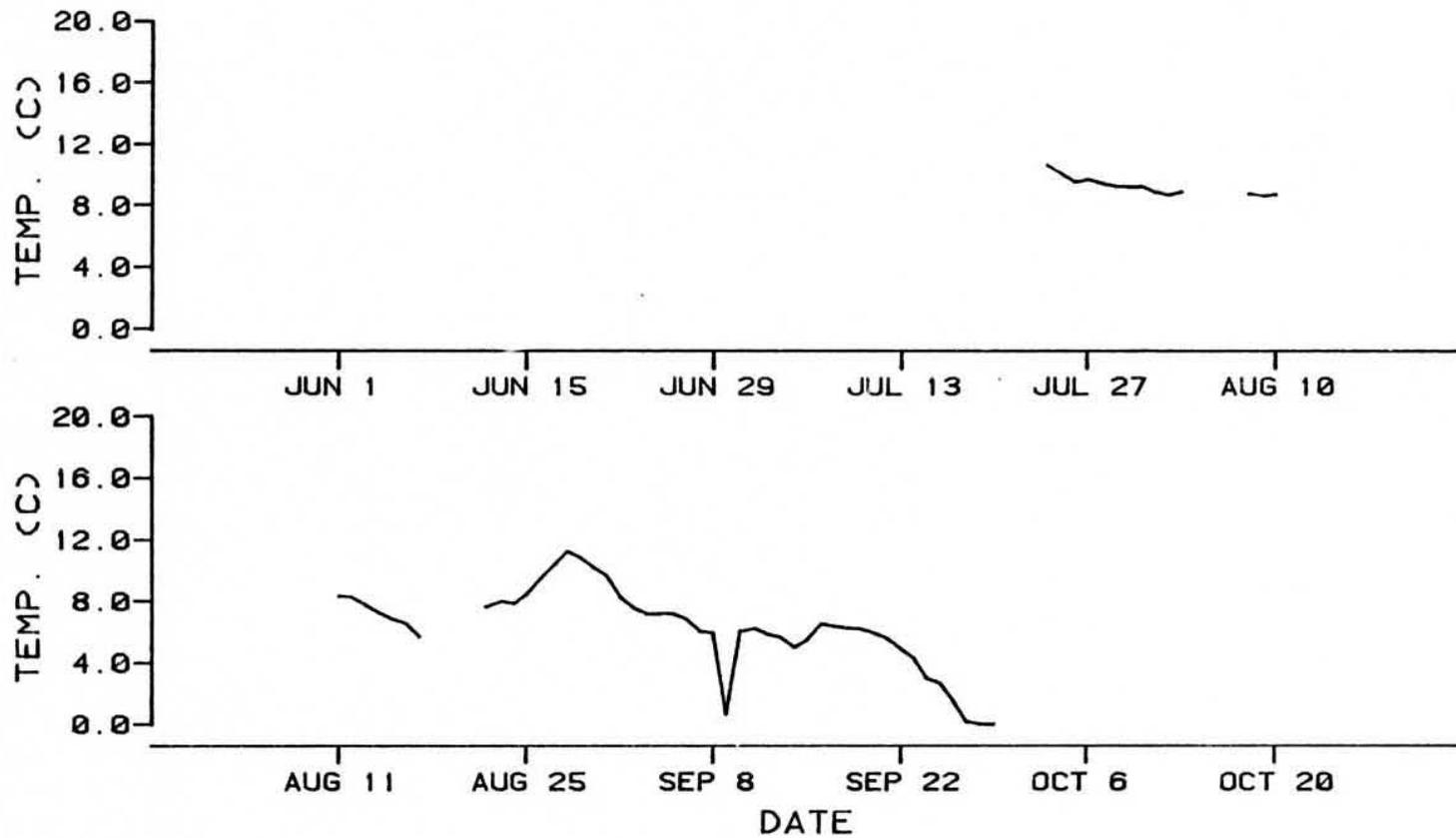
Figure 111. Water temperature versus time for the mainstem Susitna River above Gold Creek (R.M. 136.8, 31N02W20BAA).
