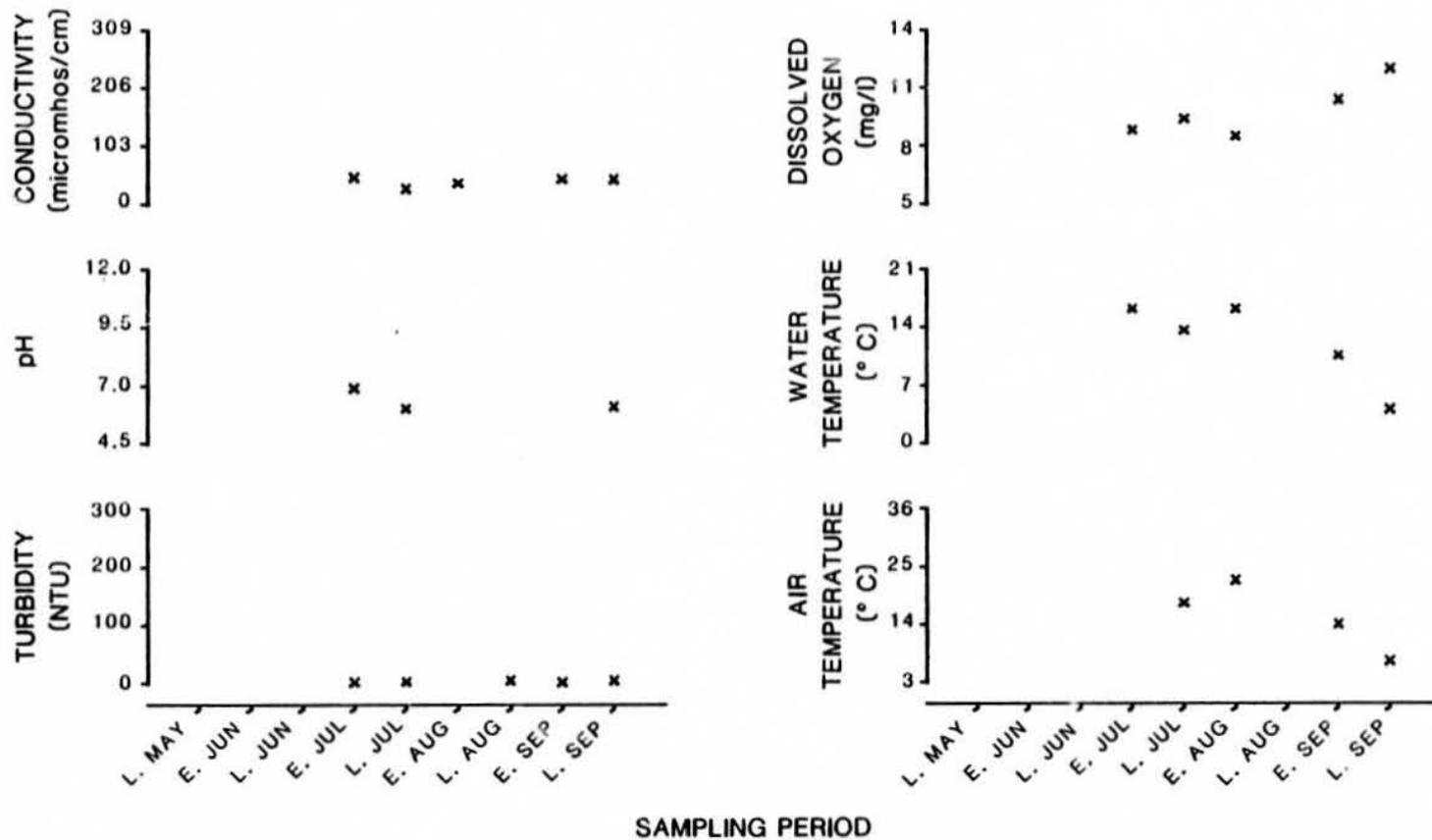
Figure 20. Physiochemical parameters versus time (May-September, 1981) for Deshka River - Site C (R.M. 40.6, Geographic Code 19N06W14BCA)
