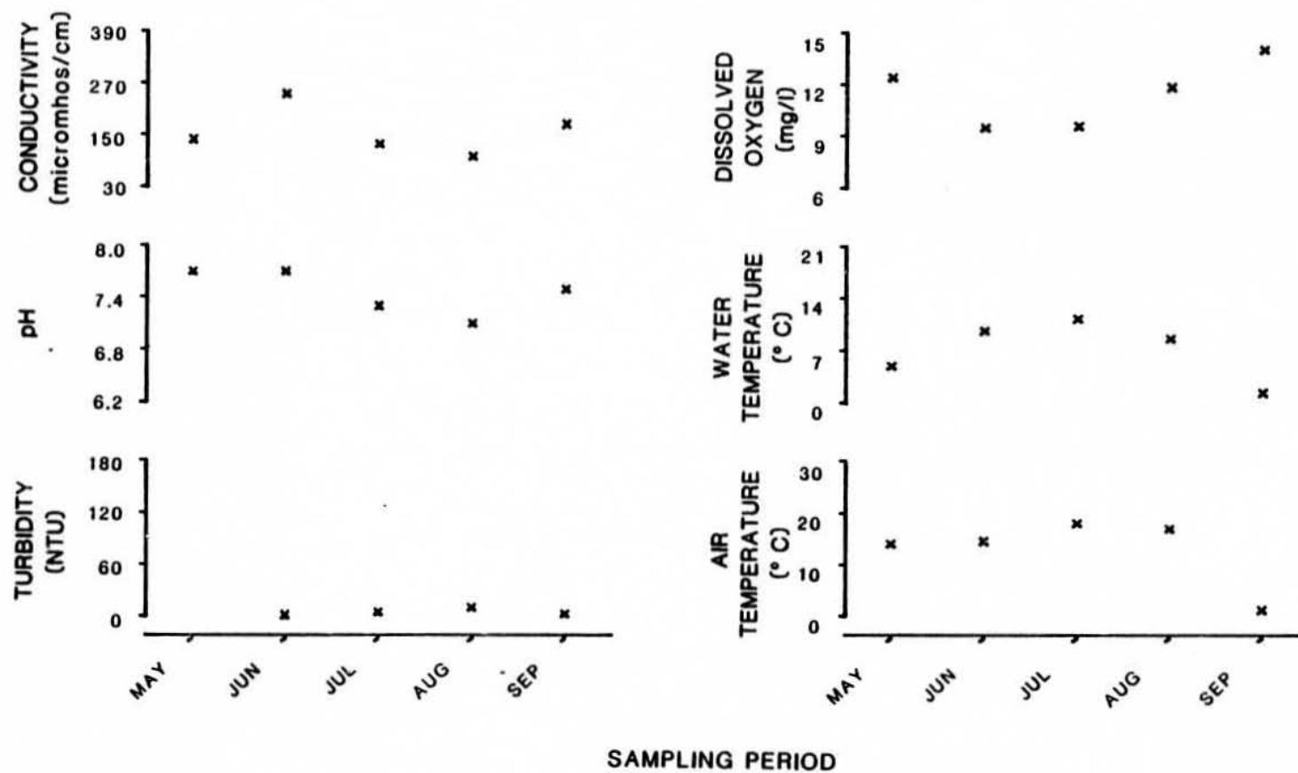
Figure 65. Physiochemical parameters versus time (May-September, 1981)
