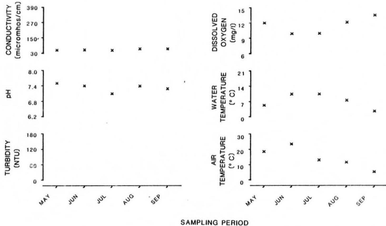
Figure 72. Physiochemical parameters versus time (May-September, 1981)
