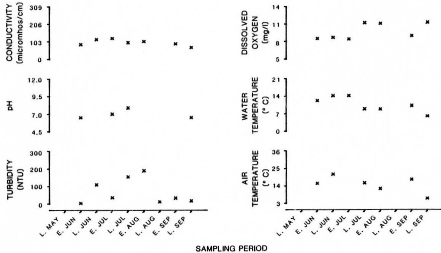
Figure 14. Physiochemical parameters versus time (May-September, 1981)
