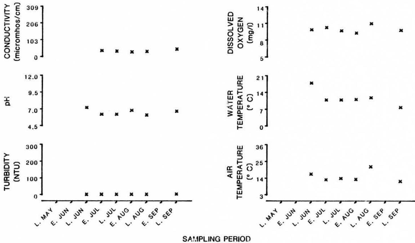
Figure 27. Physiochemical parameters versus time (May-September, 1981)
