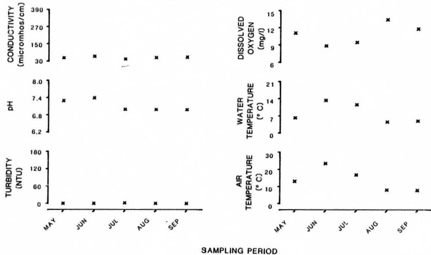
Figure 85. Physiochemical parameters versus time (May-September, 1981)
