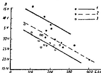
FIGURE 100. Date of ice clearing of the Kuibyshev reservoir,  $D$ , as a function of the sum of temperature rises  $\Sigma \Delta \theta$  during the period from 16 March to 15 April,  $\Sigma \Delta \theta$ , in degrees Celsius.
