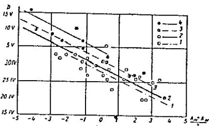
FIGURE 98. Variation in dates of ice clearing on the widened reservoir area at Ul'yanovsk,  $D$ , with the air-temperature anomaly during March and April  $\frac{\Delta H_M + \Delta H_A}{2}$ , for various values of the sum of mean-monthly air temperatures from October to March,  $\Sigma \theta_0$ .
