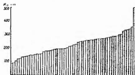
FIGURE 102. Relationship between the formation of an ice jam on the Neiman River downstream from the town of Krasnoyarsk and the maximum water stage at the initial water level point ( $H_u$  in cm above the datum line of the gage of the Krasnoyarsk water gage).
