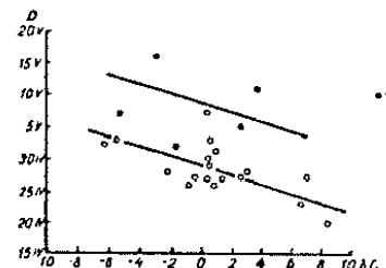
FIGURE 99. Date of ice clearing of the Kuibyshev reservoir,  $D$ , as a function of the change in the relative geopotential gradient from the first to the second half of the winter,  $M_2$ .
