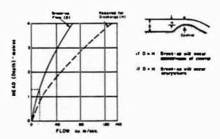
DEPTH AND BREAK-UP FLOW CURVE FOR A 10 METRE WIDTH SECTION
