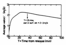
Fig. 6. Computed velocity-time variation at MacEwan Bridge  $(V/V_{\star} = 9)$ .
