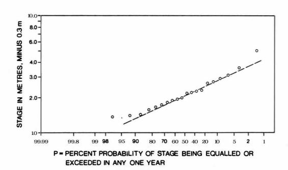
Fig. 8. Frequency curve of breakup peak stage.
