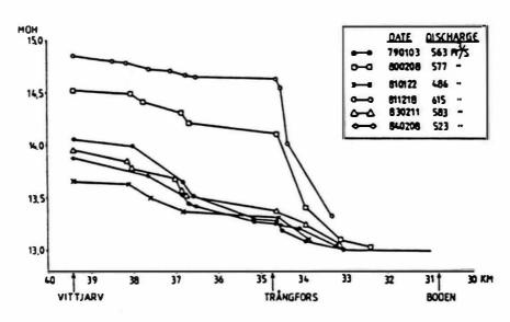
Figure 3. Measured water surface profiles for winters after 1978.
