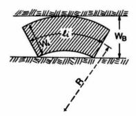
Fig. 4. Illustration of ice sheet movement threshold.
