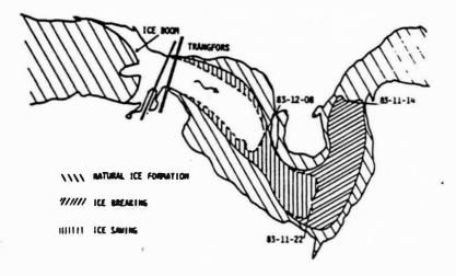
Figure 5. Open water area at Transfors after initial ice cover formation as well as after breaking and sawing of shore ice.
