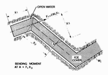
Fig.1. Shulyakovskii's mechanism of transverse crack formation.
