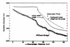
FIG. 5. Downstream variation of peak surge stage as computed with  $V/V_a = 9$ .
