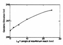
FIG. 8. Effect of jam length on peak surge stage at Mac-Ewan Bridge (computed with  $V/V_{\star} = 9$ ).
