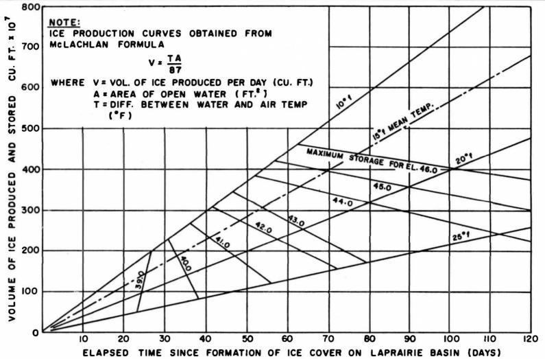
STORAGE CAPACITY OF LAPRAIRIE BASIN AT VARIOUS WATER ELEVATIONS RELATED TO ICE PRODUCTION IN LACHINE RAPIDS.
