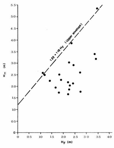
Fig. 6. Maximum stage during breakup versus  $\Pi_{F}$ .
