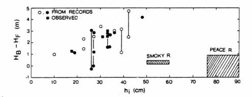
Fig. 8. Effect of ice thickness on  ${\rm H}_B$  -  ${\rm H}_F$ ; data points are for Thames R. at Thamesville; open circles denote estimated  ${\rm h}_1$  's.
