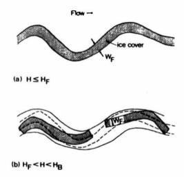
Fig.3. "Loose" arrangement of large ice sheets.
