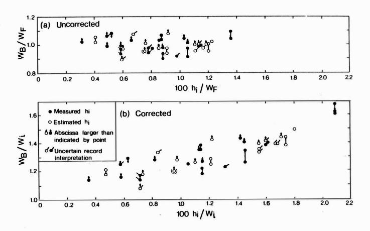
Fig. 16. Effect of side-crack correction; Nashwaak R.
