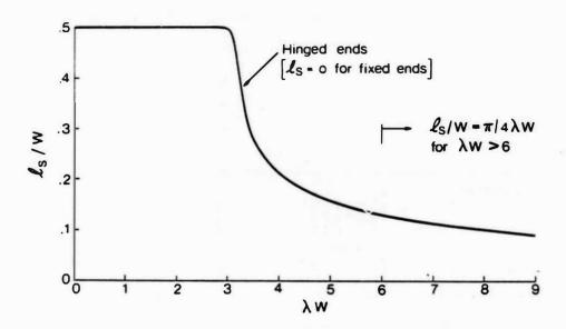
Fig. 13. Location of side cracks.
