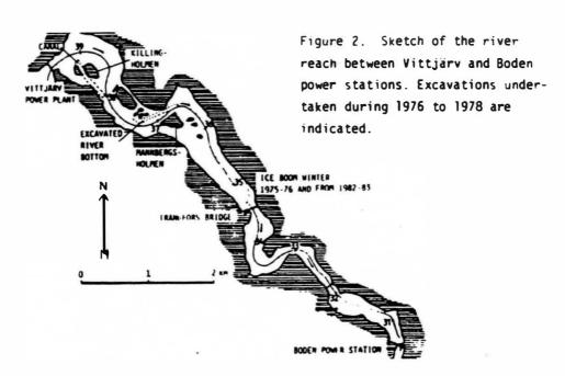
hanging dams and it was necessary to temporarily decrease the flow from 600 m<sup>3</sup>/s to 400 m<sup>3</sup>/s in order to stop further rise of the water level. The water profile dated 811218 on Figure 3 shows the effect of the hanging dam created downstream of Trangfors. The flow reduction lasted for 6 days and the extra cost for alternative power production was estimated to 4 million Swedish Crowns (about 0.5 million dollars).
