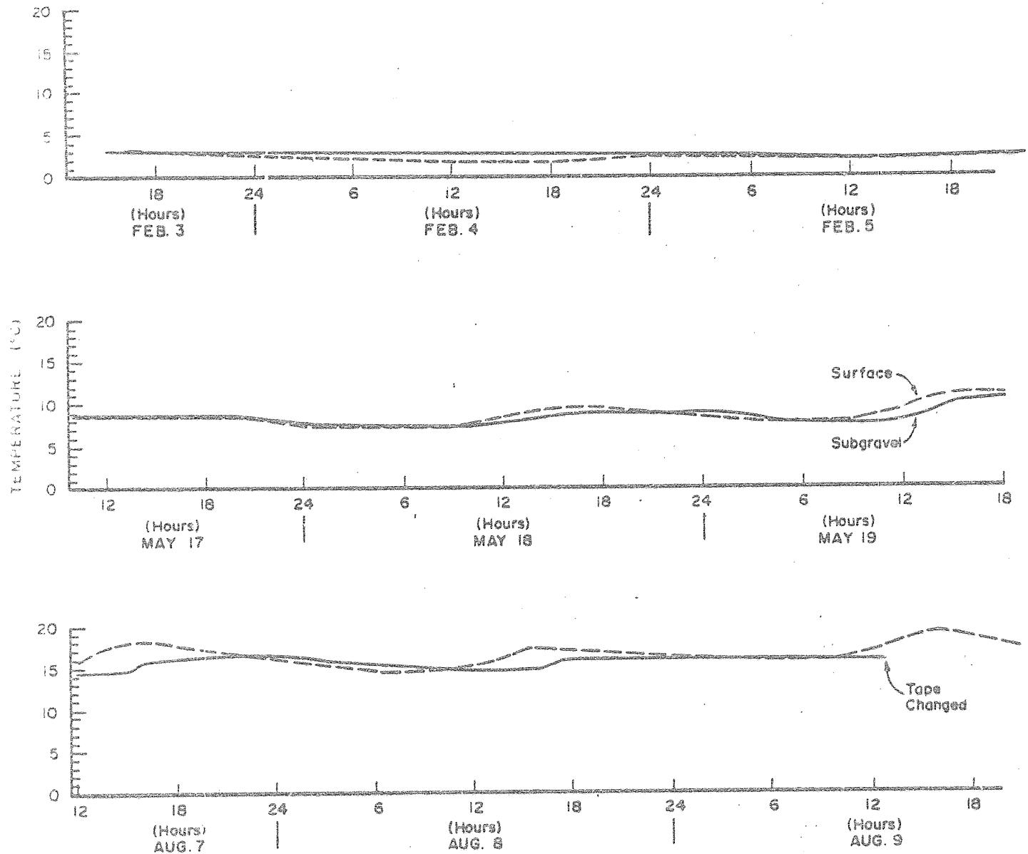
Figure 4. Excerpts from thermograph tapes selected to demonstrate diurnal lag and buffering effects in the subgravel thermal regime of Tom Browne Creek (at the FRB weir) in 1983.
