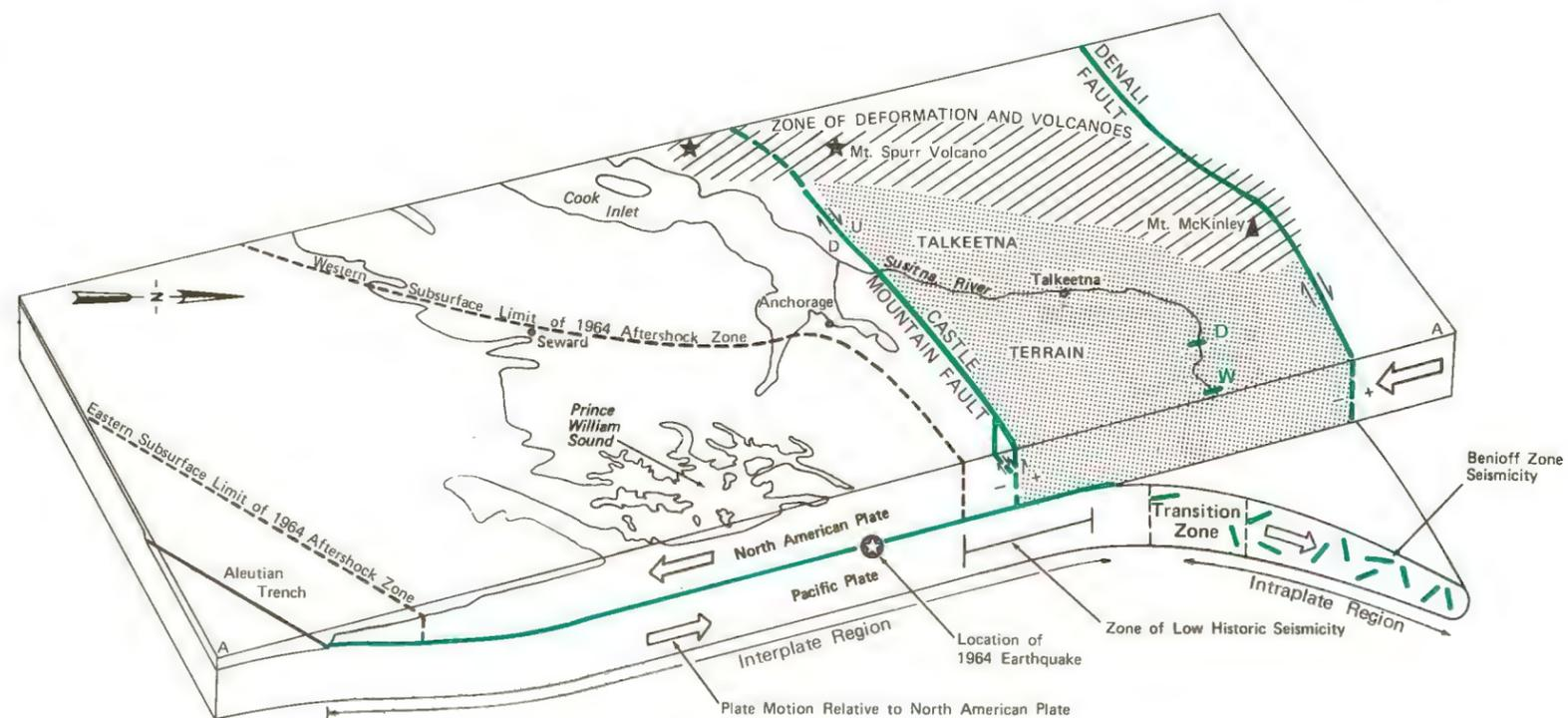
B. THREE DIMENSIONAL VIEW OF SEISMIC SOURCES
