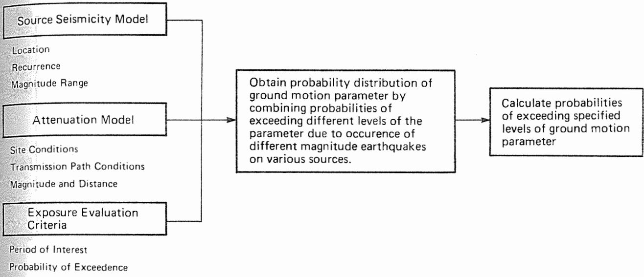
SCHEMATIC REPRESENTATION OF SEISMIC EXPOSURE ANALYSIS APPROACH
