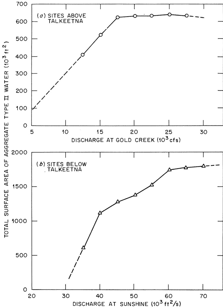
Figure H.3-3. Changes in total wetted surface area in sloughs during filling, Watana, and Watana-Devil Canyon operational flows.
