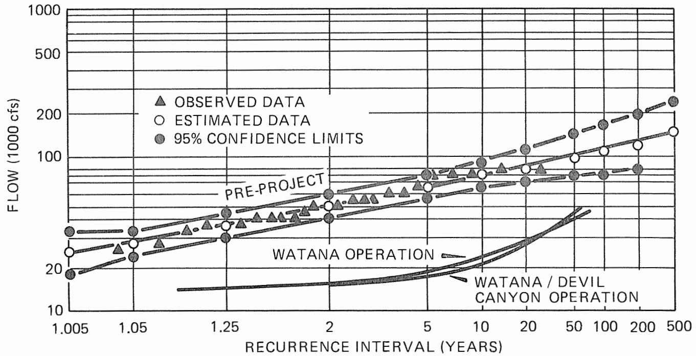
Figure H.2-7. Comparison of recurrence intervals for mean annual floods at Gold Creek under preproject, Watana, and Watana-Devil Canyon operational flow regimes. Source: Exhibit E, Figures E.2.29, E.2.155, and E.2.186.
