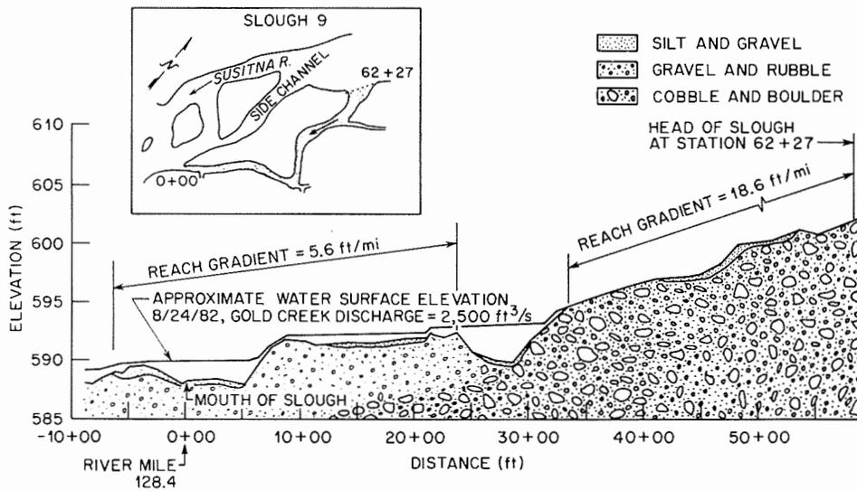
Figure H.1-5. Morphology of a typical side-channel slough.
