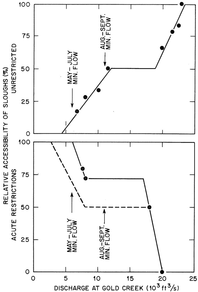
Figure H.3-1. Cumulative response of slough accessibility to mainstem discharge (dashed line in bottom graph assumes a acute accessibility threshold at Sloughs 6A and 11 at 5,000 cfs).
