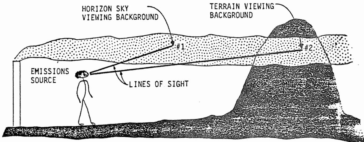
Figure G-9. Two Types of Plume Visibility Impairment Considered in the Level-1 Visibility Screening Analysis. [Source: Latimer and Ireson, 1980]
