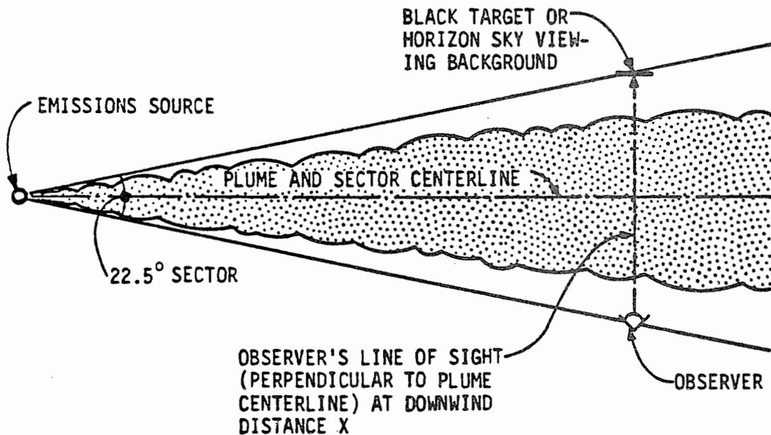
Figure G-10. Geometry of Plume, Observer, and Line of Sight Used in Level-1 Visibility Screening Analysis. [Source: Latimer and Ireson, 1980]
