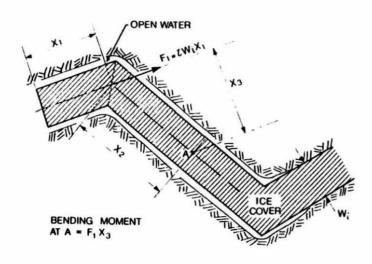
Fig.1. Shulyakovskii's mechanism of transverse crack formation.
