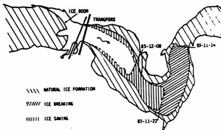
Figure 5. Open water area at Trångfors after initial ice cover formation as well as after breaking and sawing of shore ice.
