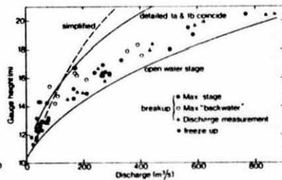
FIG. 11.—Freeze Up and Breakup Stages versus Discharges; Thames River at Thamesville ( $W = 40-65$  m,  $S = 0.00023$ )
