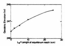
FIG. 8. Effect of jam length on peak surge stage at Mac-Ewan Bridge (computed with  $V/V_{\star} = 9$ ).
