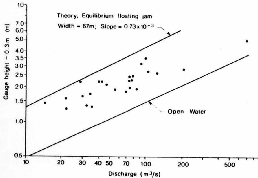
Fig. 5. Effect of discharge on breakup stage.
