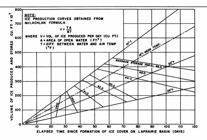
MAXIMUM STORAGE CAPACITY OF LAPRAIRIE BASIN AT VARIOUS WATER ELEVATIONS RELATED TO ICE PRODUCTION IN LACHINE RAPIDS.
