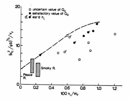
Fig. 10 Dimensionless "ice-clearing" discharge versus dimensionless ice thickness.
