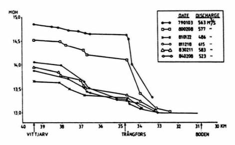
Figure 3. Measured water surface profiles for winters after 1978.
