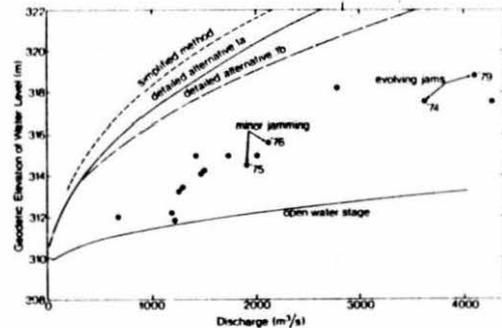
FIG. 9.—Peak Breakup Stage versus Discharge; Peace River at Peace River ( $W = 600$  m,  $S = 0.00035$ )
