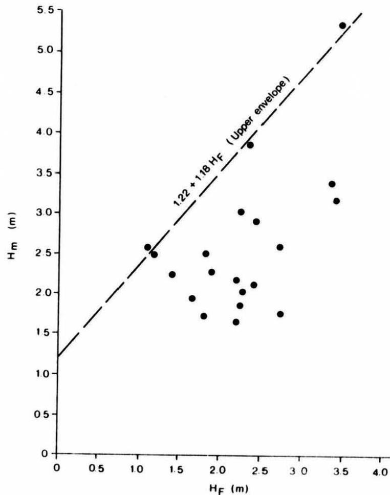
Fig. 6. Maximum stage during breakup versus  $H_F$ .
