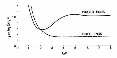
Fig. 14. Dimensionless uplift pressure head required to cause side cracking.
