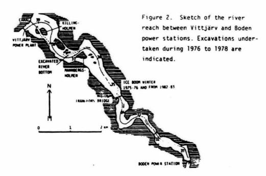
hanging dams and it was necessary to temporarily decrease the flow from 600 m<sup>3</sup>/s to 40G m<sup>3</sup>/s in order to stop further rise of the water level. The water profile dated 811218 on Figure 3 shows the effect of the hanging dam created downstream of Transfors. The flow reduction lasted for 6 days and the extra cost for alternative power production was estimated to 4 million Swedish Crowns (about 0.5 million dollars).
