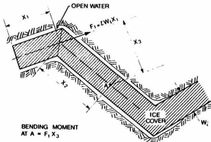
Fig. 1. Shulyakovskii's mechanism of transverse crack formation.
