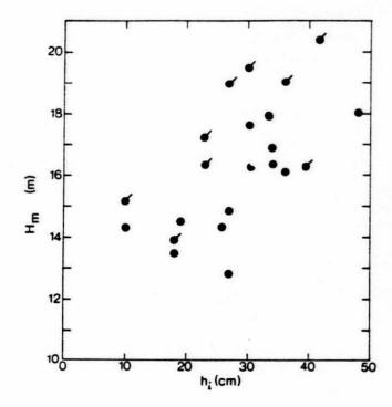
Fig. 7. Effect of ice thickness on maximum breakup stage, Thames R. at Thamesville, Ontario. (H<sub>m</sub> = water surface elevation above an arbitrary datum. Data points with strokes indicate that ice thickness was estimated - error up to 30%).
