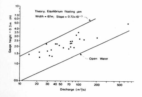
Fig. 5. Effect of discharge on breakup stage.
