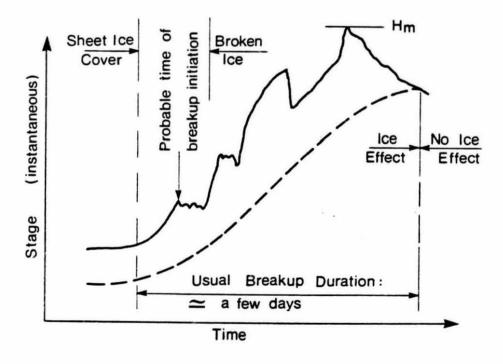
Fig. 6 Schematic illustration of instantaneous stage variation with time during breakup.
