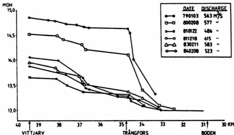
Figure 3. Measured water surface profiles for winters after 1978.
