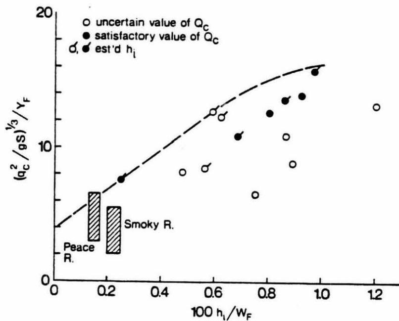
Fig. 10 Dimensionless "ice-clearing" discharge versus dimensionless ice thickness.
