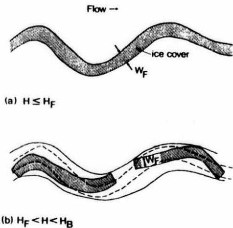
Fig.3. "Loose" arrangement of large ice sheets.
