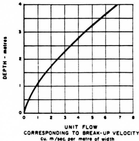
DEPTH AND BREAK-UP FLOW CURVE
