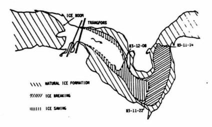
Figure 5. Open water area at Trangfors after initial ice cover formation as well as after breaking and sawing of shore ice.
