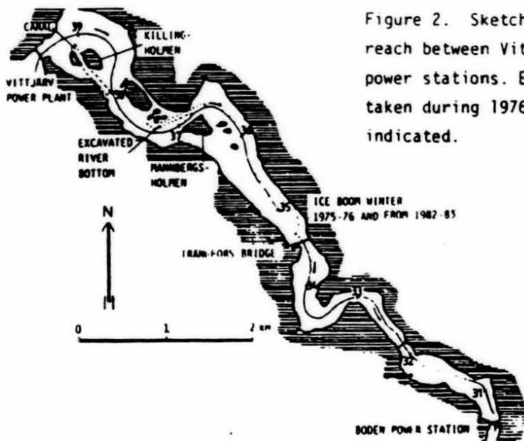
Figure 2. Sketch of the river reach between Vittjärva and Boden power stations. Excavations undertaken during 1976 to 1978 are indicated.
