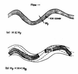
Fig.3. "Loose" arrangement of large ice sheets.
