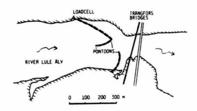
Figure 4. Ice boom at Trangfors with a central gap that can be closed.
