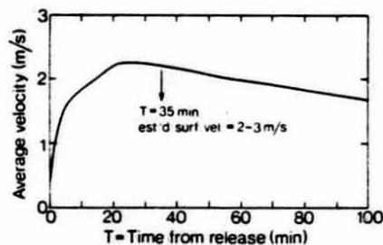
FIG. 6. Computed velocity-time variation at MacEwan Bridge ( $V/V_* = 9$ ).
