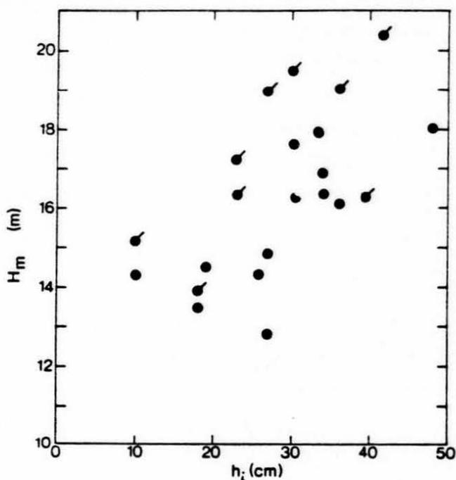
Fig. 7. Effect of ice thickness on maximum breakup stage, Thames R. at Thamesville, Ontario. ( $H_m$  = water surface elevation above an arbitrary datum. Data points with strokes indicate that ice thickness was estimated - error up to 30%).
