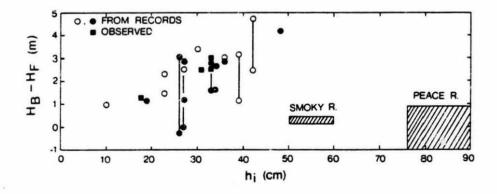
Fig. 8. Effect of ice thickness on H<sub>B</sub> - H<sub>F</sub>; data points are for Thames R. at Thamesville; open circles denote estimated h<sub>i</sub>'s.
