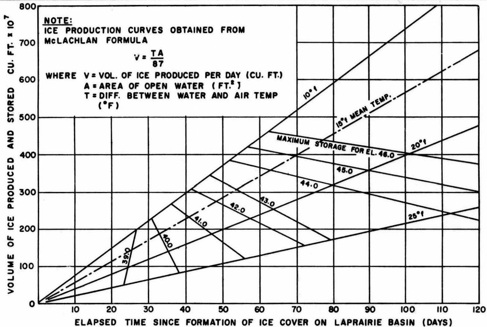
MAXIMUM STORAGE CAPACITY OF LAPRAIRIE BASIN AT VARIOUS WATER ELEVATIONS
