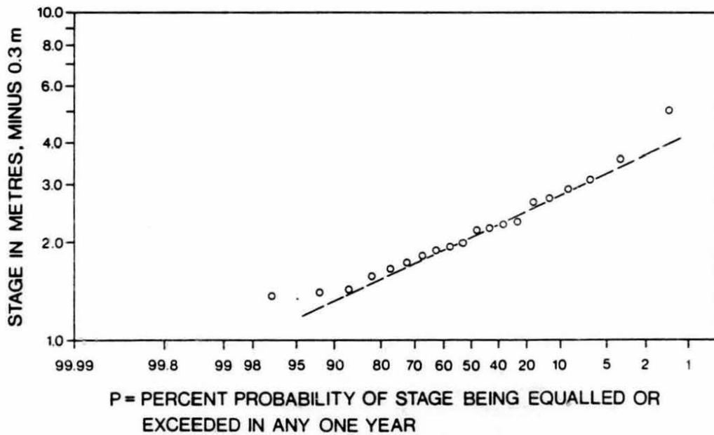
Fig. 8. Frequency curve of breakup peak stage.
