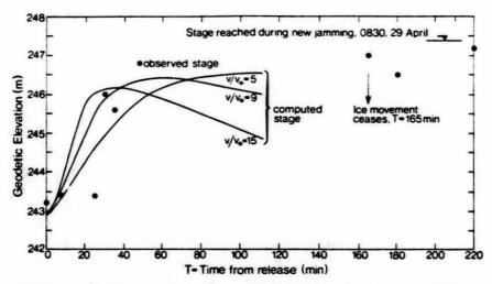
Fig. 4. Computed versus observed stage-time variations at MacEwan Bridge (T = 0 is taken at 1950 h, April 28, 1979; observed stages are approximate).
