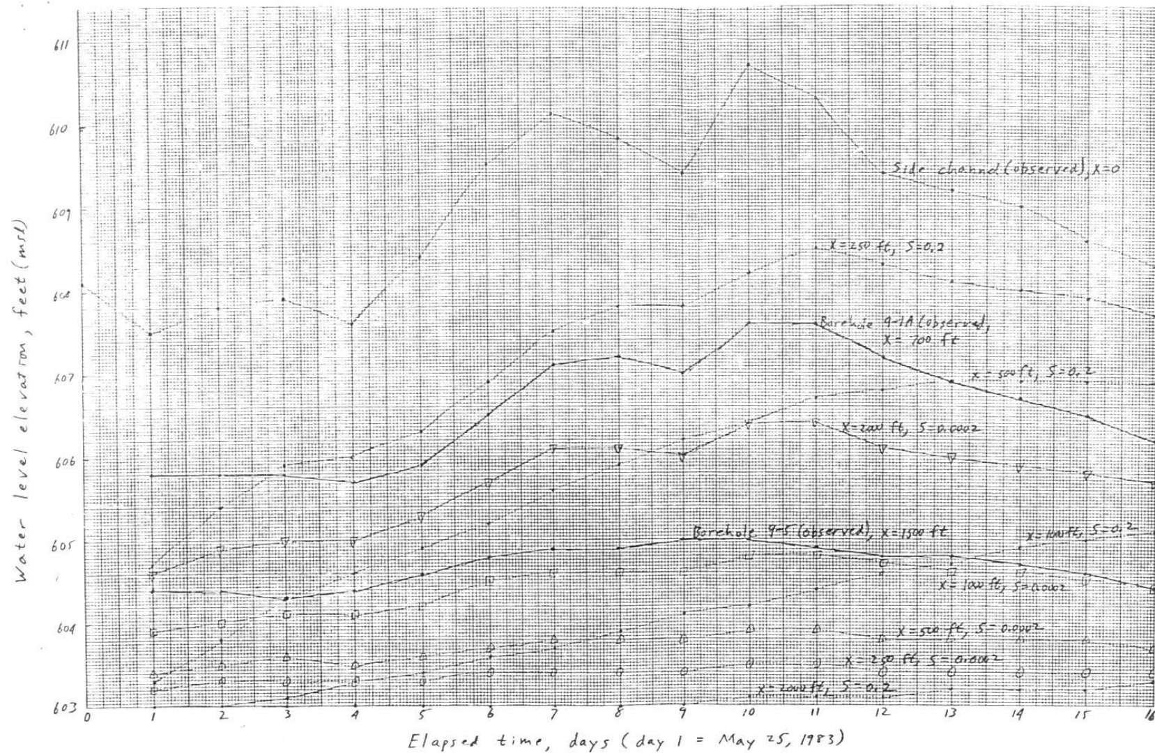
Figure 14. Simulated Groundwater Level Variations in Response to River Stage Variations
