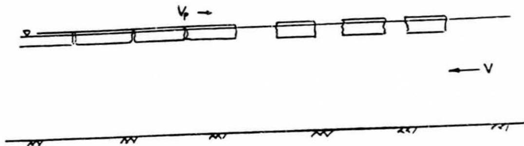
2. Progression, but the arriving floes thicken to values greater than the initial thickness of the arriving ice,  $t_j/H < 0.33$ , or  $t_j/H > .33$ .
