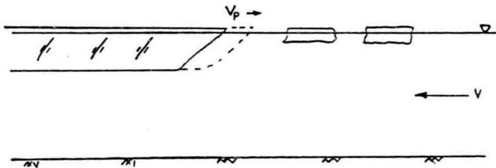
3. Progression with ice cover thickening and ice also being transported beneath the cover.
