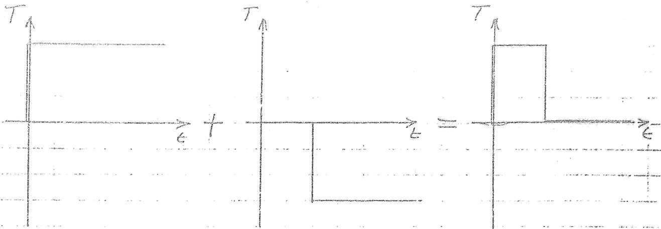
SUM OF EQUALLY SPACED PULSES = SQUARE WAVE
