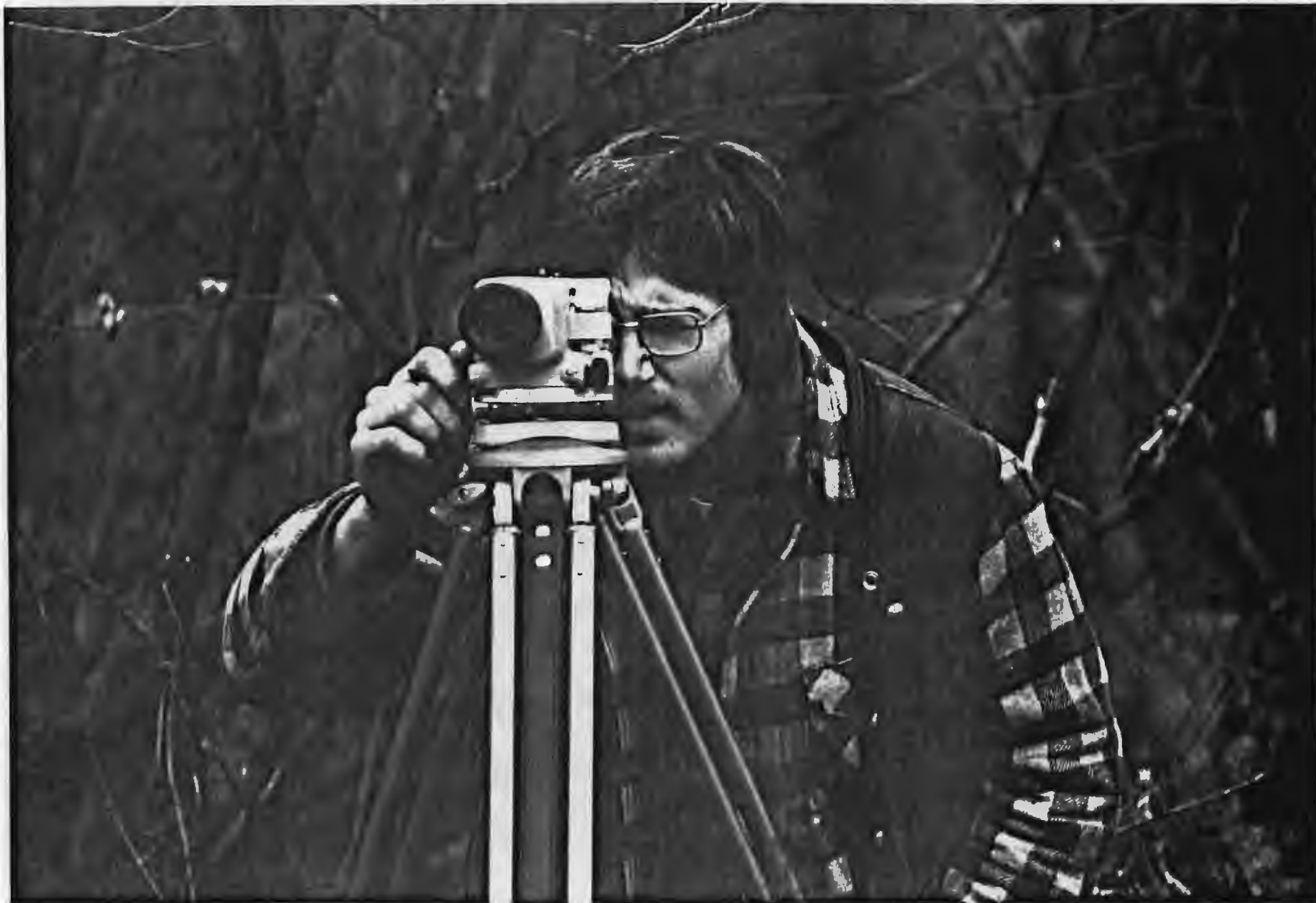
Plate 8. Use of a Leitz B-2 survey level for surveying in the selected habitat study sloughs.
