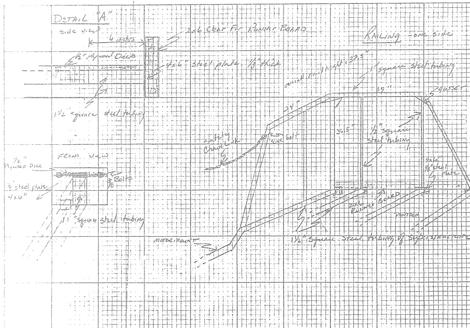
Appendix Figure 3-F-2. Side view of the points of attachment for the pontoon floats and the safety railing on the downstream migrant trap, 1982.
