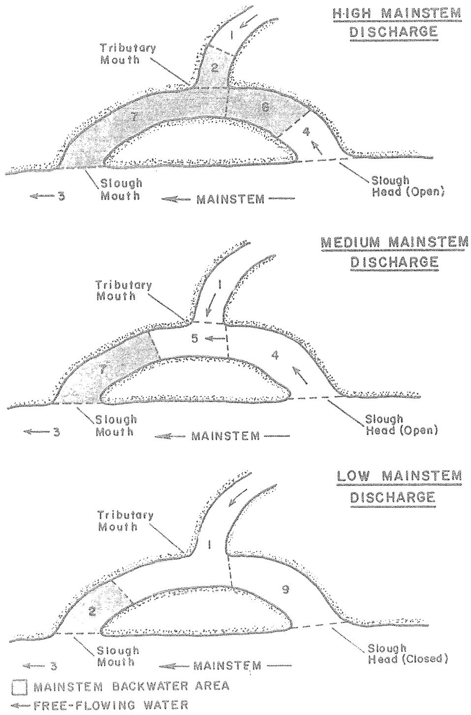
Figure 3-2-3. Hypothetical slough with associated tributary showing hydraulic zones present at three mainstem discharges.
