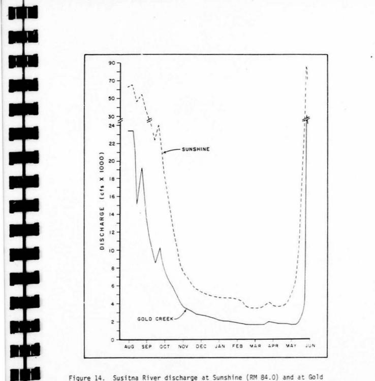
Figure 14. Susitna River discharge at Sunshine (RM 84.0) and at Gold Creek (RM 136.7), August 1984 to June 1985. All measurements are provisional data provided by USGS.
