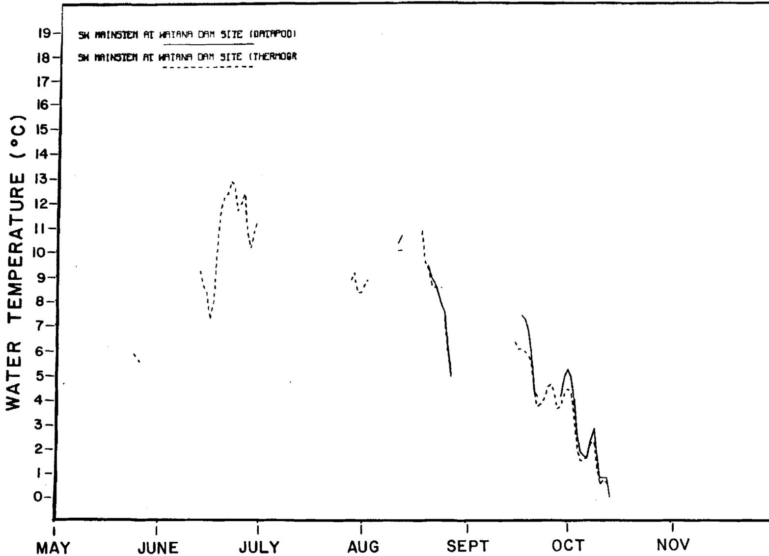
Figure 16. Mean daily surface water temperature recorded at Mainstem Susitna River at Watana Dam Site (RM 184.2) during the 1984 open water season.
