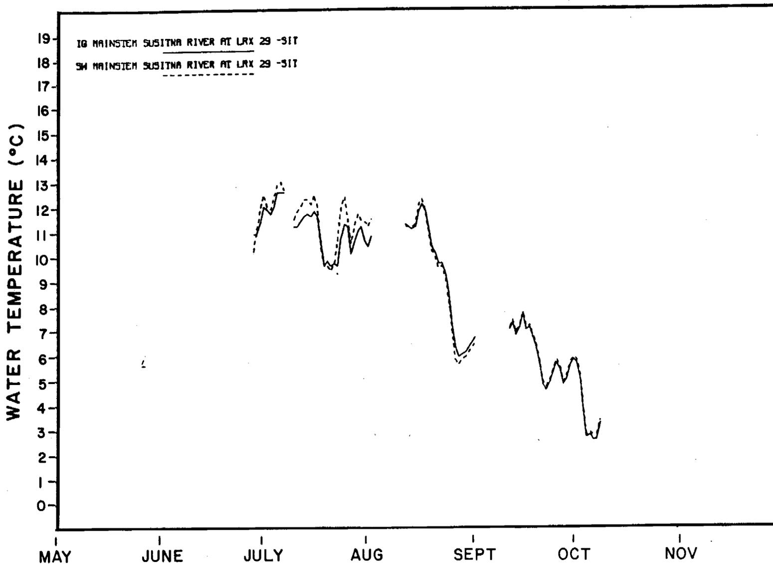
Figure 11. Mean daily surface and intragravel water temperatures recorded at Mainstem Susitna River at LRX 29 (RM 125.9) during the 1984 open water season.
