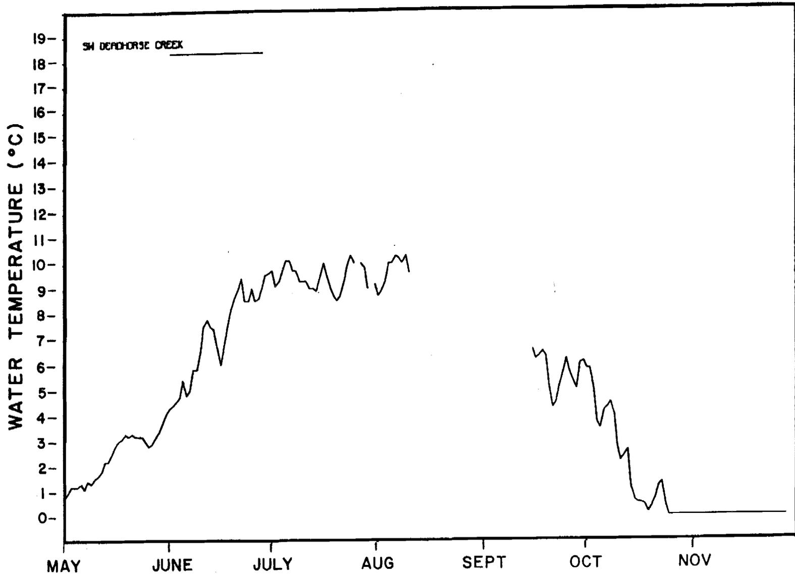
Figure 25. Mean daily surface water temperature recorded at Deadhorse Creek (RM 120.9, TRM 1.0) during the 1984 open water season.
