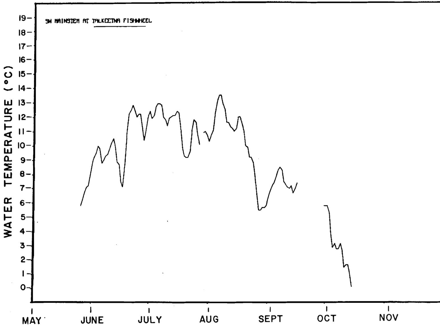
Figure 8. Mean daily surface water temperature recorded at Mainstem Susitna River at Talkeetna Fishwheel Camp (RM 103.0) during the 1984 open water season.
