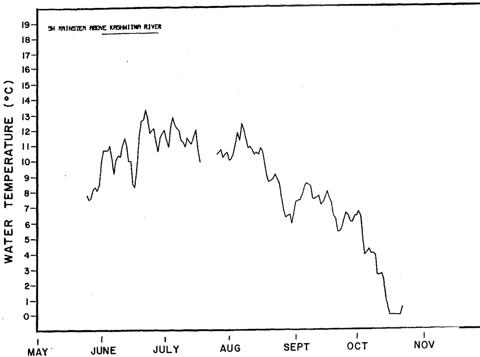
Figure 5. Mean daily surface water temperature recorded at Mainstem Susitna River above the Kashwitna River (RM 61.2) during the 1984 open water season.
