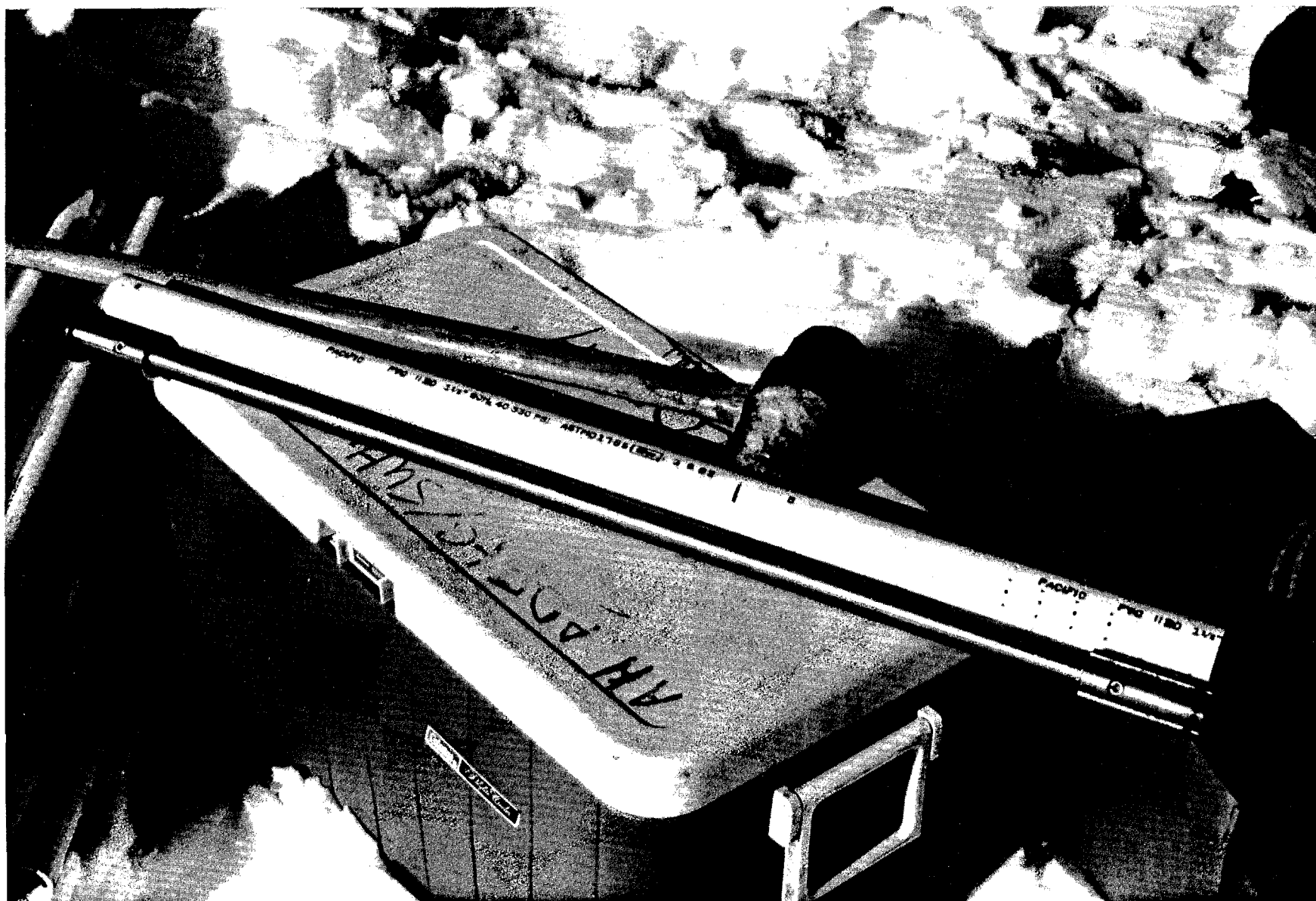
Plate 3-2. Standpipe (with 48 one-eighth inch holes) used for monitoring intragravel water quality and driver used for installation.
