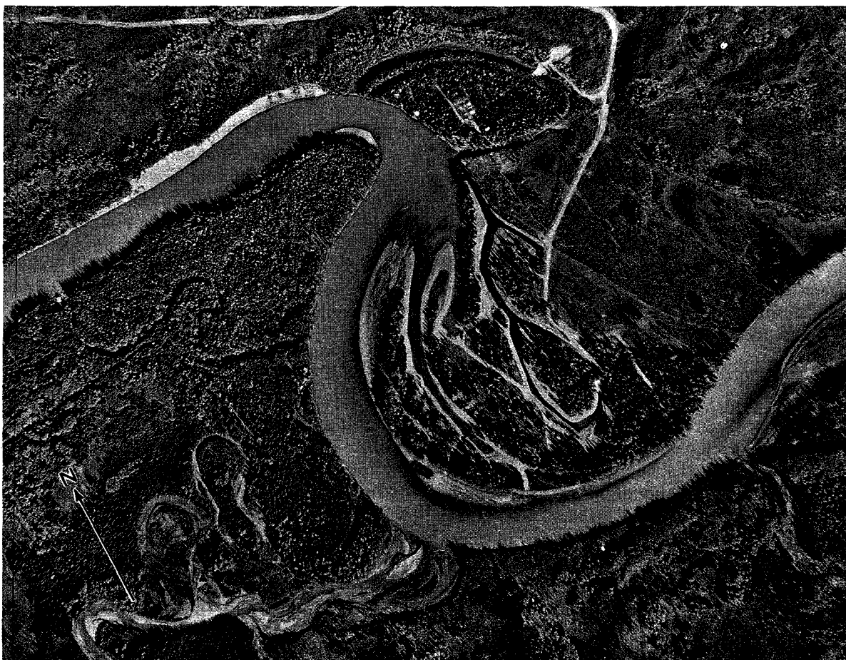
FIGURE 19.—Kenai River between approximate river miles 44.8 and 42.9. Interior of meander loop has been developed with canals. Note natural channels across neck of meander; one channel has been partly excavated to form a canal. The Killey River enters from bottom of photograph. Flow direction is from right to left. Scale, 1:12,000, or 1 in. = 1,000 ft. Date: September 24, 1972. Photograph credit: U.S. Army Corps of Engineers.
