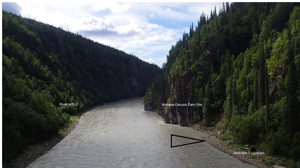
Photo G-4. Aerial view of Site 2 of the sonar feasibility study, July, 2013. Direction of river flow is from bottom to top of the photo. A conceptual depiction of ARIS sonar sampling area is shown with black triangle; actual sample volume is an expanding trapezoid with the longest axis in the upstream-downstream direction. River discharge at the time the photograph was taken was 21,313 cfs at the Tsusena Creek gage.
