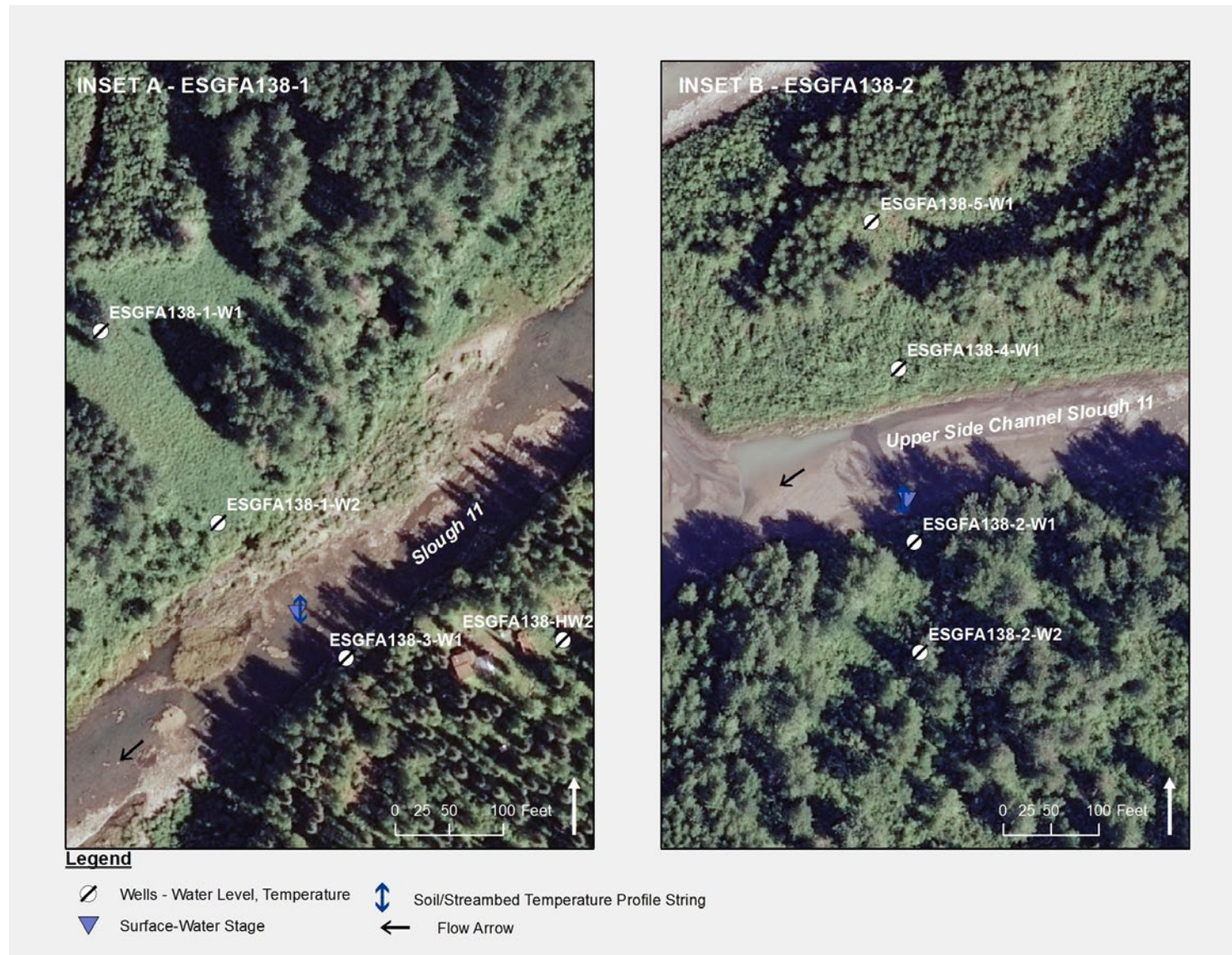
Figure 4.5-13. Inset A (left) and B (right) show locations of aquatic transect stations with continuously measured parameters at FA-138 (Gold Creek) Focus Area. These study sections are intended to improve the understanding of GW/SW interaction processes relevant to aquatic habitat evaluations.
