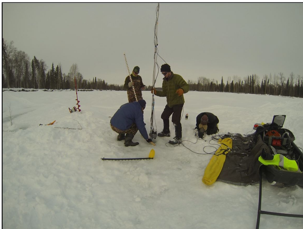
Figure 3-7. Lowering camera equipment through hole in ice at ESS40.
