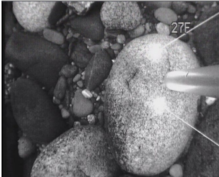
Figure 3-8. AquaVu image from ESS40 using lasers and both the AquaVu integrated lights and Princeton Tec scuba flashlights. (Note: The temperature sensor was not calibrated and values are erroneous.)
