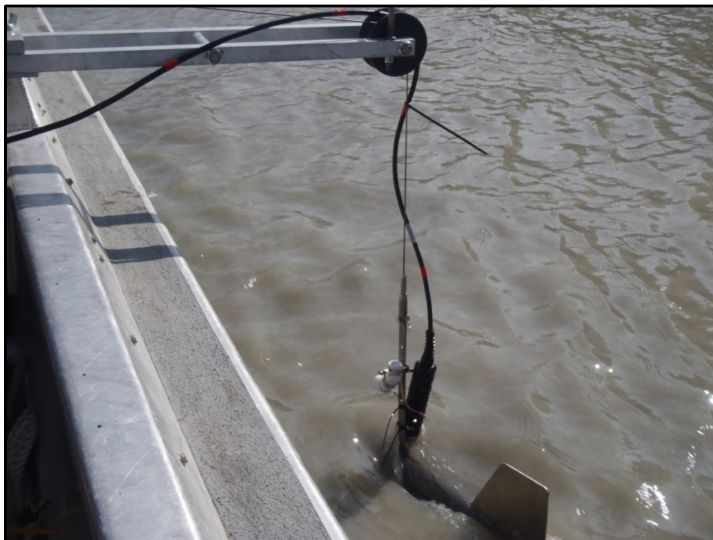
Photo I-3. Deploying water quality probe. Probe is attached to a 60 lb. lead fish.
