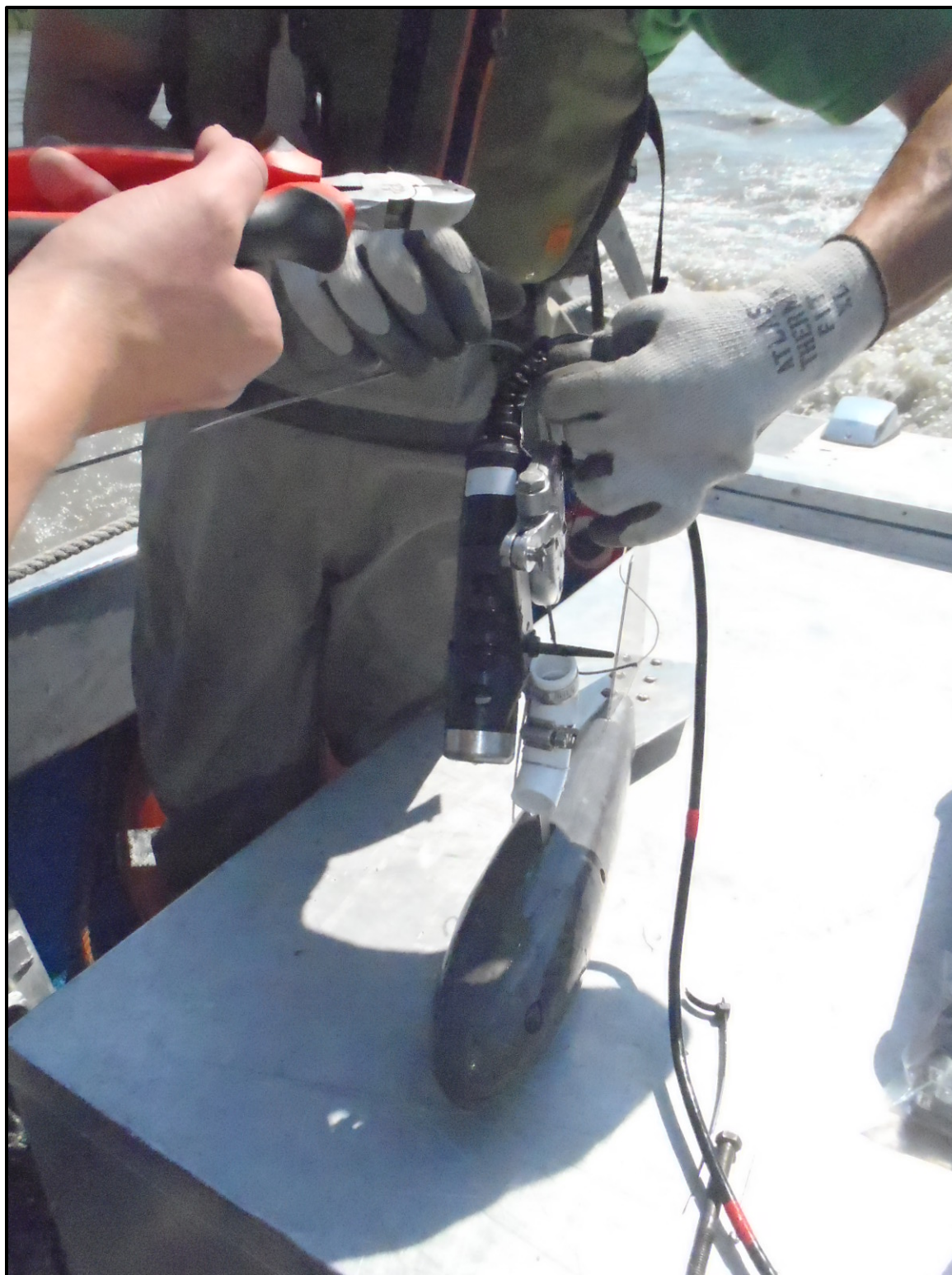
Photo I-1. Preparing water quality parameter probe for deployment from boat.
