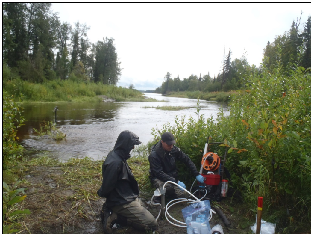
Photo I-10. Collecting water sample from Focus Area well.
