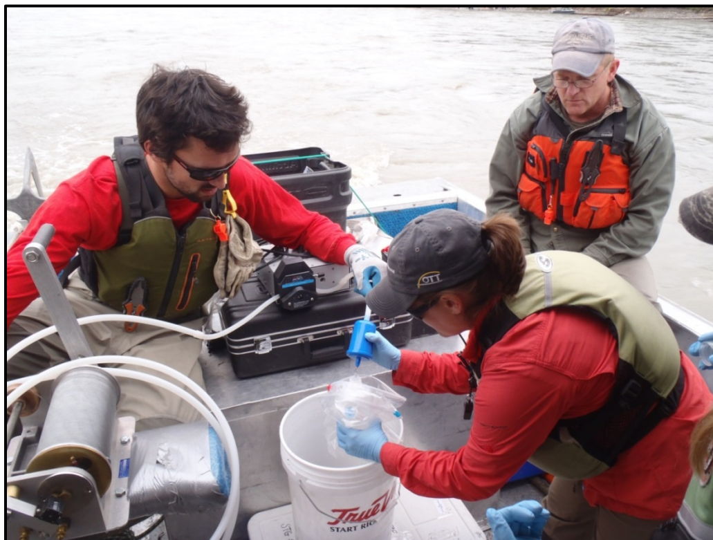
Photo I-6. Collection of filtered water quality sample.
