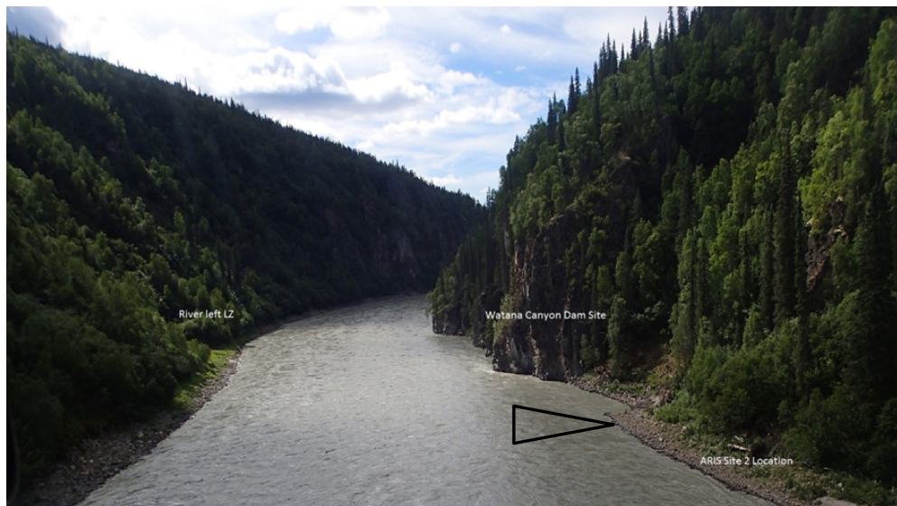
Photo G-4. Aerial view of Site 2 of the sonar feasibility study, July, 2013. Direction of river flow is from bottom to top of the photo. A conceptual depiction of ARIS sonar sampling area is shown with black triangle; actual sample volume is an expanding trapezoid with the longest axis in the upstream-downstream direction. River discharge at the time the photograph was taken was 21,313 cfs at the Tsusena Creek gage.
