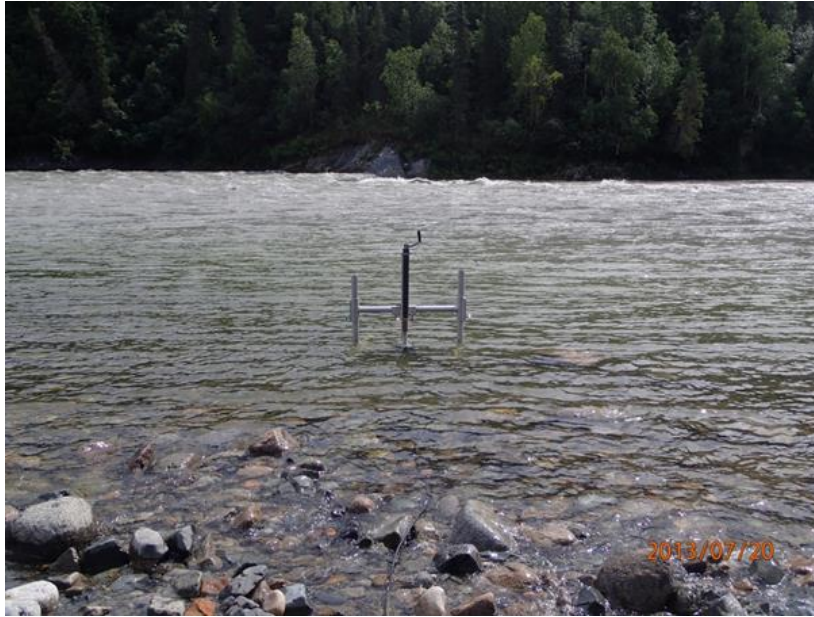
Photo G-1. Aluminum H-mount frame used to deploy the ARIS 1200 sonar at Site 1 during the Watana Canyon sonar feasibility study, July, 2013.
