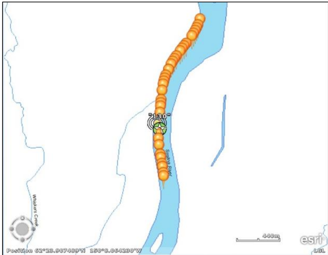
Figure C.A2-12. Detections for radio tag 151.934 Code 45 during Pass 2. The yellow circle indicates the location of the tag and the star is the location of the highest power detection. The power of the detection is located above the star and is on a scale from 40 to 154.
