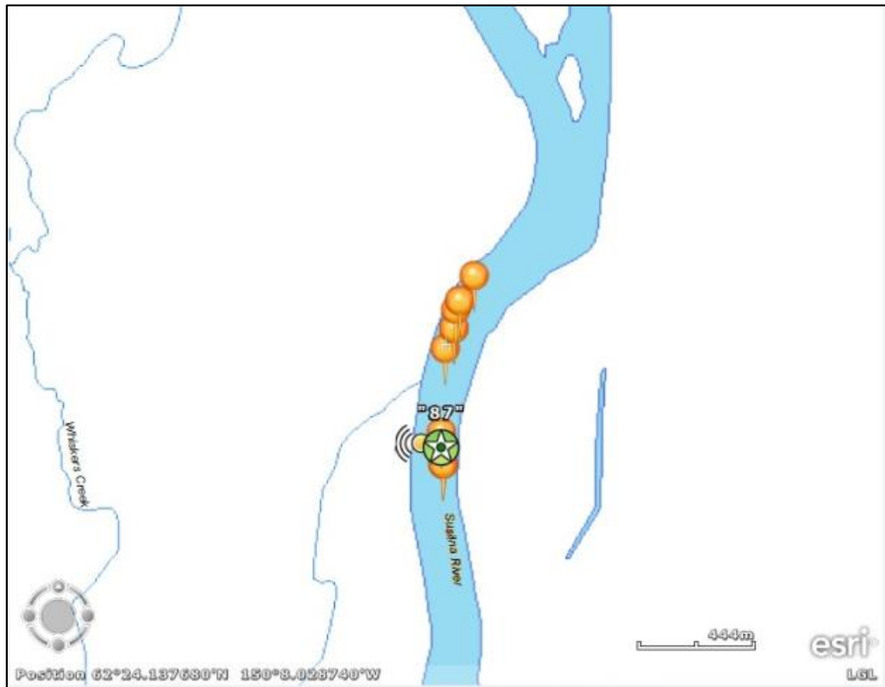
Figure C.A2-13. Detections for radio tag 151.934 Code 68 during Pass 1. The yellow circle indicates the location of the tag and the star is the location of the highest power detection. The power of the detection is located above the star and is on a scale from 40 to 154.
