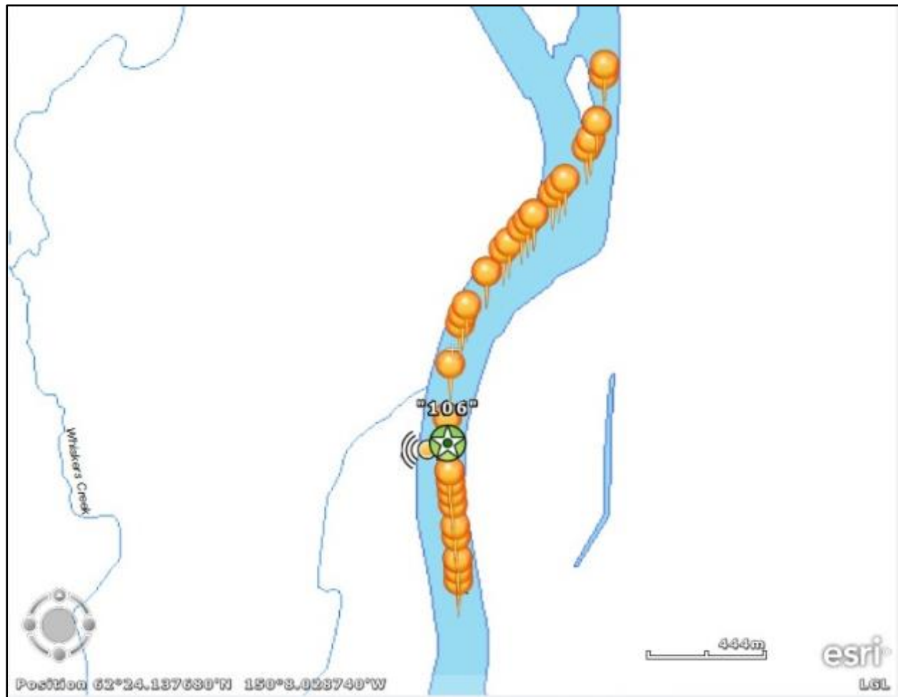
Figure C.A2-9. Detections for radio tag 151.934 Code 94 during Pass 1. The yellow circle indicates the location of the tag and the star is the location of the highest power detection. The power of the detection is located above the star and is on a scale from 40 to 154.
