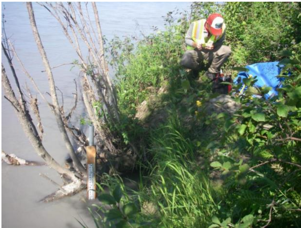
Figure 2. Example stilling well and staff gage setup.
