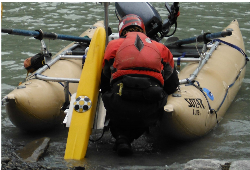
Figure 3. M9 trimaran mount, inverted to show transducer head.
