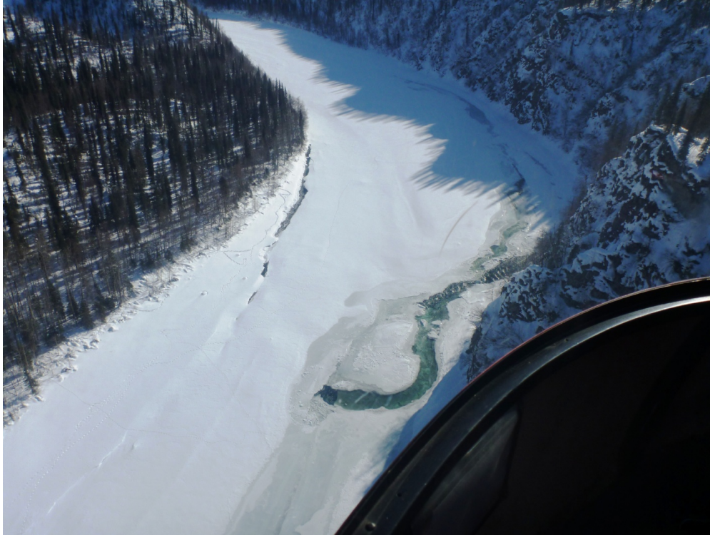
Figure 3.2-1. PRM 149.4 (RM146) - Thermal lead on river right and a velocity lead on river left near Susitna. Note that flow is from top to bottom in this photo and river right and river left are with respect to flow. March 22nd, 2012.
