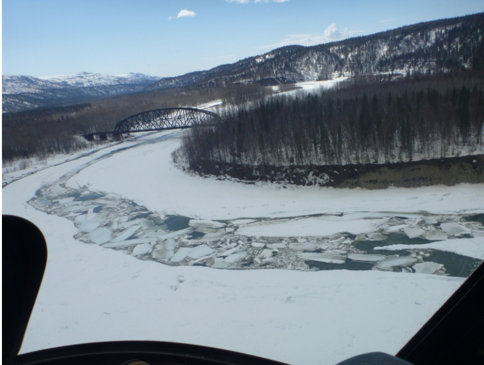
Figure 1.1-7. PRM 140.4 (RM 137)- A small jam in a middle river velocity lead. Flow is from right to left in this photo. April 19, 2012.
