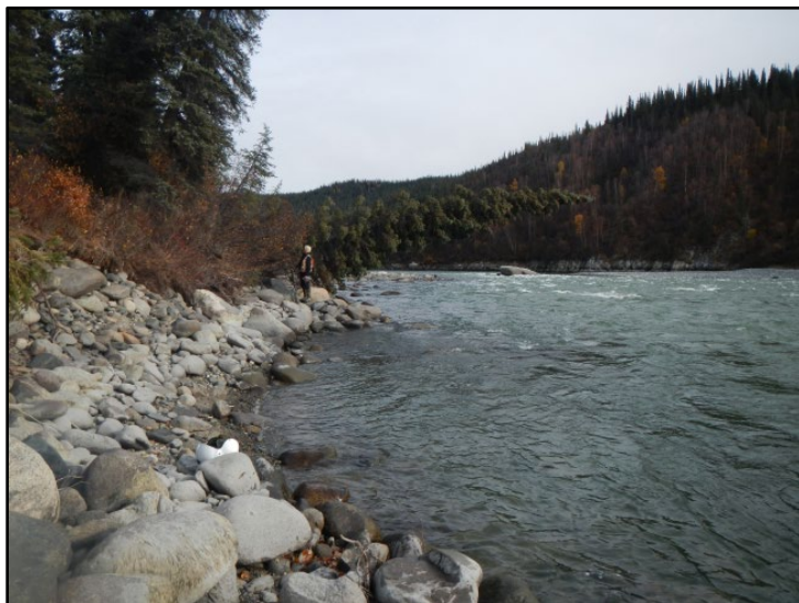
Figure 5.3-1. October 3, 2013 flow conditions at the high pool elevation for the proposed reservoir operations, looking downstream at the left bank. The white helicopter helmet on the bank is marking the approximate high pool elevation line.
