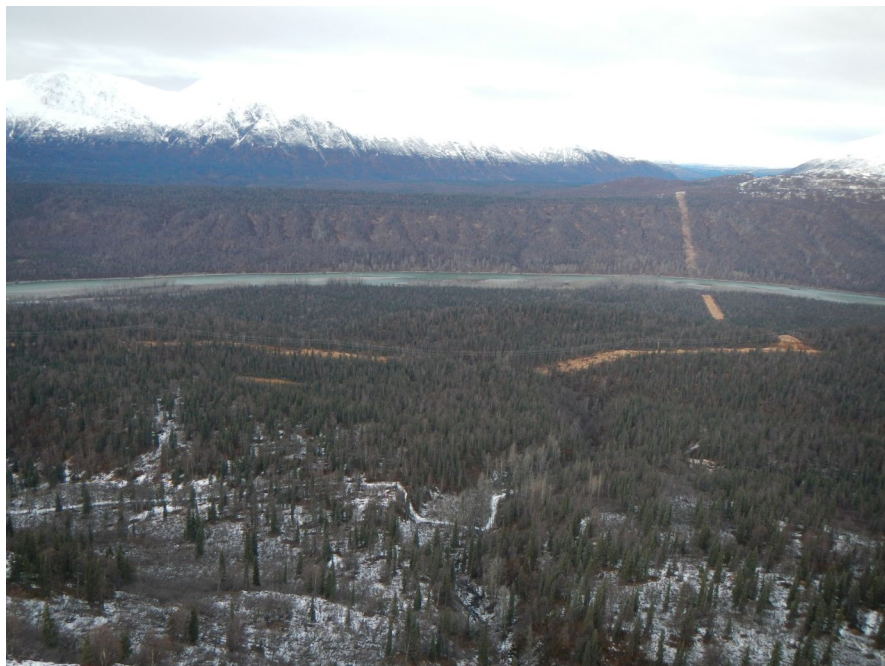
Figure 5.2-1. October 31, 2013 aerial observations of the groundwater recharge zone for FA-144 (Slough 21), which is just downstream of the power line cut visible on the right-hand side of the image. The watershed areas upgradient of the Slough 11 serve as a collection area for snowmelt and rainfall, which partially contributes to the groundwater recharge in the slough.
