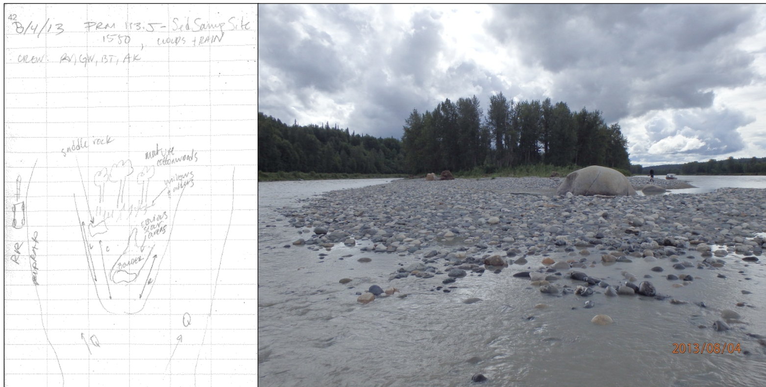
Figure 4.1-1. Sketch of transect locations (identified as L, C and R) for surface sampling at sample location PRM 113.5 (left) and photograph of sample location, view downstream (right).
