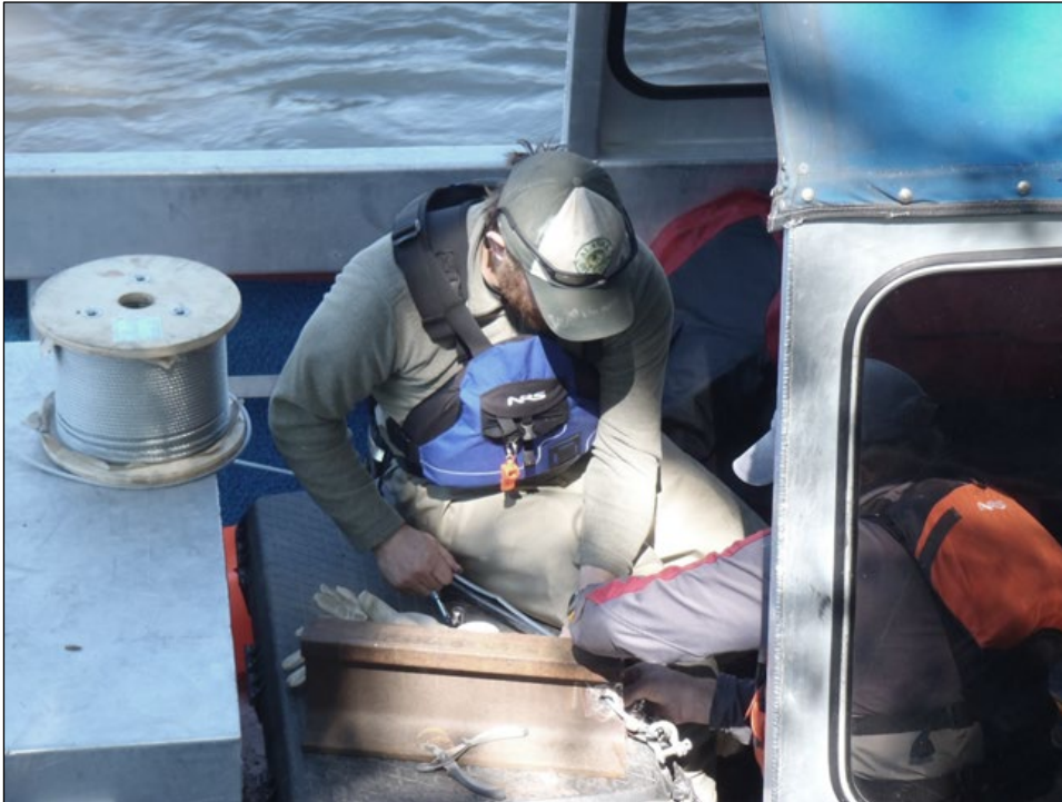
Photo A-25c. Attaching thermistor string to buoy system anchor
