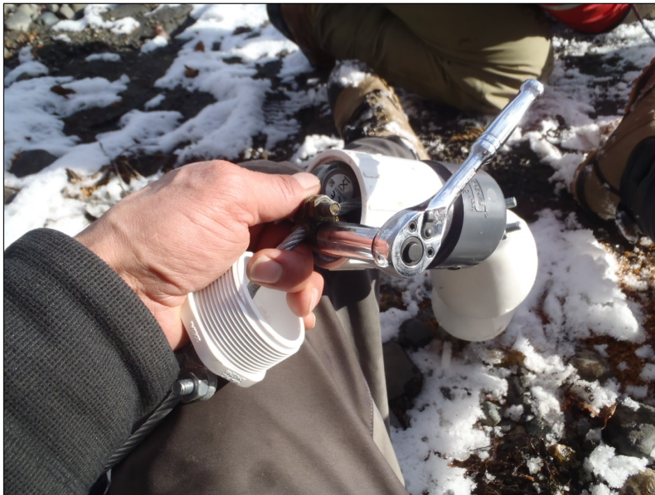
Photo A-30c. Installing thermistor in overwinter system.
