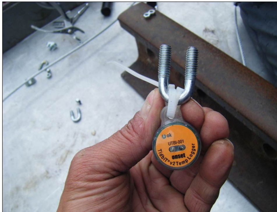
Photo A-3c. Onset® Tidbit water temperature data logger
