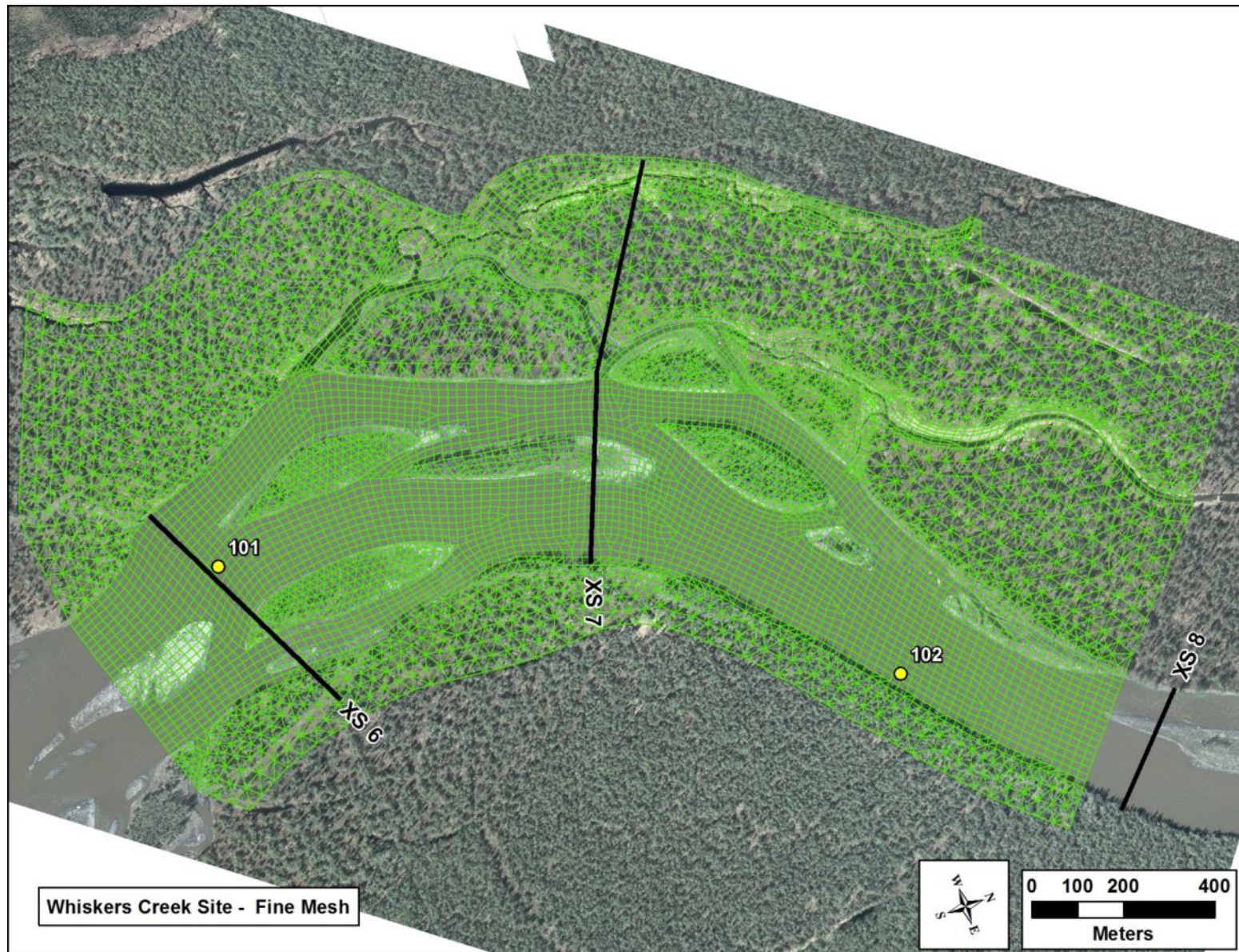
Figure 4-24. Example of Fine Mesh Applied in Whiskers Slough Focus Area.
