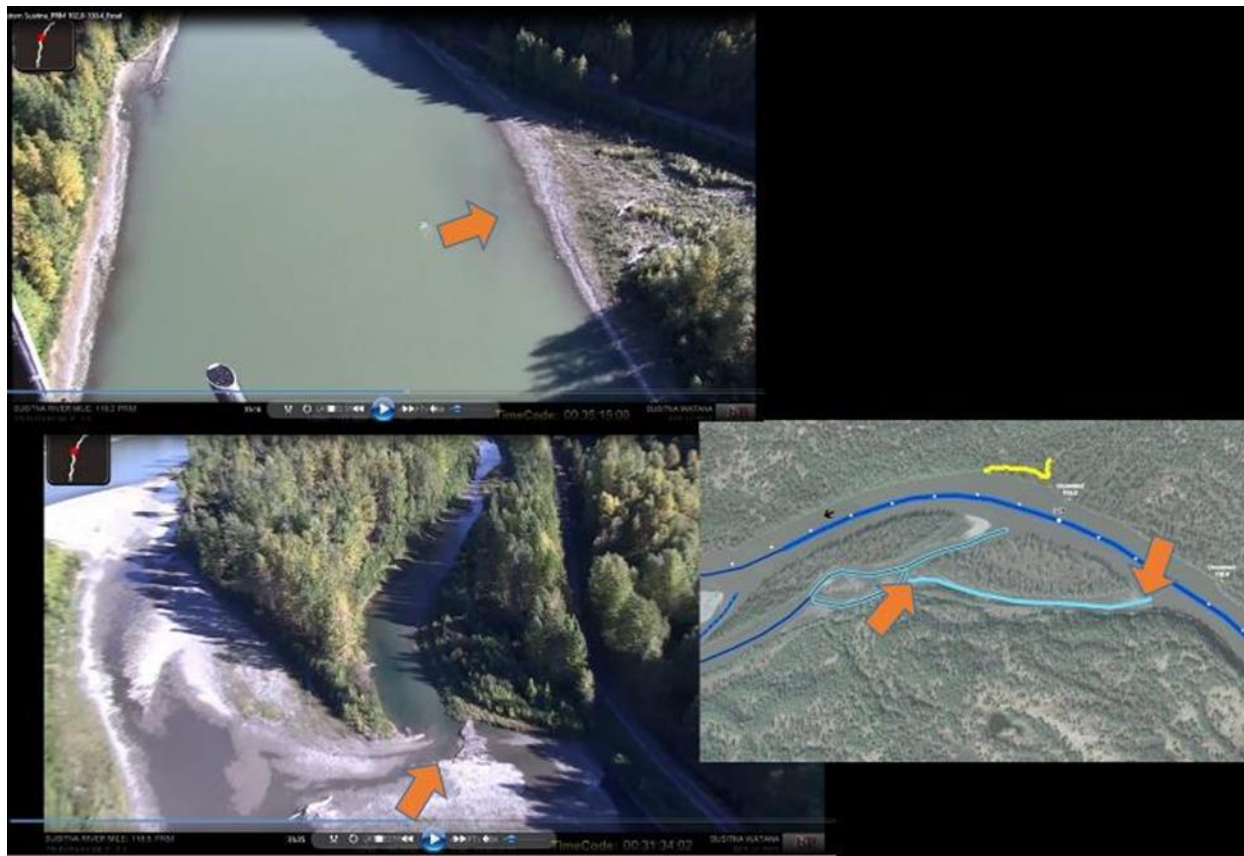
Figure 9. Two channels misclassified by AEA as side channels (inset). The right channel has clear water (bottom video capture) and upstream ends of both channels do not have an open water connection to the mainstem (top video capture). Based on AEA's classification methods both of these channels should be side sloughs. Side sloughs cannot change into split main channel as shown in inset.
