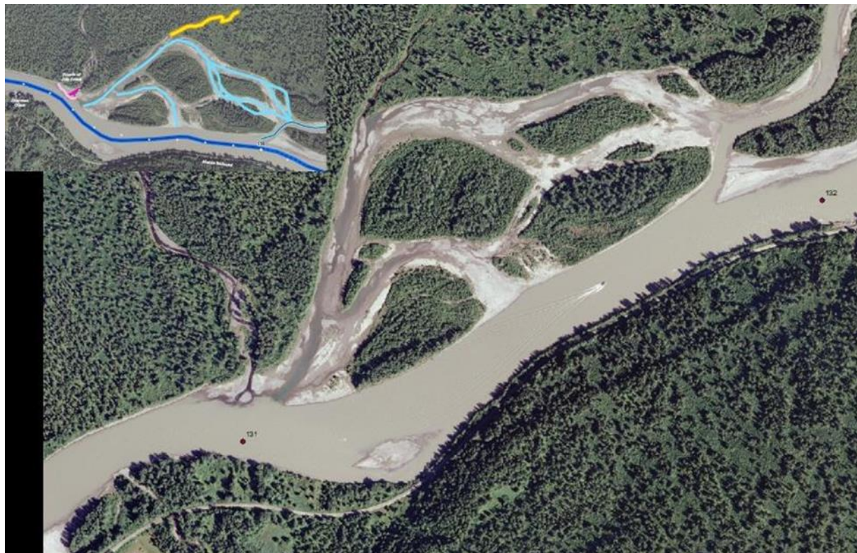
Figure 11. Differences in water turbidity and upstream connection to the main channel even under the higher flows in this aerial photograph shows that these side sloughs at PRM 131 were misclassified by AEA as side channels (inset).
