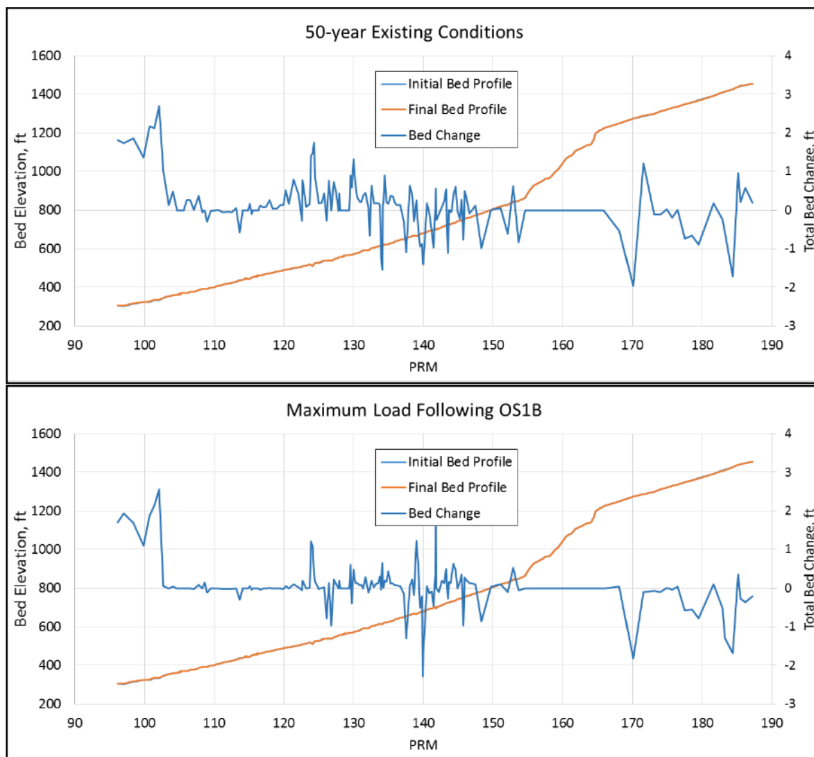
Figure 4. Bed changes along Middle Susitna River over a period of 50 years reported in Figure 5.1-9 of Fluvial Geomorphology Model Development - Technical Memorandum (Nov. 2015).
