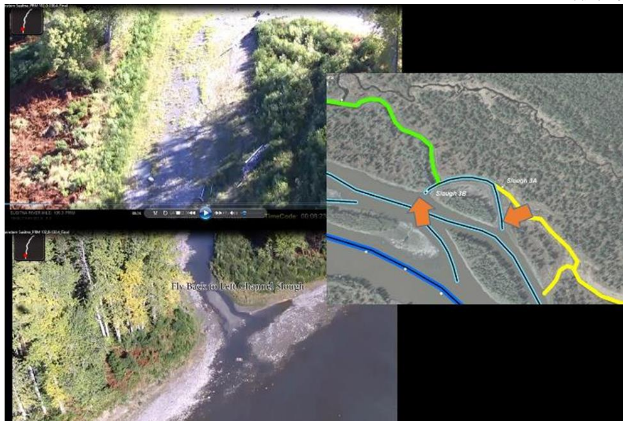
Figure 7. Upstream (top) (location shown with arrow on inset) and downstream (bottom) ends of channel within FA 104 from AEA 2012 video. Habitat was originally misclassified by AEA as side channel. The upstream end of the channel is partially vegetated and not connected to the mainstem and therefore, per AEA classification methods, the channel should be classified as a side slough. This channel was reclassified as side slough in AEA's latest classification maps.
