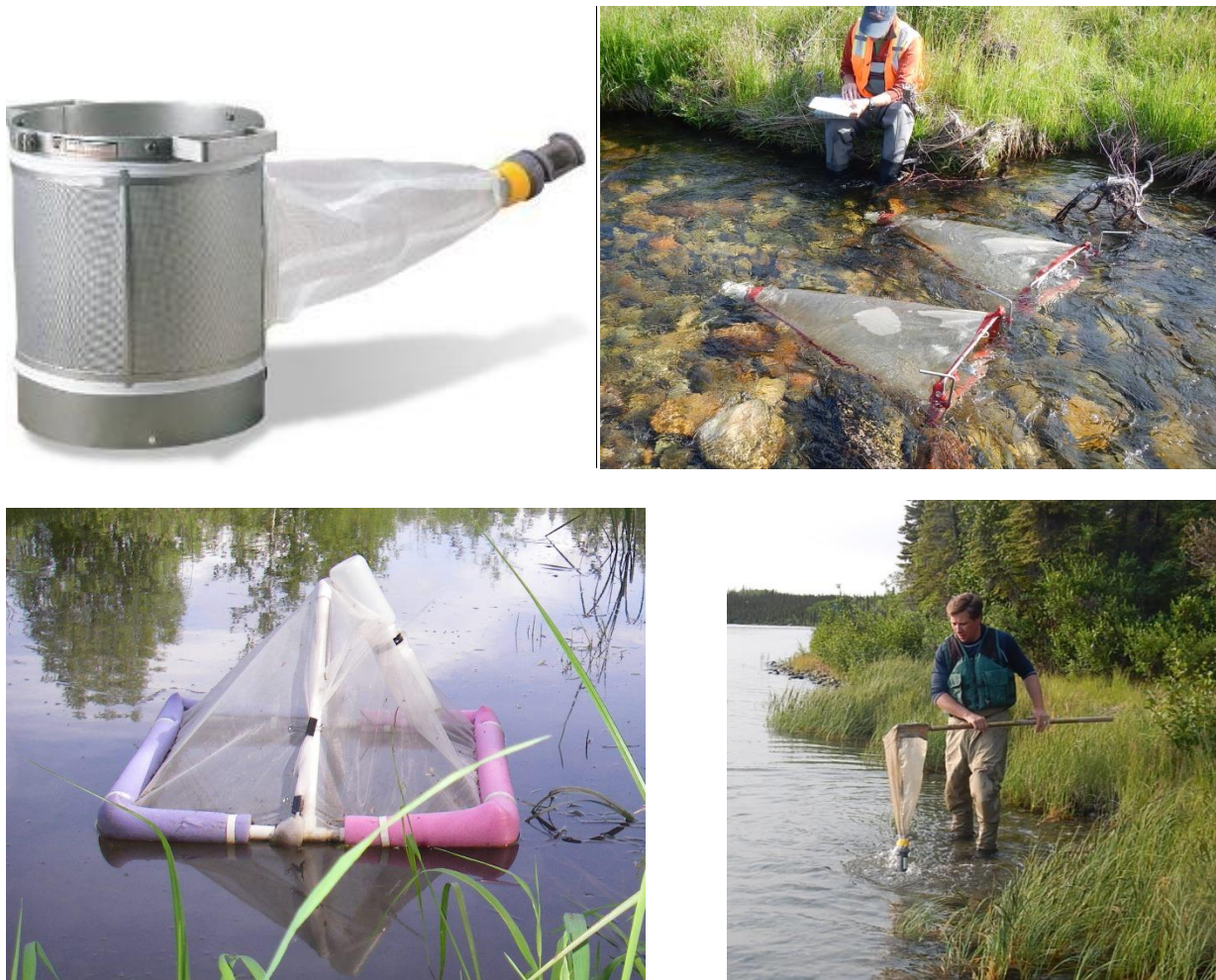
Figure 4.6-1. Sampling equipment used to collect benthic macroinvertebrates in streams and rivers Top left: Hess stream sampler. Top right: drift nets. Bottom left: floating aquatic insect emergence trap. Bottom right: D-net kick sampler.
