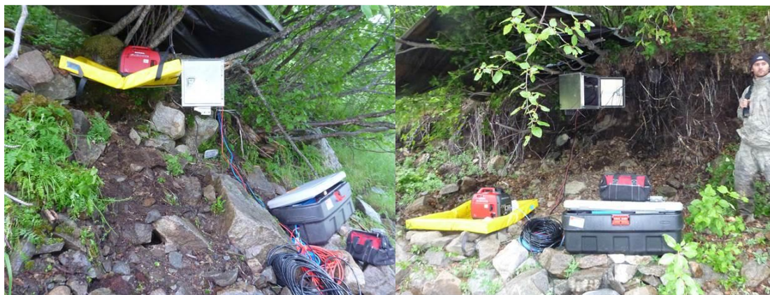
Figure G-3. Photographs showing the environmental boxes used to house the ARIS systems electronic components, and power sources (battery banks are inside action packers) for the left bank (left) and right bank (right) monitoring stations.
