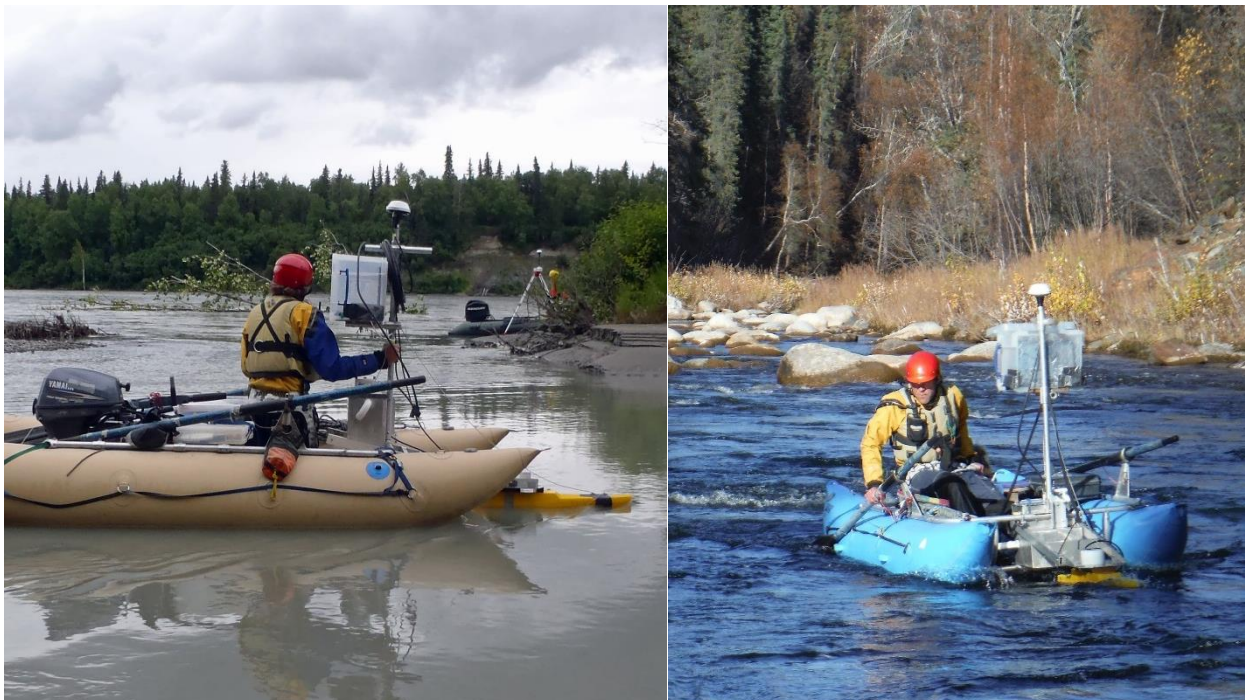
Figure 3. Techniques for maintaining a constant boat orientation.
