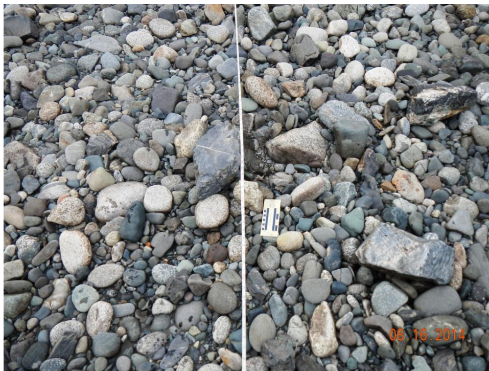
Figure A.2-91 – Surface material sediment sampling site at PRM 190.1. Median particle diameter ( D_{50} ) is 56.7 mm (P484).
