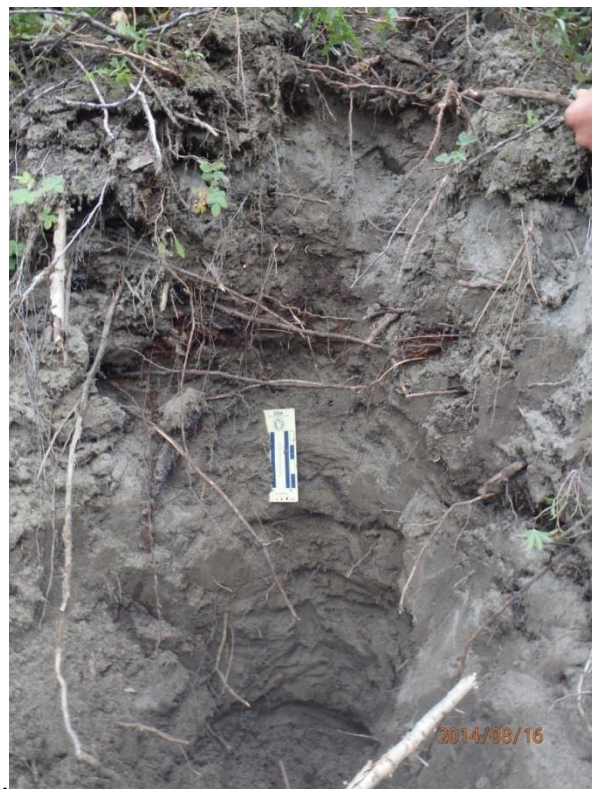
Figure A.2-87 – Bank stratification at PRM196.6. Note – This was the first observed occurrence of a relatively low floodplain in the Upper River Segment typical of those common in the Middle River Segment (approximately 6' from water surface on 8/16/14) (P432).
