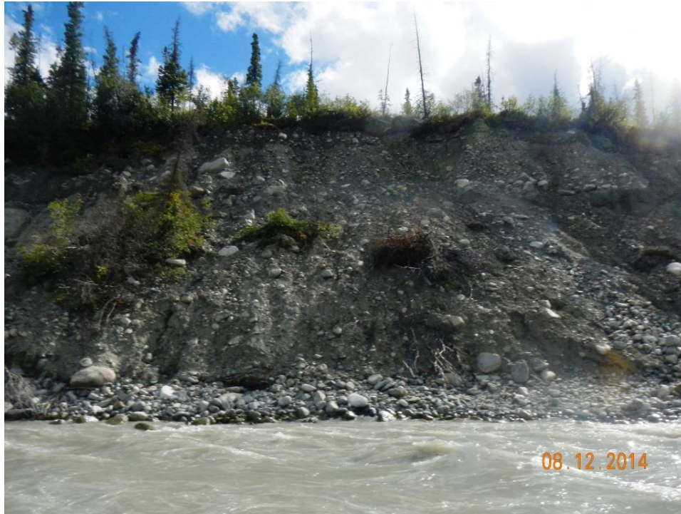
Figure A.2-37 - Course grained sediment (cobbles and boulders) source (till) near PRM 235.6 (P701).
