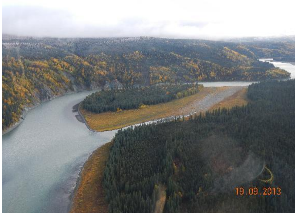
Figure A.2-65 – View upstream near PRM 208.5 of terrace height island and side channel. Lateral weir at head of channel and vegetating side channel bed. Active landslide zone and local sediment supply on outside bend (river right) (P5473).
