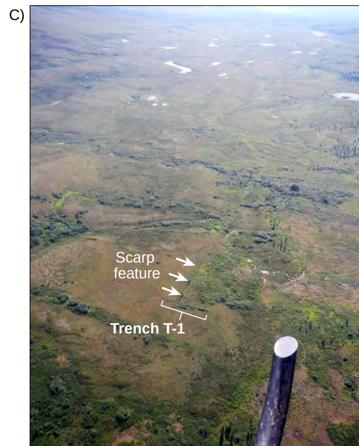
View of WCC T-1 looking southwest. Note how the expression of the scarp feature dies out along the projected trend of the feature.
