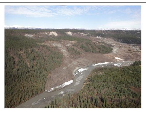
Figure 10. Translational Slide on SW-facing Slope along Watana Creek (Sheet 12-5).
