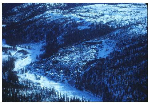
Figure 11. Translational Slide, Earth Block Slide of Frozen Ground, NE-facing Slope, Watana Creek (Sheet 12-6).
