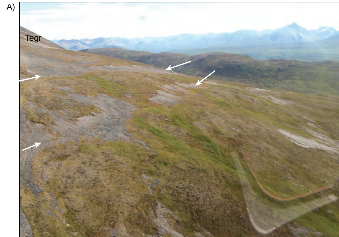
View looking east at likely solifluction-related scarps on hillside that correspond with mapped lineaments. Large arrows point along lineaments.
