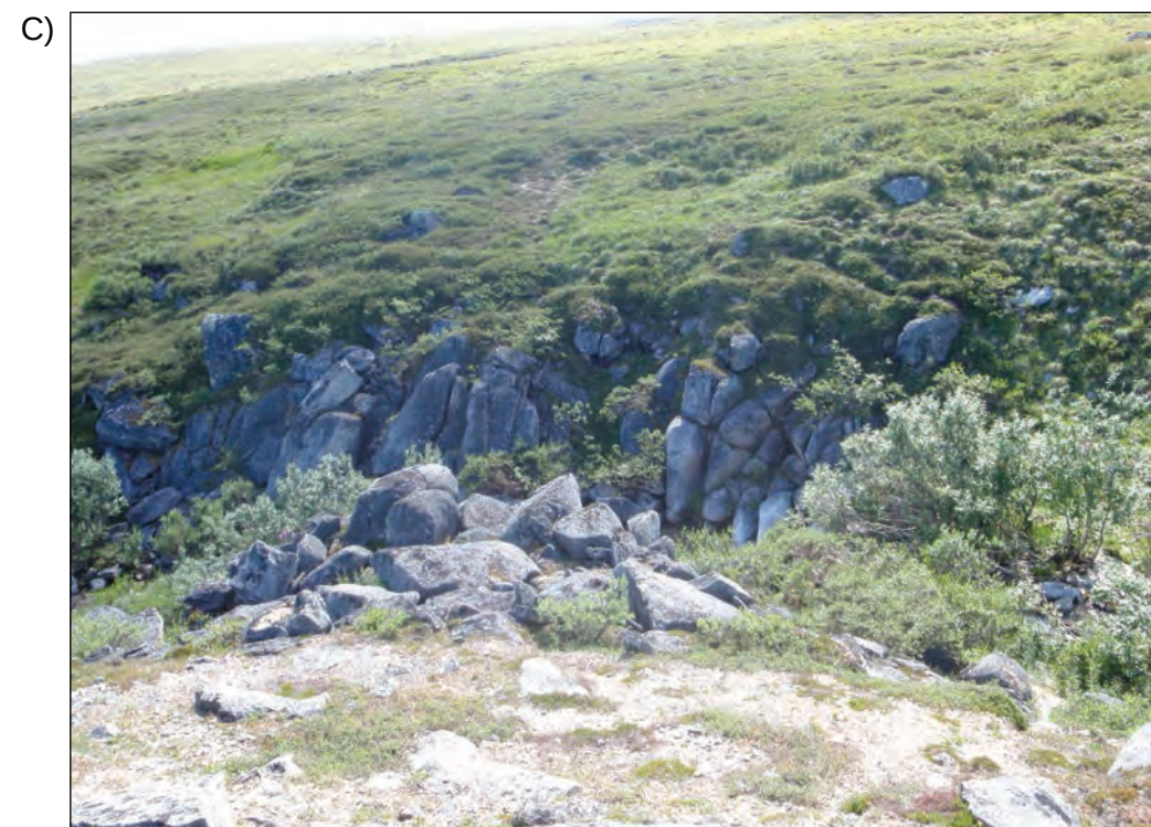
Photograph looking south-southwest from location C at widely spaced, near vertical, well-developed joints in trondhjemite (aka tonalite) bedrock. Joint spacing is 1 to 1.5 meters. Predominant orientations of joints are 042/80SE, 012/85SE, and 082/85SE but other orientations exist. Joint faces have clean surfaces with relief of minerals of 1 to 3 mm. No gouge or mineralization observed on joint surfaces, nor any sense of movement indicators (striae or mullions).
