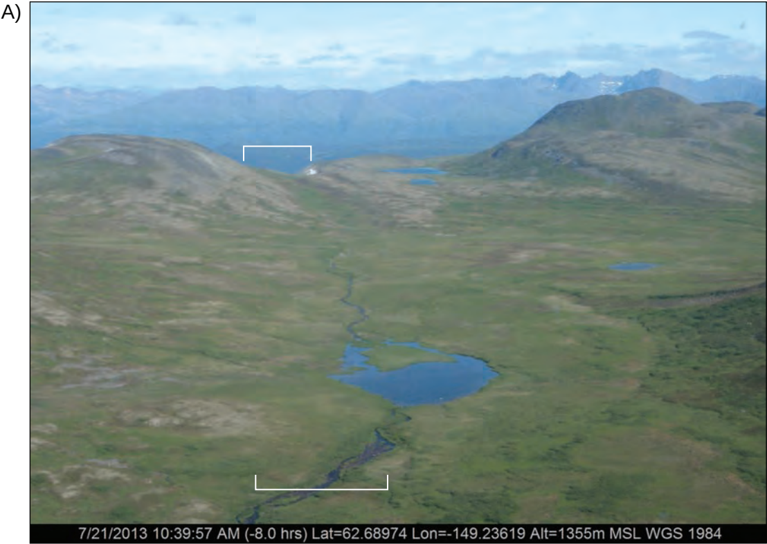
View looking north at middle portion of lineament group 8 along mapped inferred fault. Brackets show position of fault but note that no geomorphic expression of faulting is readily apparent.
