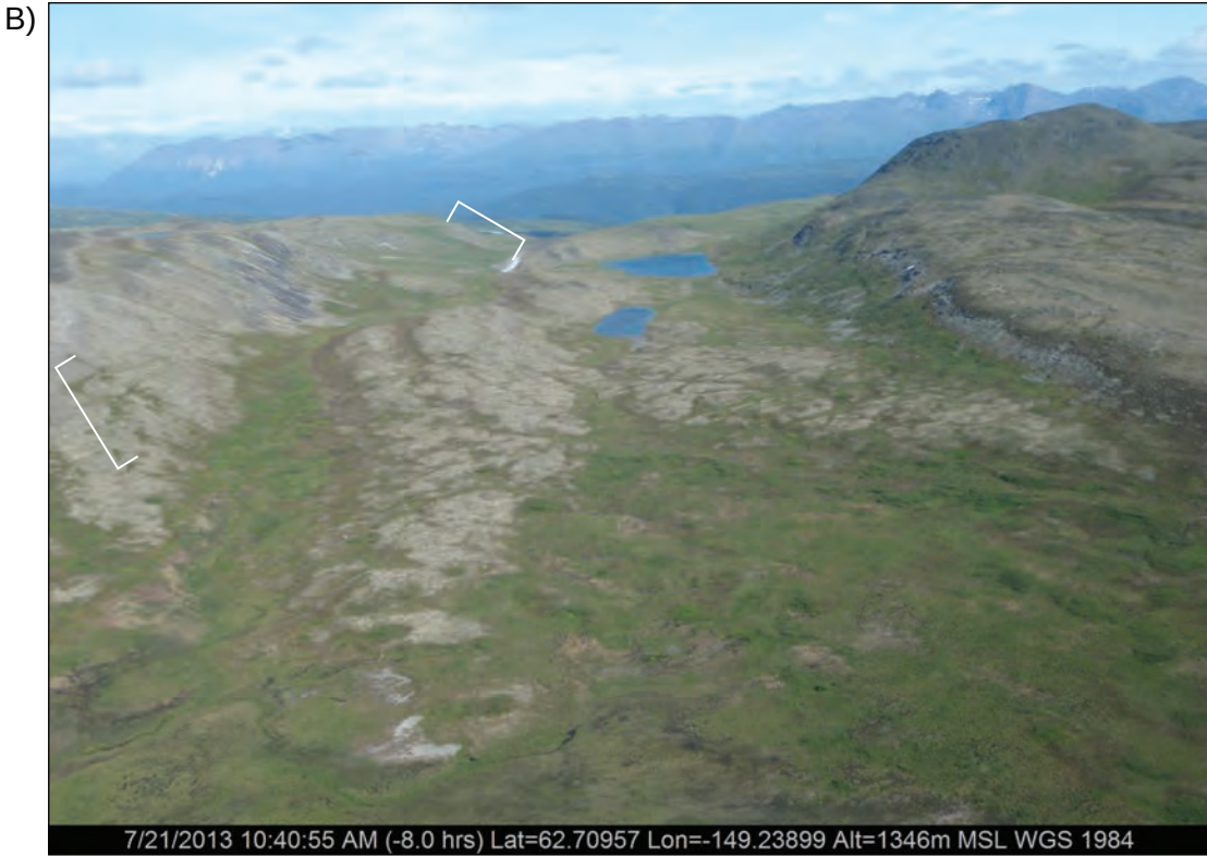
Close up view of saddle area shown in Photograph A. Brackets, again, show position of fault but note that no geomorphic expression of faulting is readily apparent.
