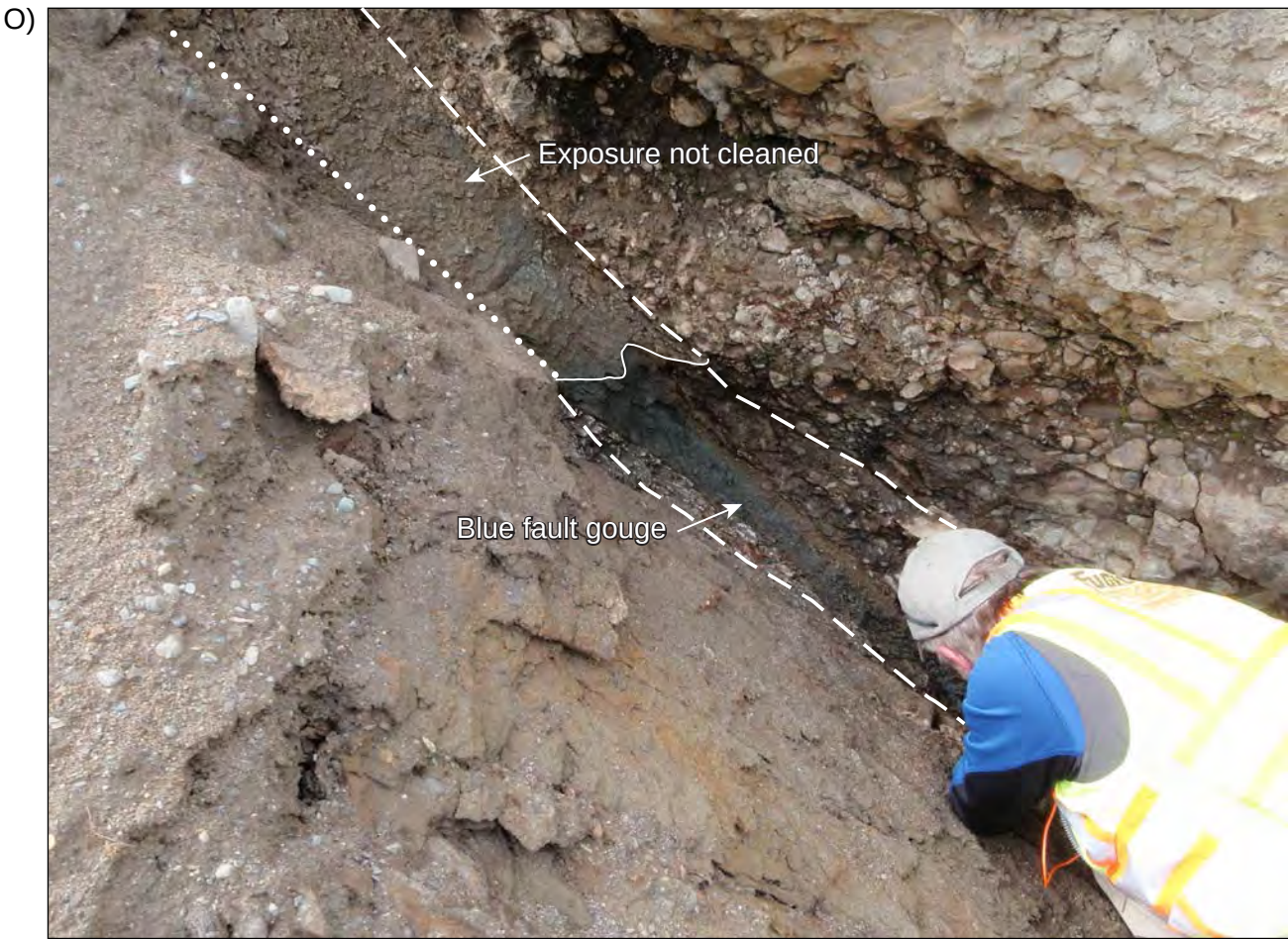
Close up of fault in cobble-rich Tertiary deposit.
