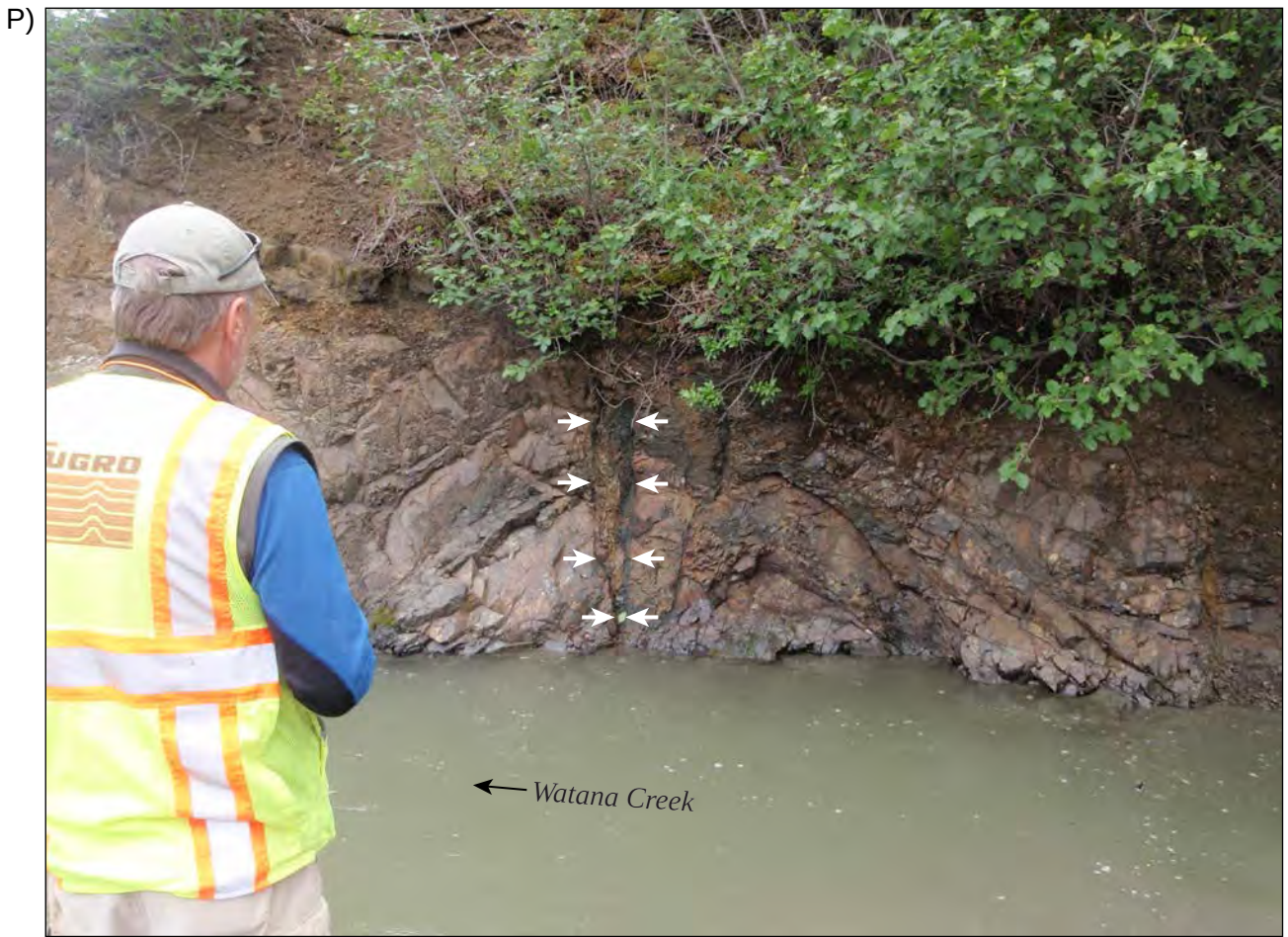
View looking south at vertical fault in Triassic rocks; visually estimated apparent strike is northeast.
