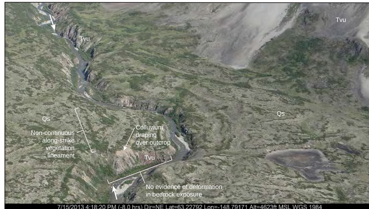
Photograph taken from location A looking east-northeast. Arrows show the alignment of FCL-mapped lineament. Note lack of apparent deformation in bedrock exposure along Jack River.
