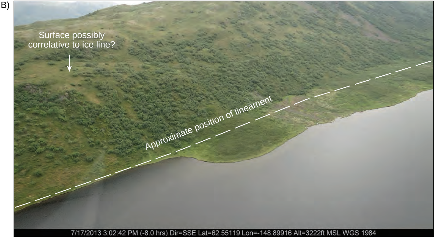
View looking south southwest at lake margin of glacial valley. Lineament was mapped at base of slope, and is not expressed as a scarp-type feature. Apparent colluvium along projection of lineament does not appear offset.
